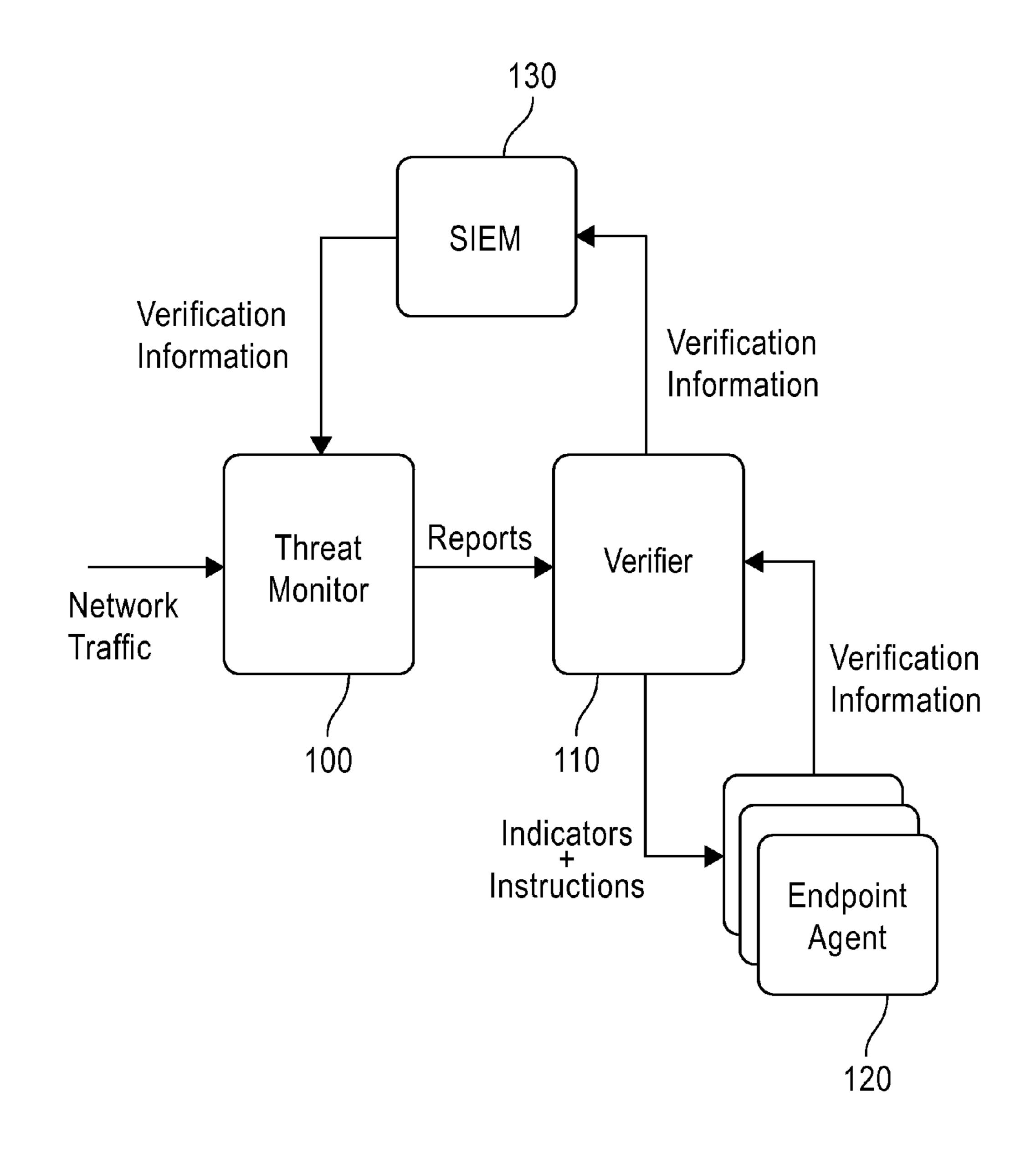
Fig. 1 SIEM Verification Verification Information Information Reports Threat Verifier Monitor Network Traffic Verification Information 100 110 Indicators Instructions Endpoint Agent
