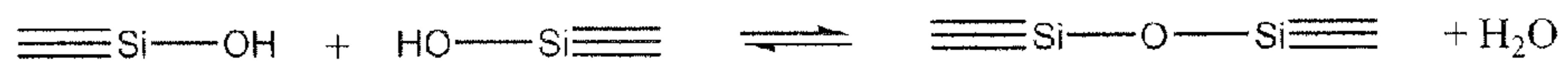
Figure 5. Condensation of hydrolyzed cyclohexyltrimethoxysilane with acid as a catalyst.
