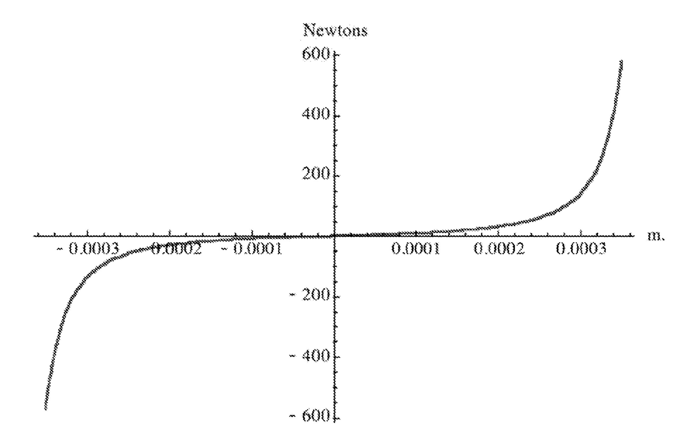
Stiffness at equilibrium position =  $\pm 176$  N/mm. Inductor losses at equilibrium = 97 Watts = 2.3% per 24 hours
