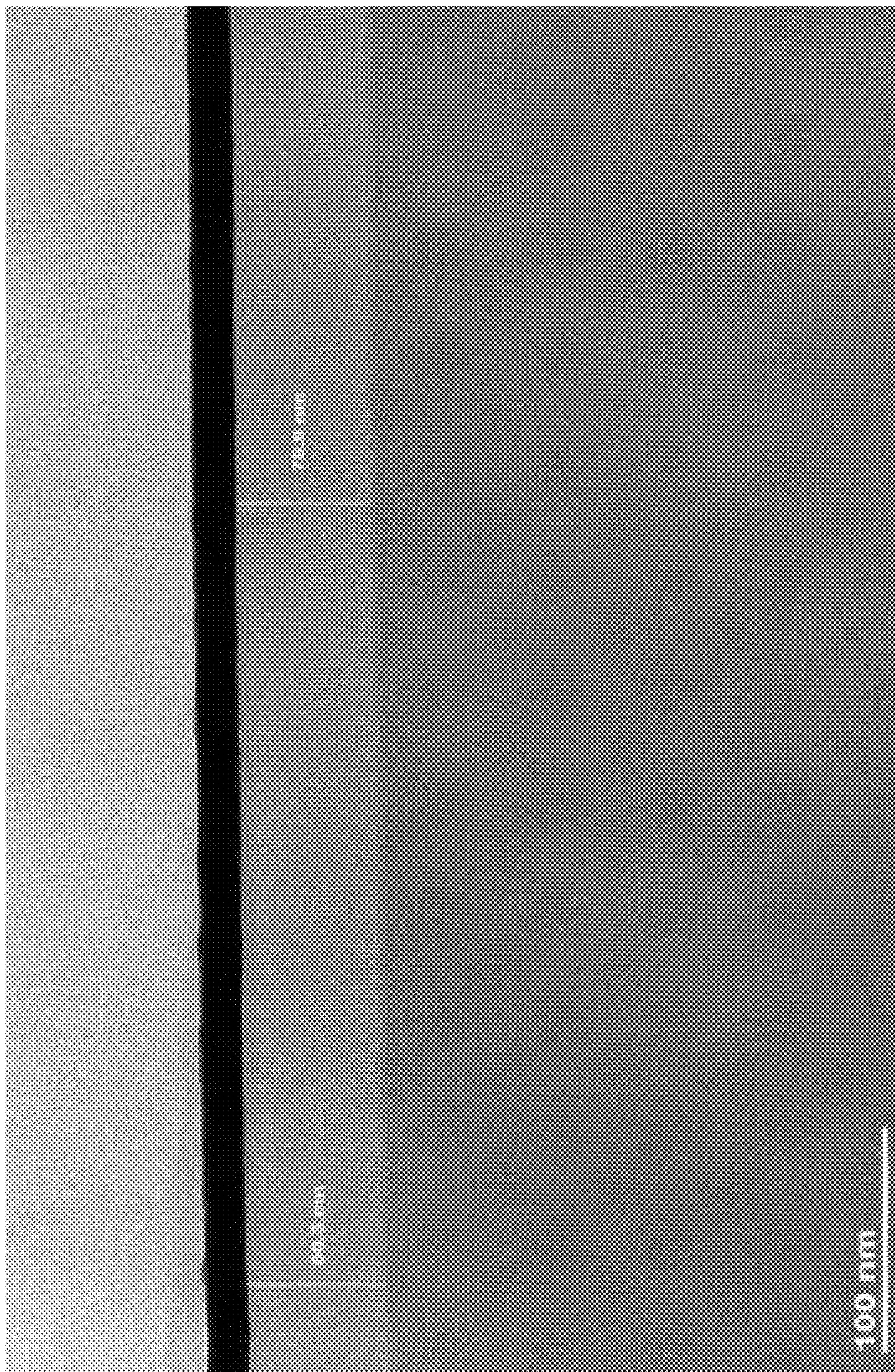
Figure 3A, Cross-sectional view of coating made from composition in Example 2
