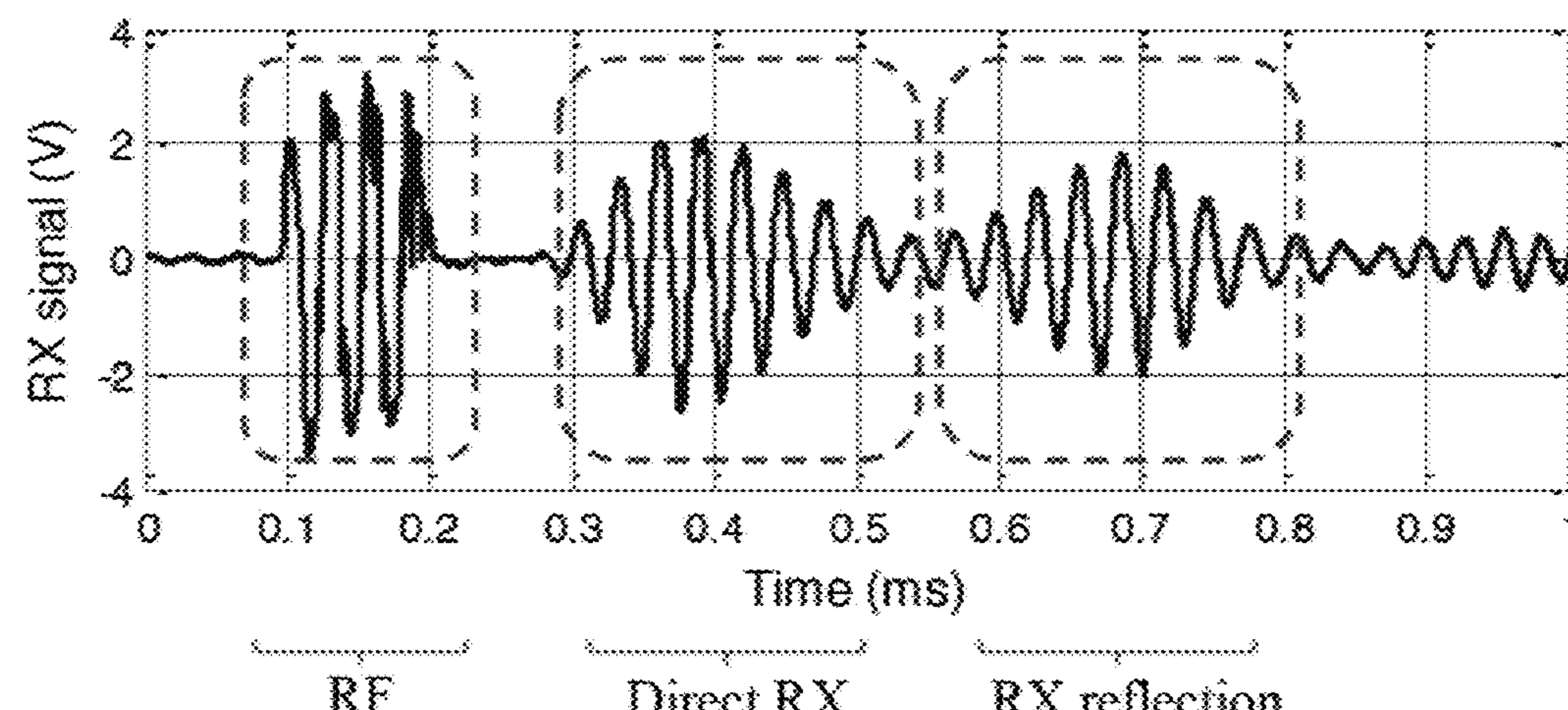
RF feedthrough      Direct RX signal      RX reflection from chamber wall
