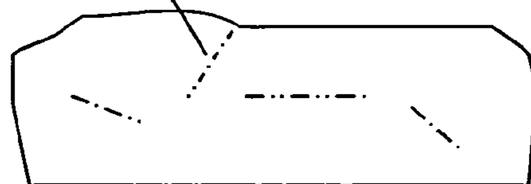
Graphene poly-crystal with incomplete grain boundaries (essentially a graphene single crystal with defects)
