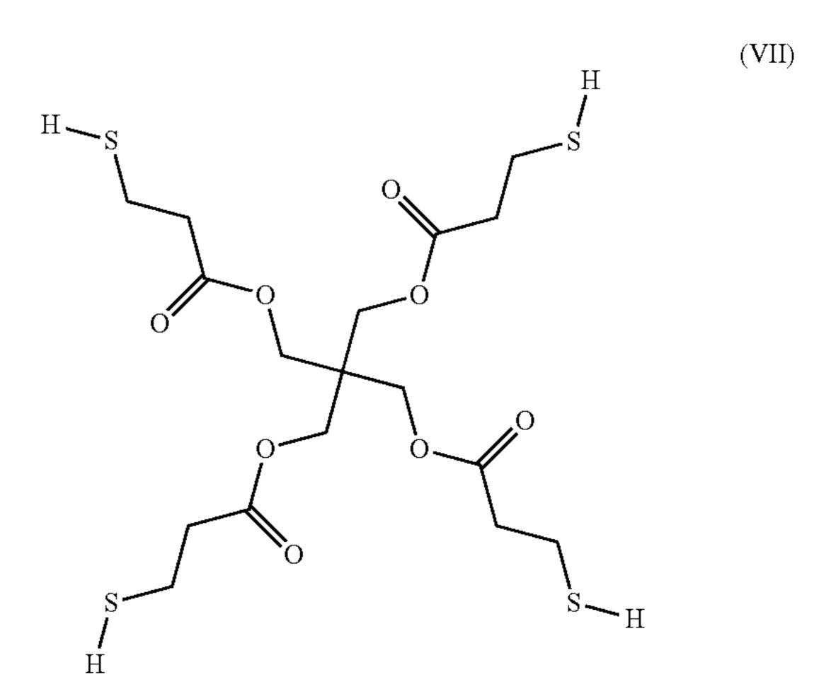
[0049] This tetrathiol preferably is reacted with triallyl isocyanurate as the polyfunctional allyl monomer. The weight ratio of the polyfunctional thiol to the polyfunctional allyl monomer is preferably comprised in the range from 55/45 to 57/43.
