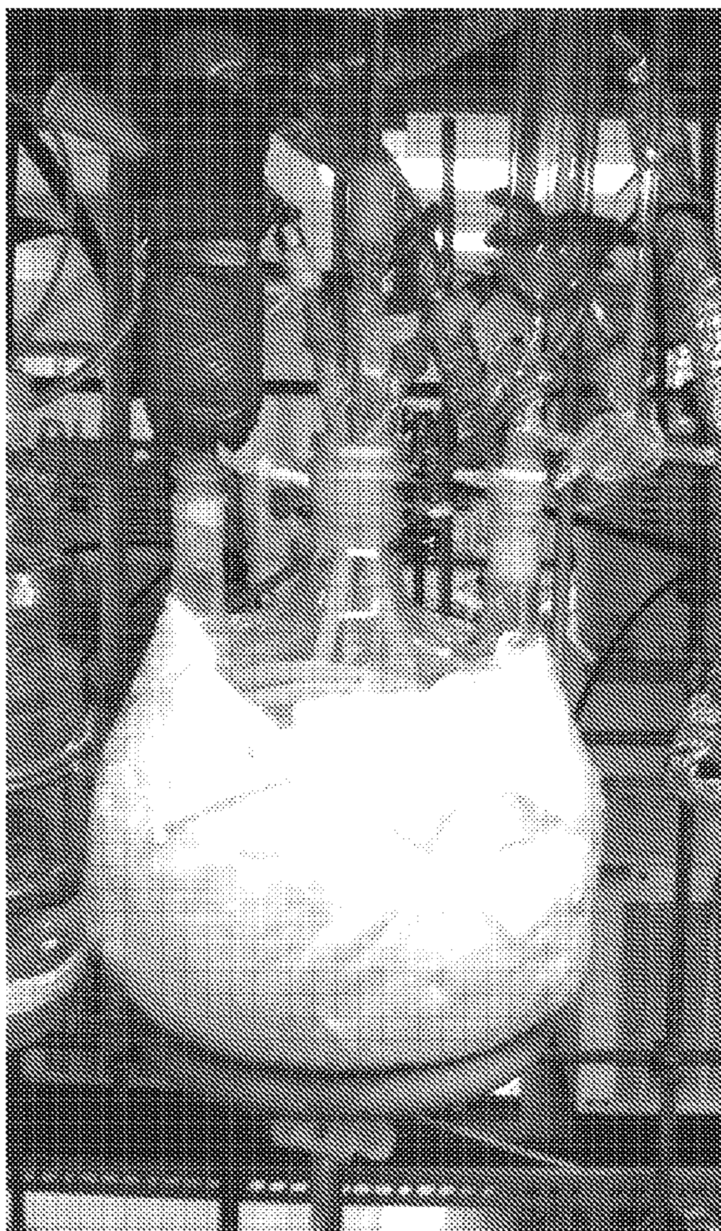
APPARATUS 1 - Apparatus for Hydroxypropylation of 1.3 kg of lignin comprised of a 12 L round-bottomed flask with bottom stopcock, internal cooling coils, reflux condenser, water-jacketed addition funnel, and overhead stirrer.
