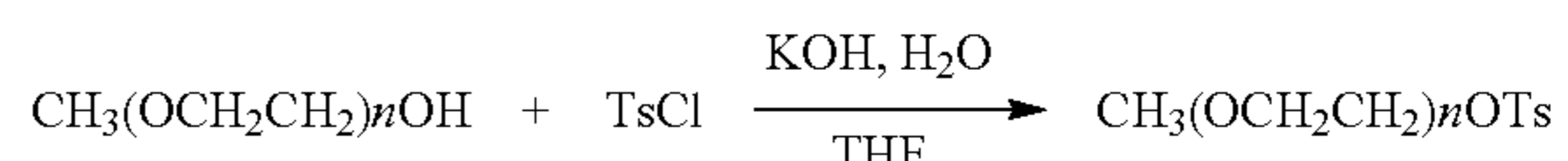
Scheme 2. Generic structure of monomer synthesis
