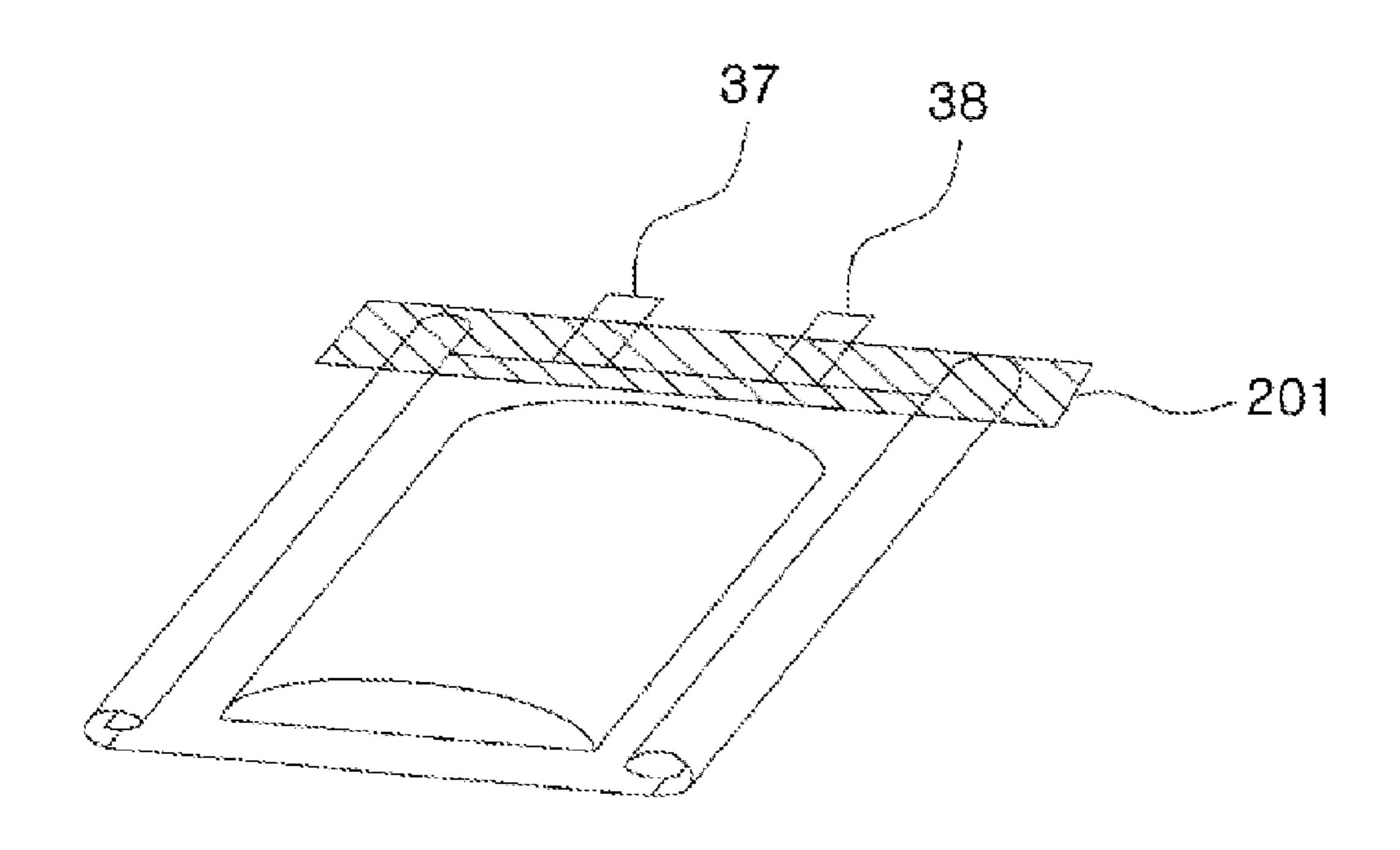
POUCH-TYPE BATTERY WITH IMPROVED SAFETY BY COATING SEALING UNIT WITH FLAME RETARDANT AND HEAT RESISTANT RESIN COMPOSITION PREPARED BY MIXING FLAME RETARDANT MATERIAL AND HEAT RESISTANT MATERIAL TO THERMOPLASTIC RESIN OR THERMOSETTING RESIN AND PRODUCTION METHOD THEREOF
