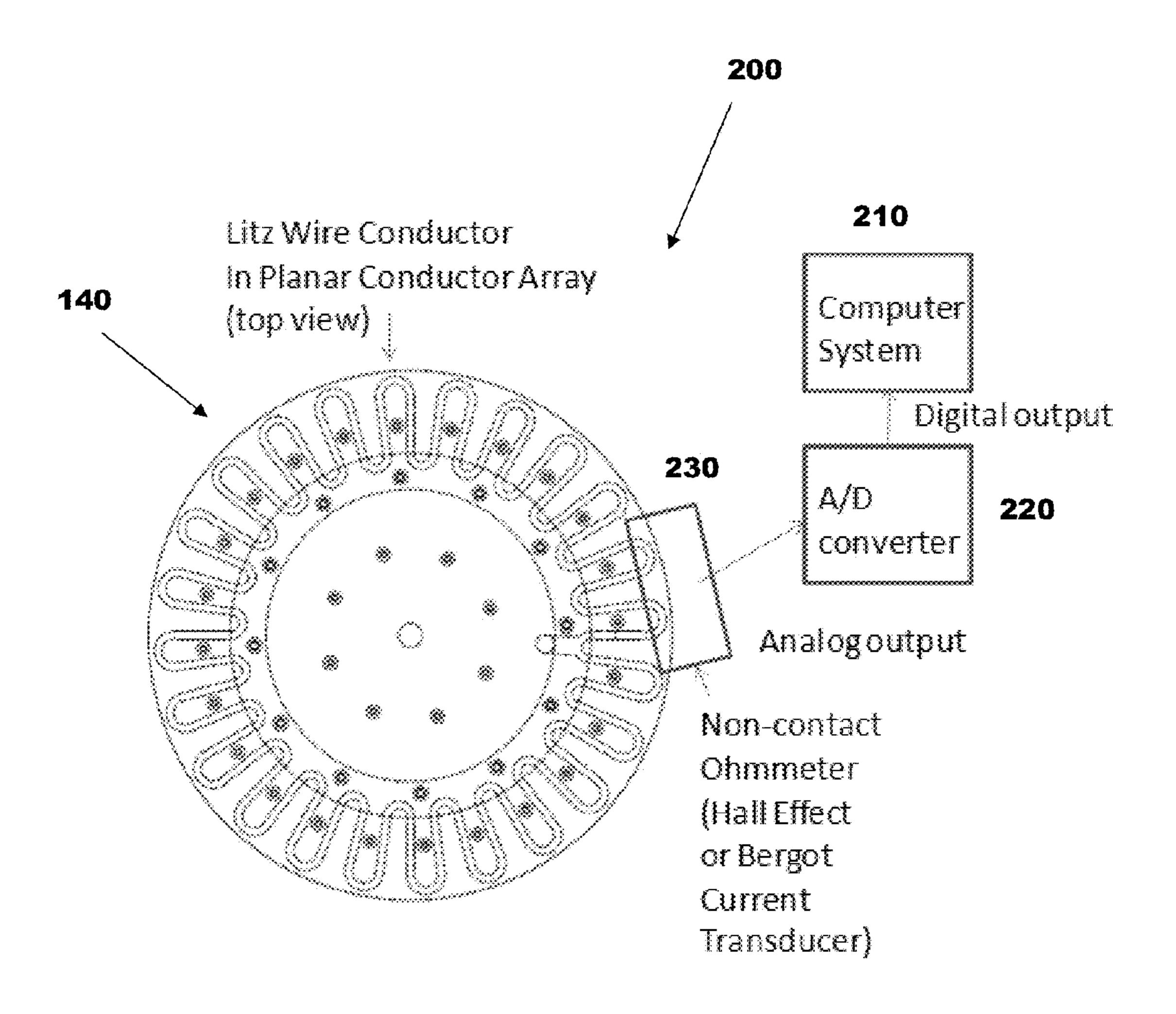
APPARATUS, SYSTEM AND METHOD FOR DETECTING ANOMALOUS AXIAL DISPLACEMENTS OF A MAGNETICALLY LEVITATED FLYWHEEL IN AN ELECTROMECHANICAL BATTERY SYSTEM AND RELATED SYSTEMS AND METHODS
