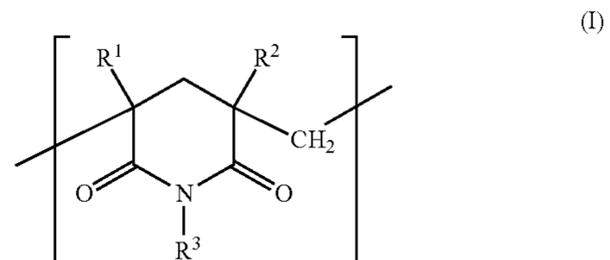
in which R<sup>1</sup> and R<sup>2</sup> are identical or different and denote hydrogen or a methyl group and R<sup>3</sup> denotes hydrogen or an alkyl or aryl radical having up to 20 carbon atoms.
