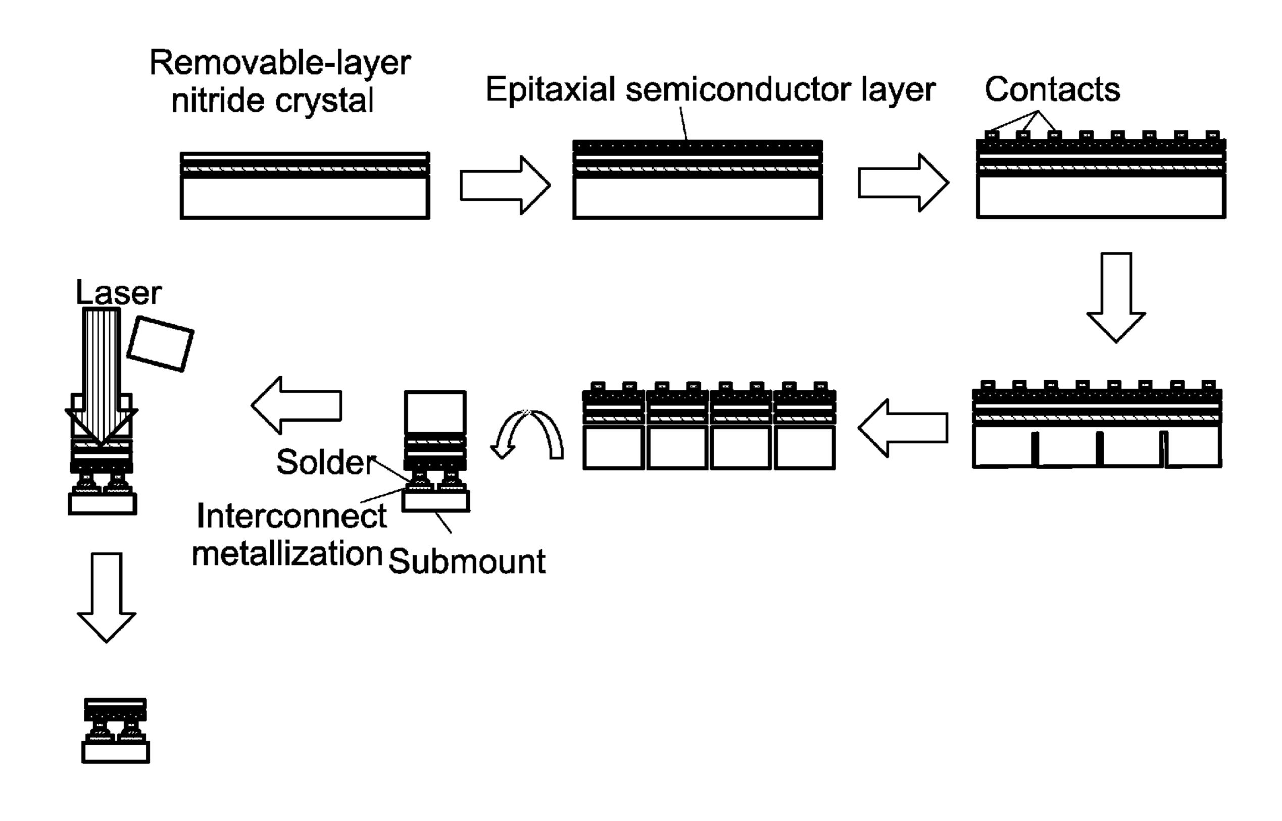
Fig. 1: Substrate fabrication
