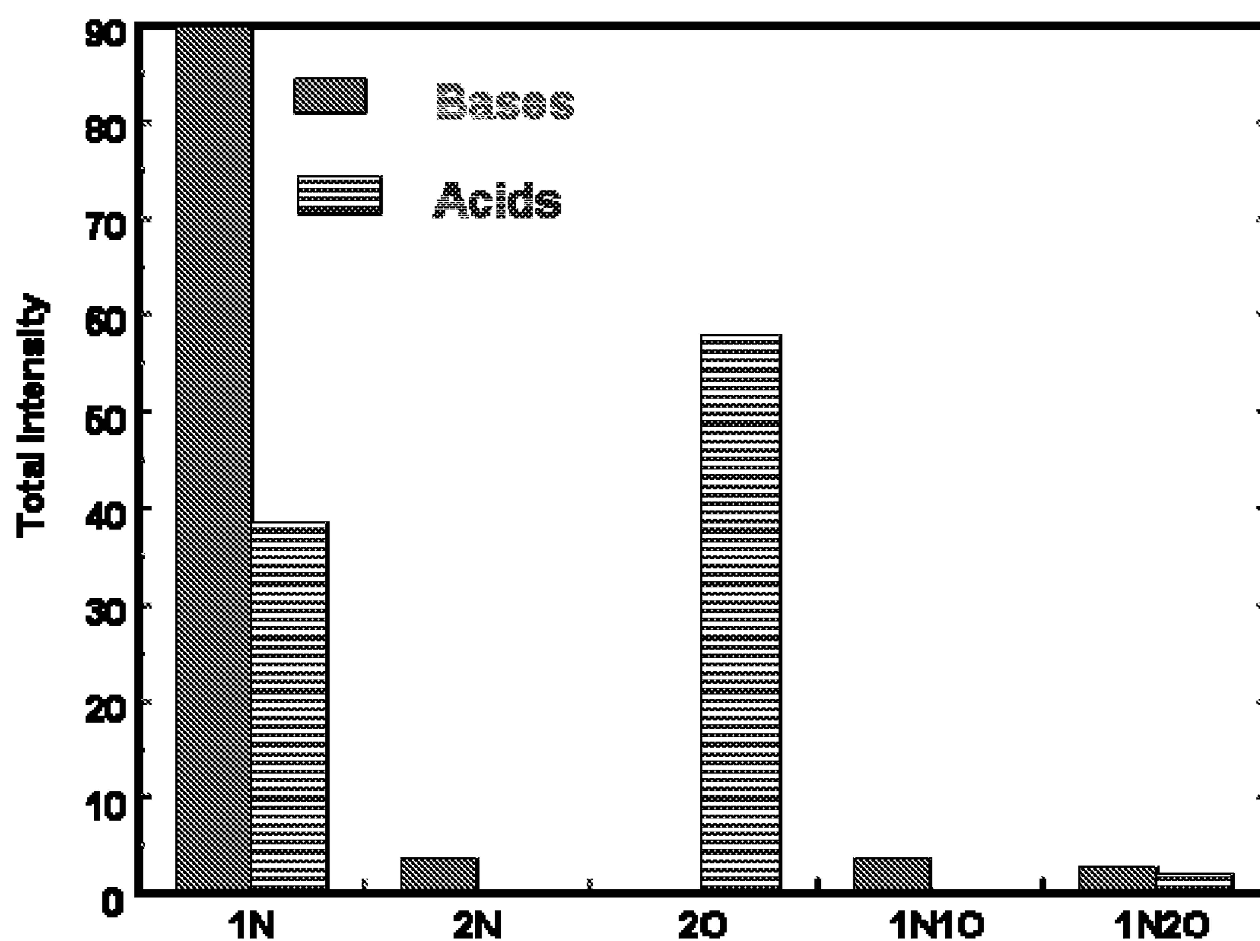
FIGURE 21 : Z-Number and Molecular Weight Distributions of Bases and Acids in DOBA VR
