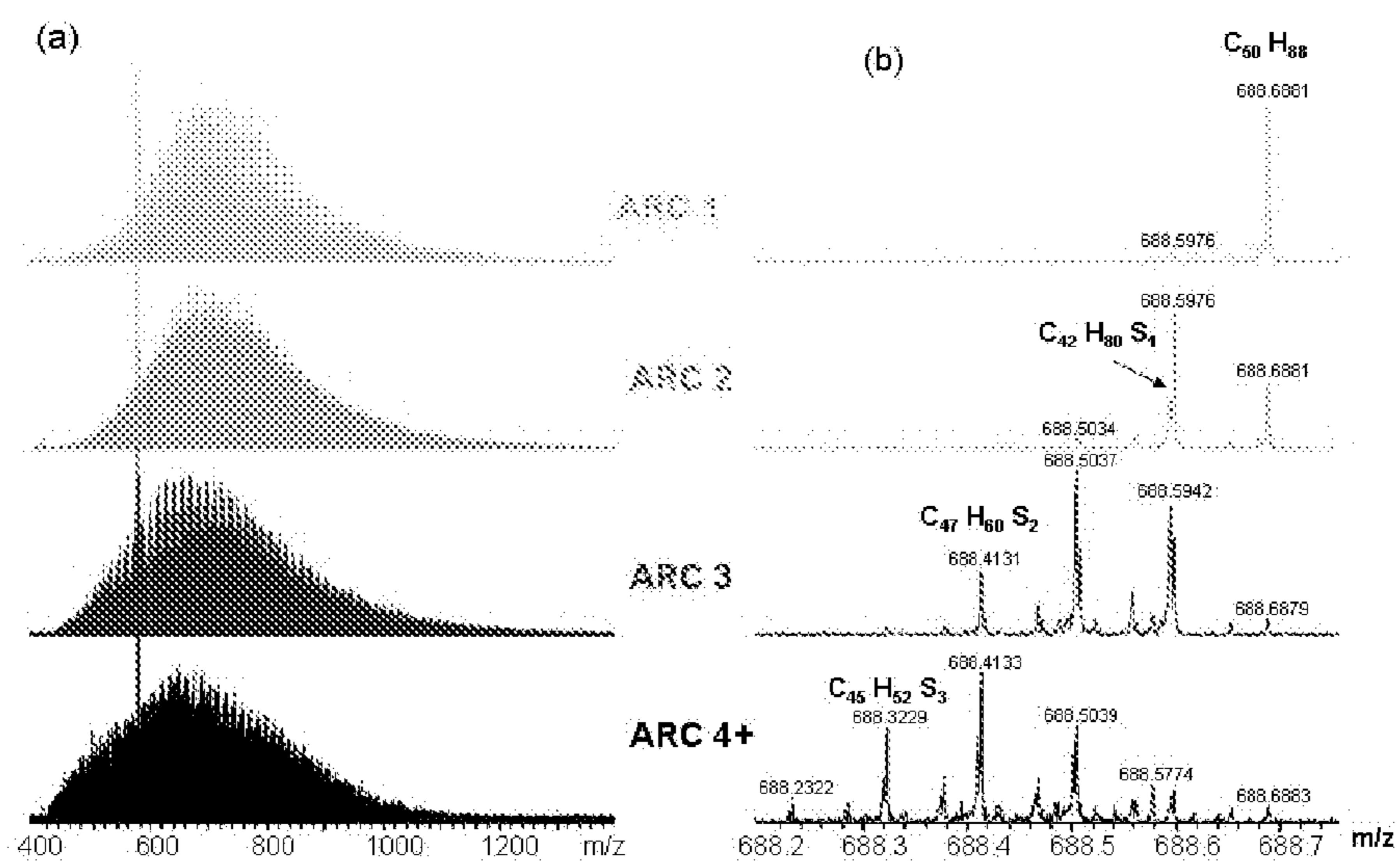
FIGURE 4 : The ionization of 1250F+ molecules asphaltenes and deasphalted oil (DAO) by laser desorption. Molecular weight species beyond 1500 g/mol are new species that cannot be volatized by APPI.
