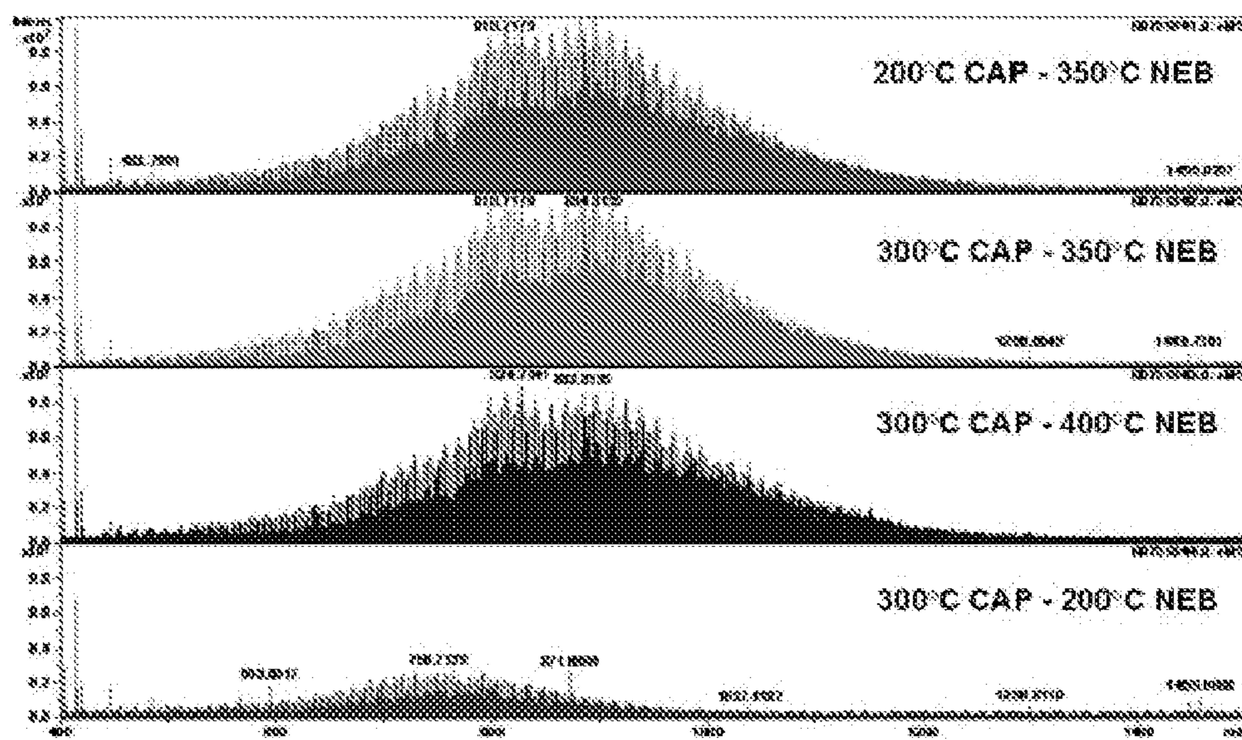
FIGURE 12 : APPI of Asphatene at 350F and 450F Nebulizer Temperatures
