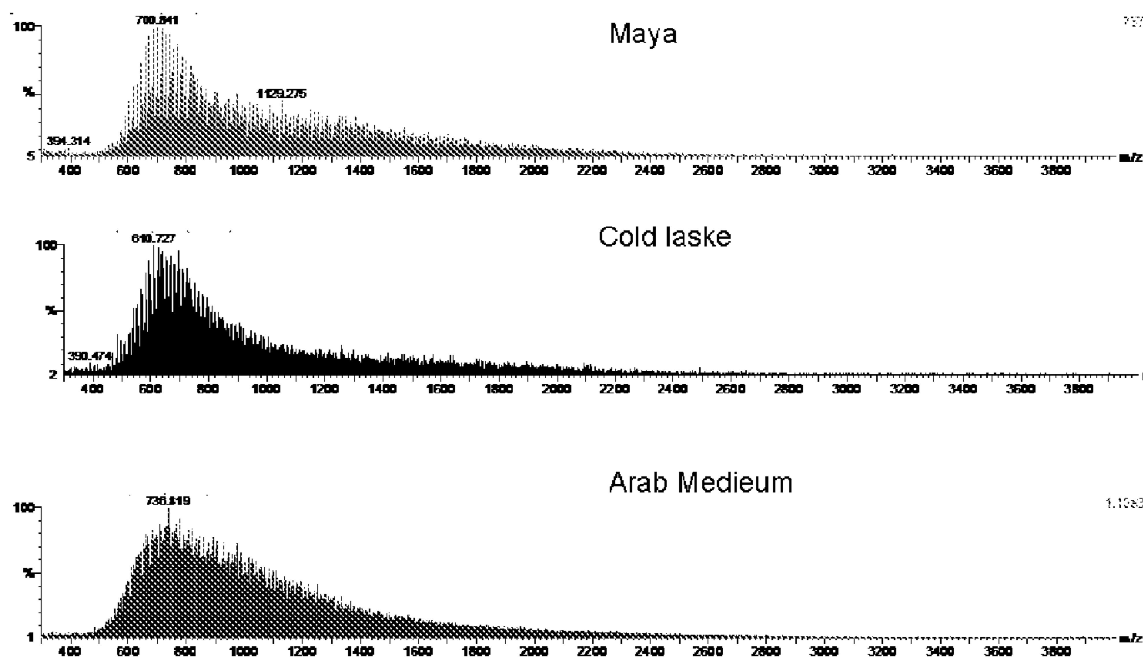
FIGURE 6 : The ultra-high mass resolving power by FTICR-MS needed to resolve petroleum molecules.
