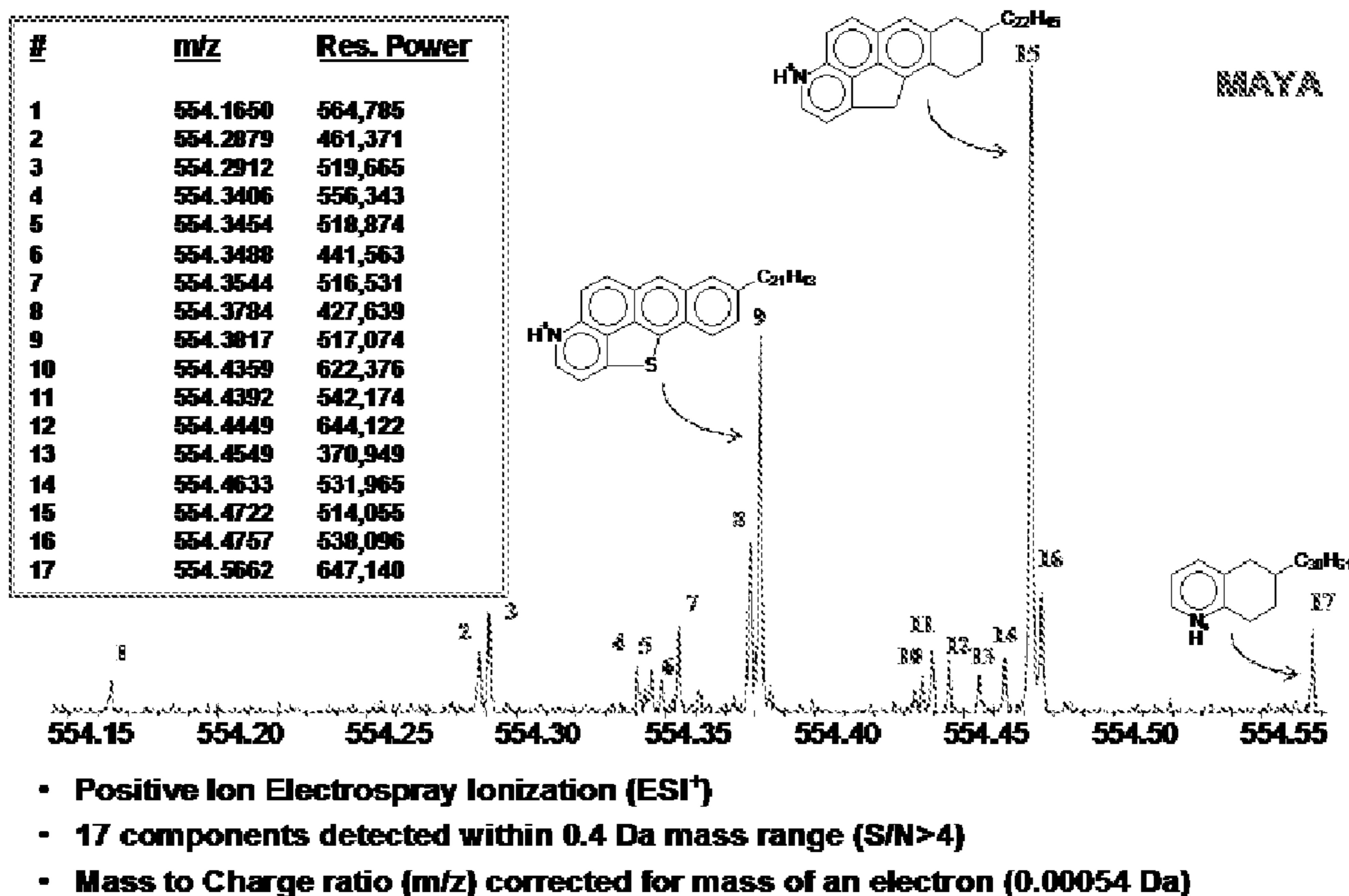
FIGURE 7 : The assignments of molecular formulas for an asphaltene sample.
