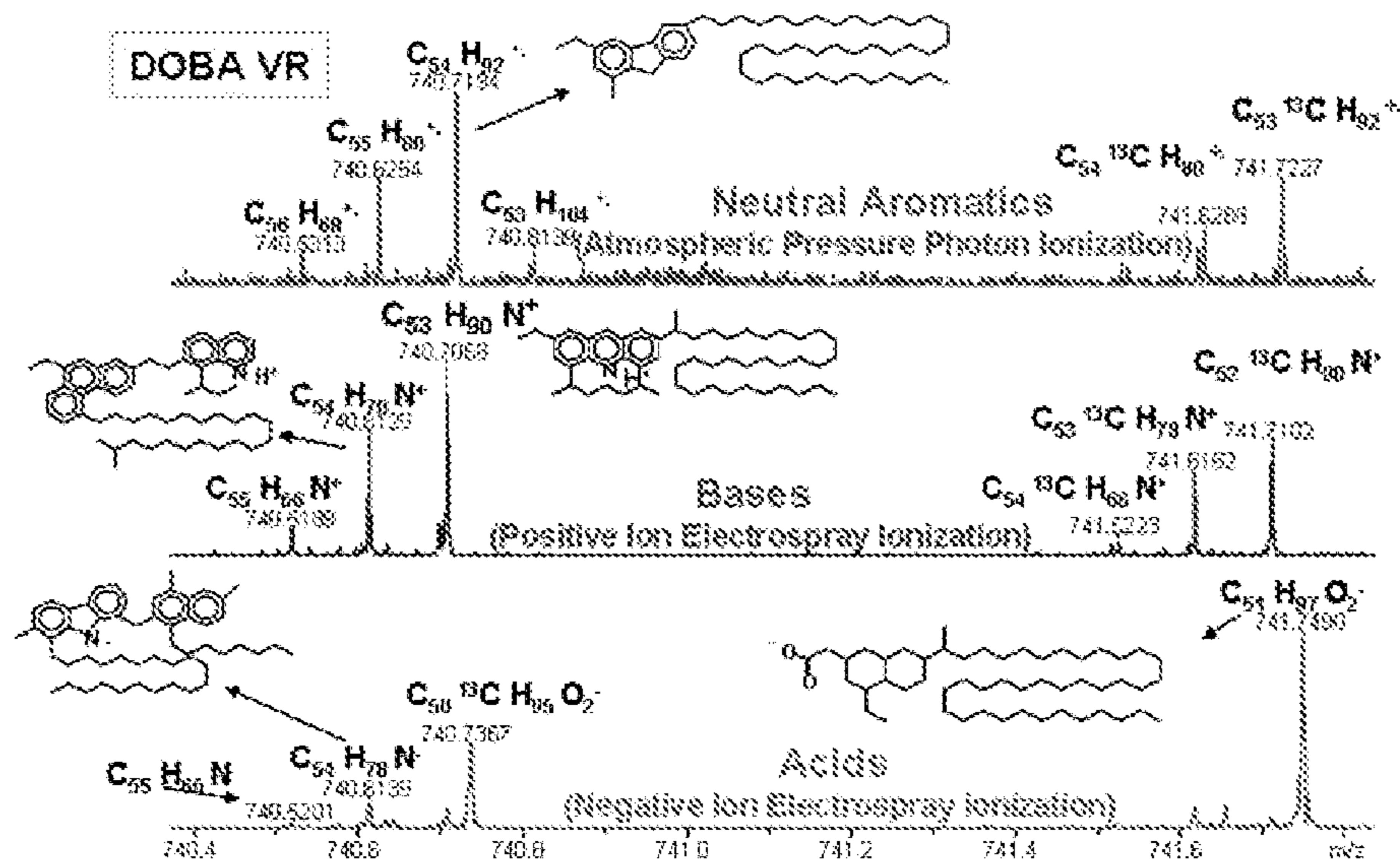
FIGURE 3 : The ionization of aromatic ring classes by Atmospheric Pressure Photoionization for Cold Lake VR ARC fractions (a) full range
