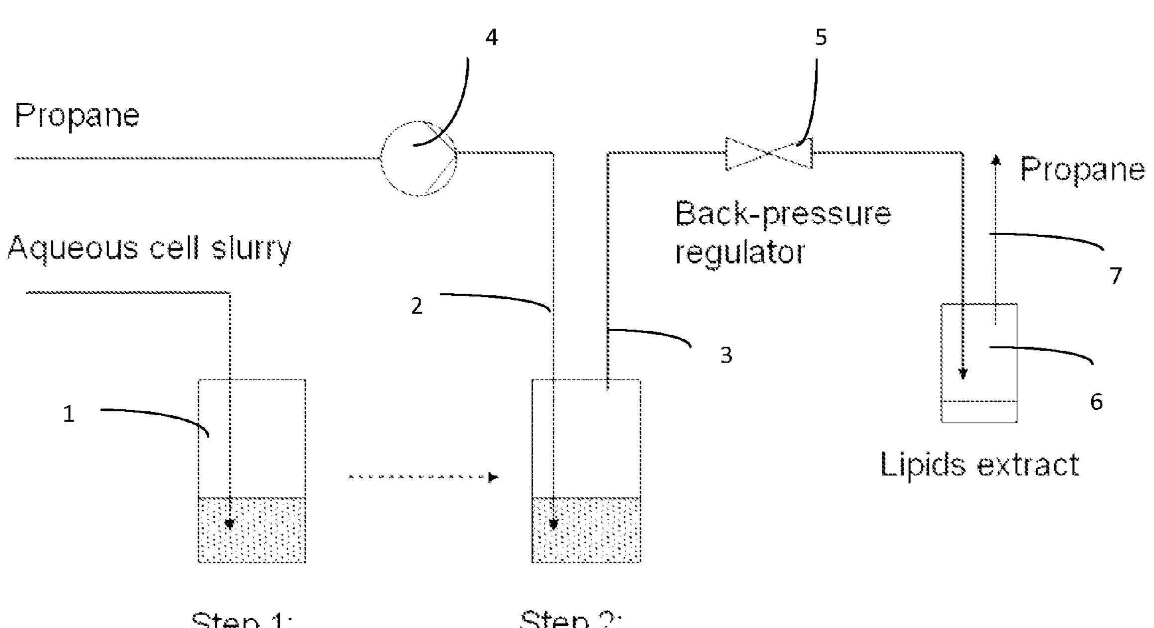
Step 1: Step 2: Heat treatment Lipids extraction with propane
