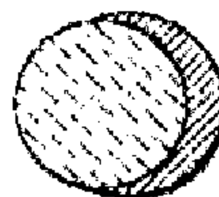
PA-CONTAINING NANO-PARTICLE COVERED WITH METAL NANOCAP
