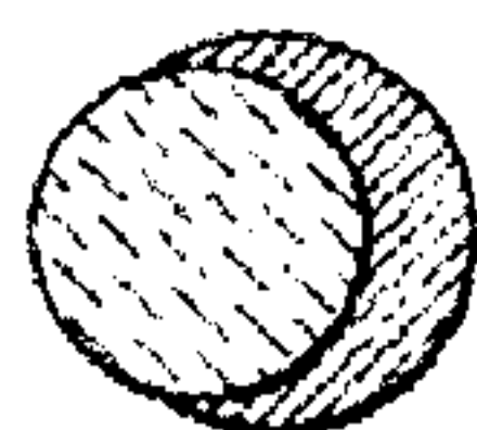
DIELECTRIC NANOPARTICLE CORE COVERED WITH METAL NANOCAP
