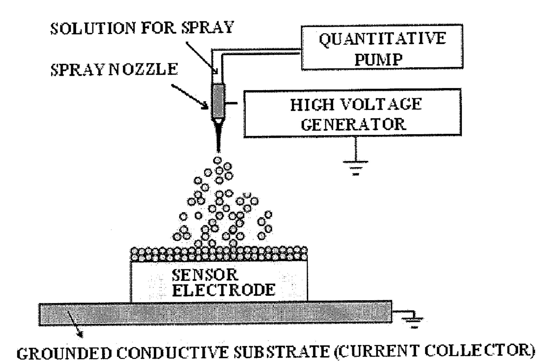
SOLUTION FOR SPRAY = METAL OXIDE NANOPARTICLES
