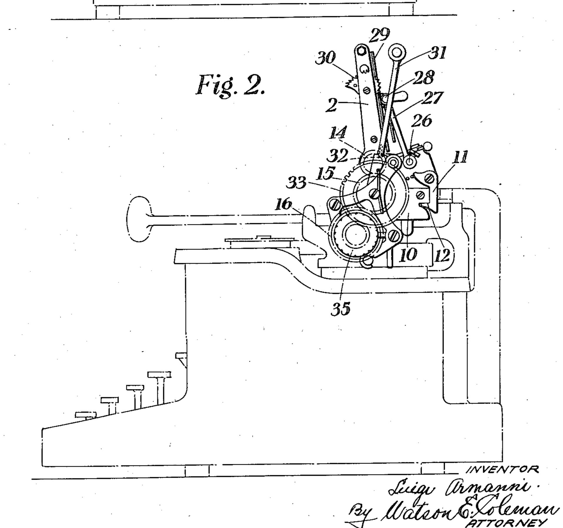
MEANS FOR FEEDING SHEETS OF PAPER, ENVELOPES AND THE LIKE TO TYPEWRITING MACHINES Filed May 6, 1933 2 Sheet
