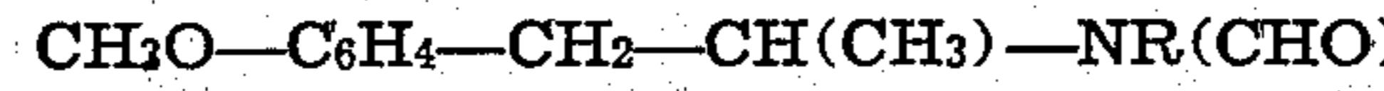
which comprises: reacting paramethoxybenzyl methyl ketone, a salt of an amine  $\text{RNH}_2$ , and a salt of formic acid, R designating hydrogen, an alkyl radical or an aralkyl radical.
