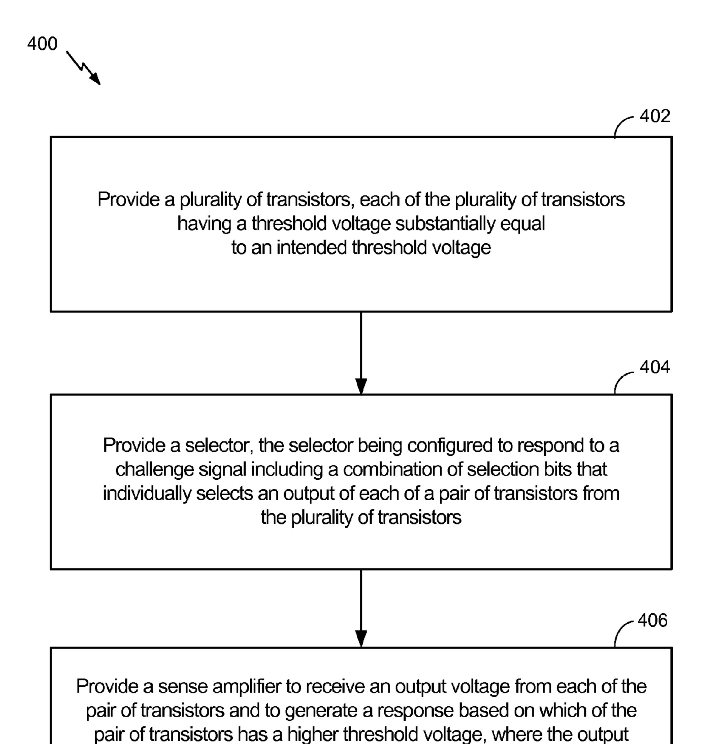
voltage of each of the pair of transistors varies as a result of a variation
