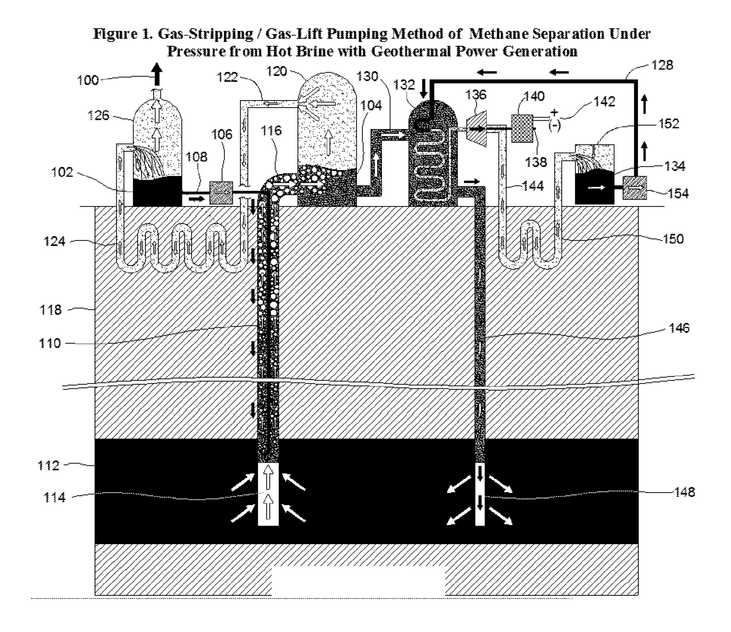
Figure 2. Gas-Stripping / Gas-Lift Pumping Method of Methane Separation Under Pressure from Hot Brine with Geothermal Power Generation and with Total Flow Concept Kinetic Energy Power Generation
