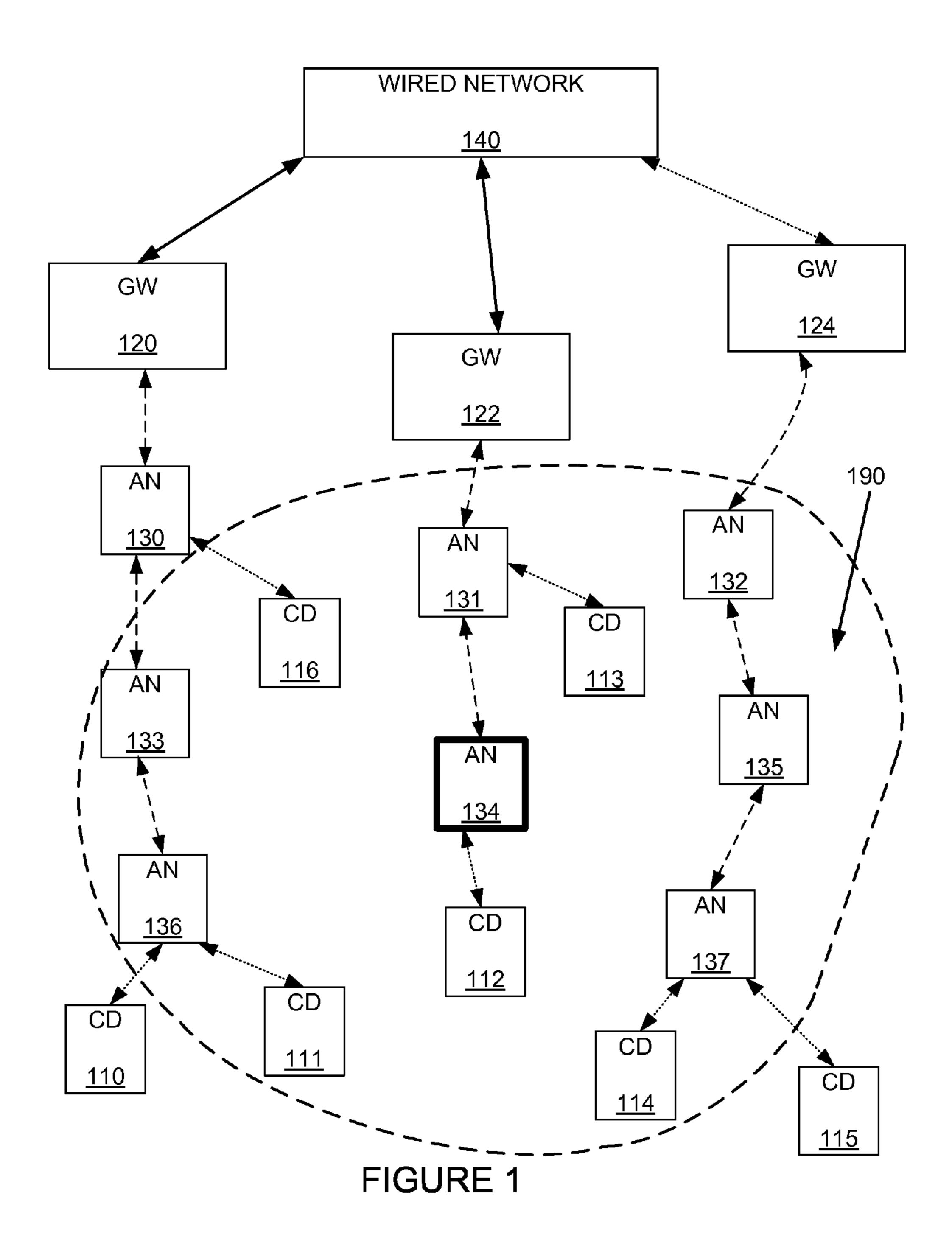
The wireless node monitoring air-time available to the wireless node for wireless transmission
