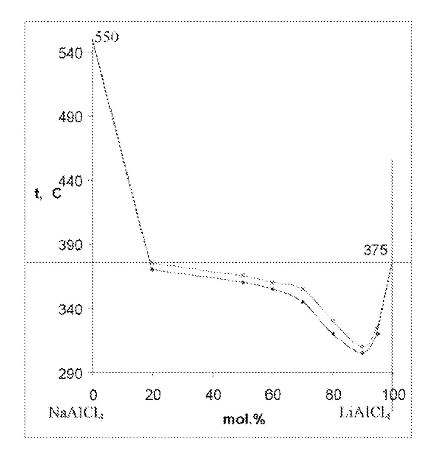
Fig. 1. Liquidus curve of the pseudo-binary LiAlCl<sub>4</sub>-NaAlCl<sub>4</sub> system containing additional 5 mol.% NaCl.
