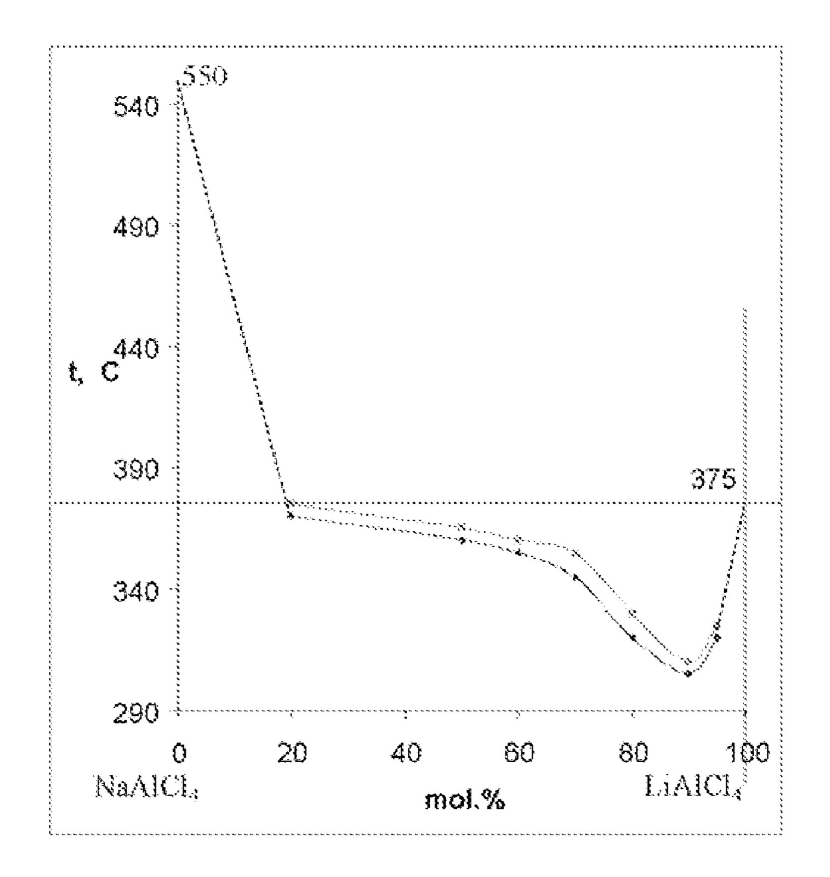
Liquidus curve of the pseudo-binary LiAlCl<sub>4</sub>-NaAlCl<sub>4</sub> system containing additional 5 mol.% NaCl.
