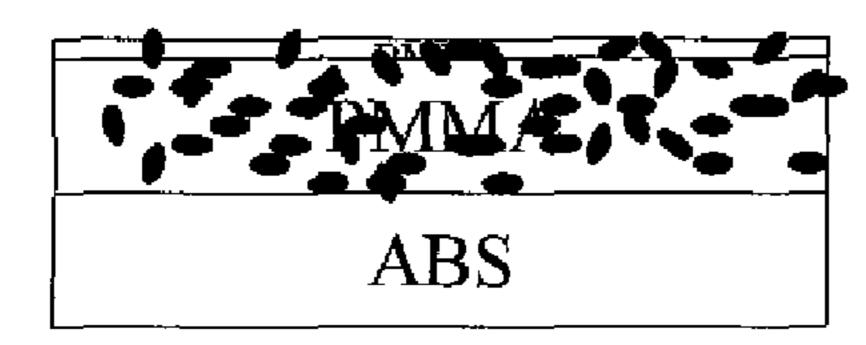
Produced by conventional coextrusion.
