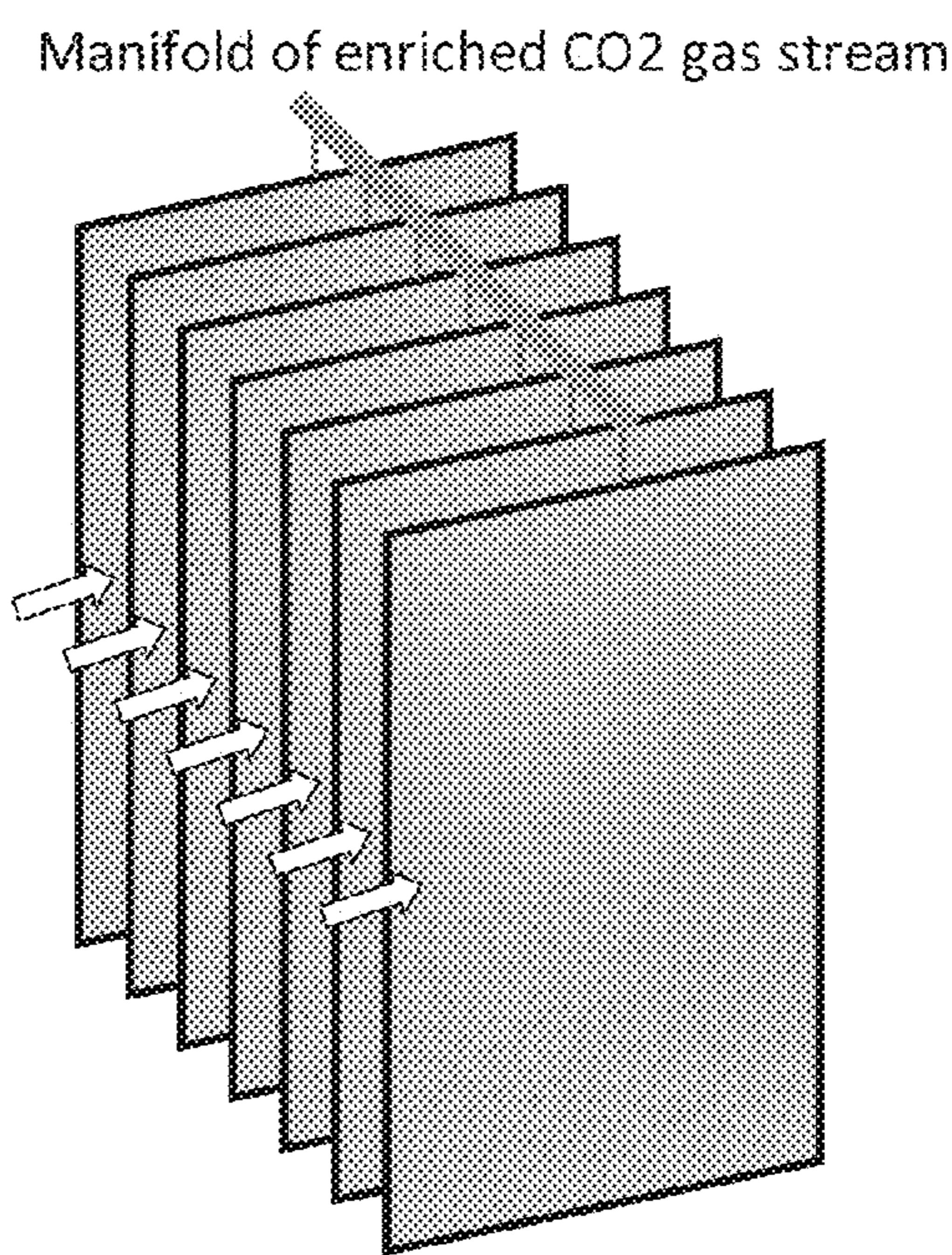
(b) membrane module assembled from a number of units
