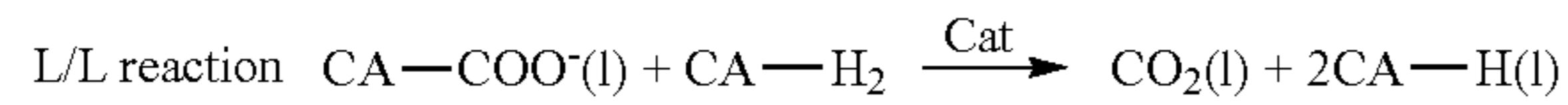
**[0100]** Carbon dioxide loading into the liquid increases with the concentration of the coupling agent. The selective reaction of  $\text{CO}_2$  with the coupling agent over the other molecules makes the facilitated transport process prevail over the physical absorption. In this way, both high  $\text{CO}_2$  selectivity and permeance are obtained, because the selectivity difference in physical absorption between  $\text{CO}_2$  and other molecules is small.
