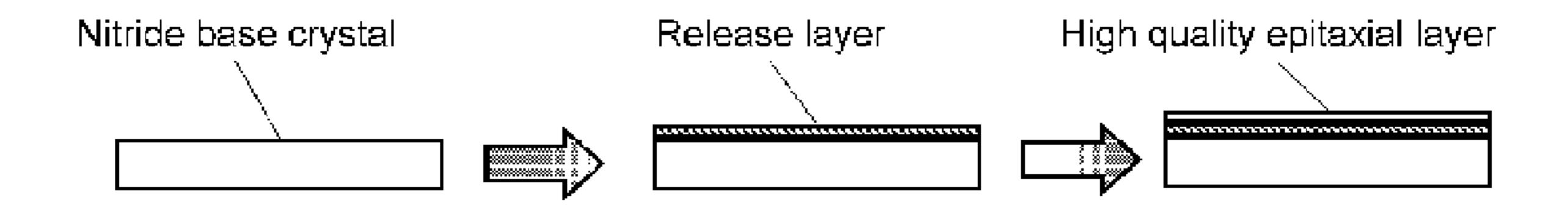
Fig. 1: Substrate fabrication
