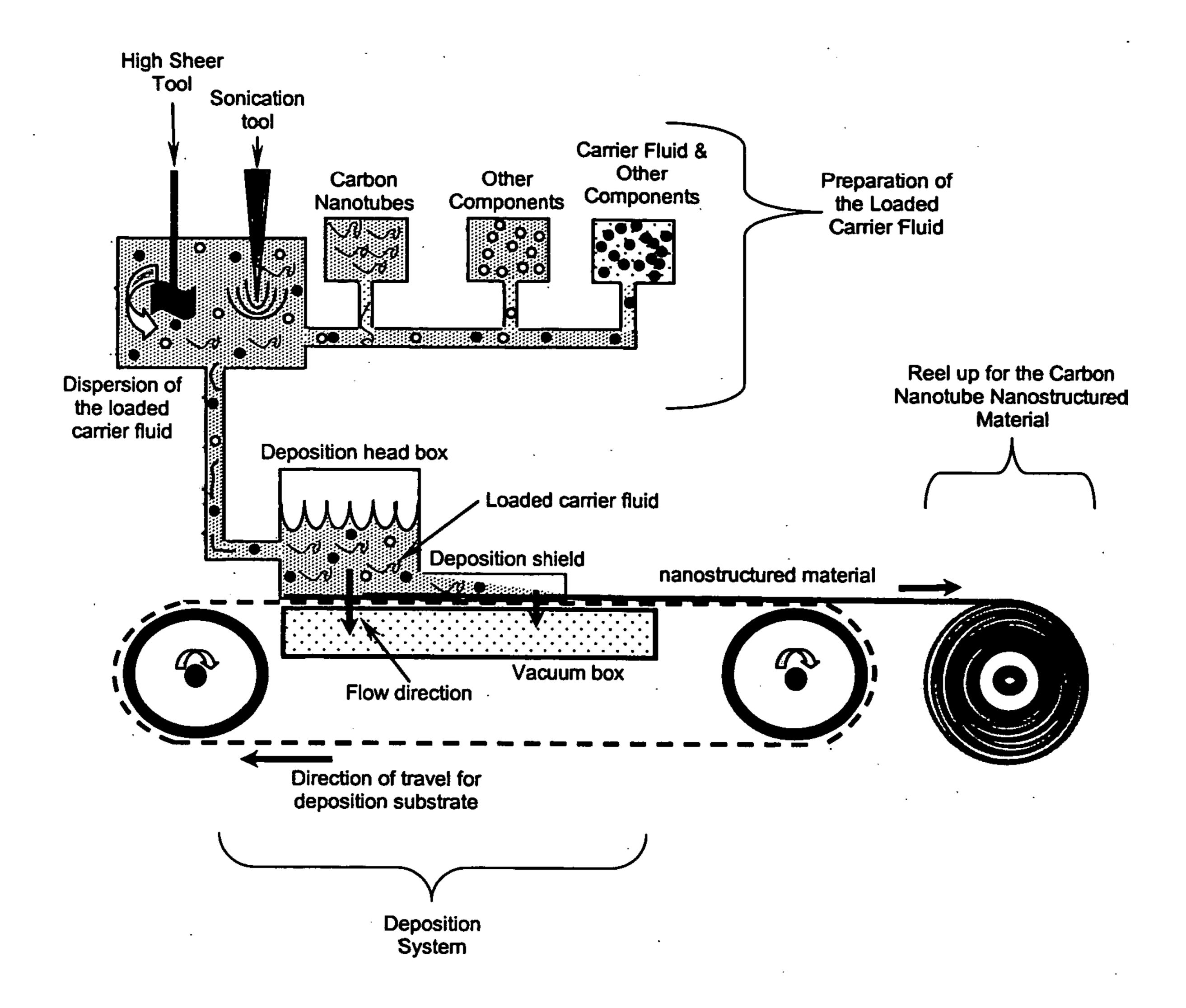
Figure 1. A Continuous Type Carbon Nanotube
