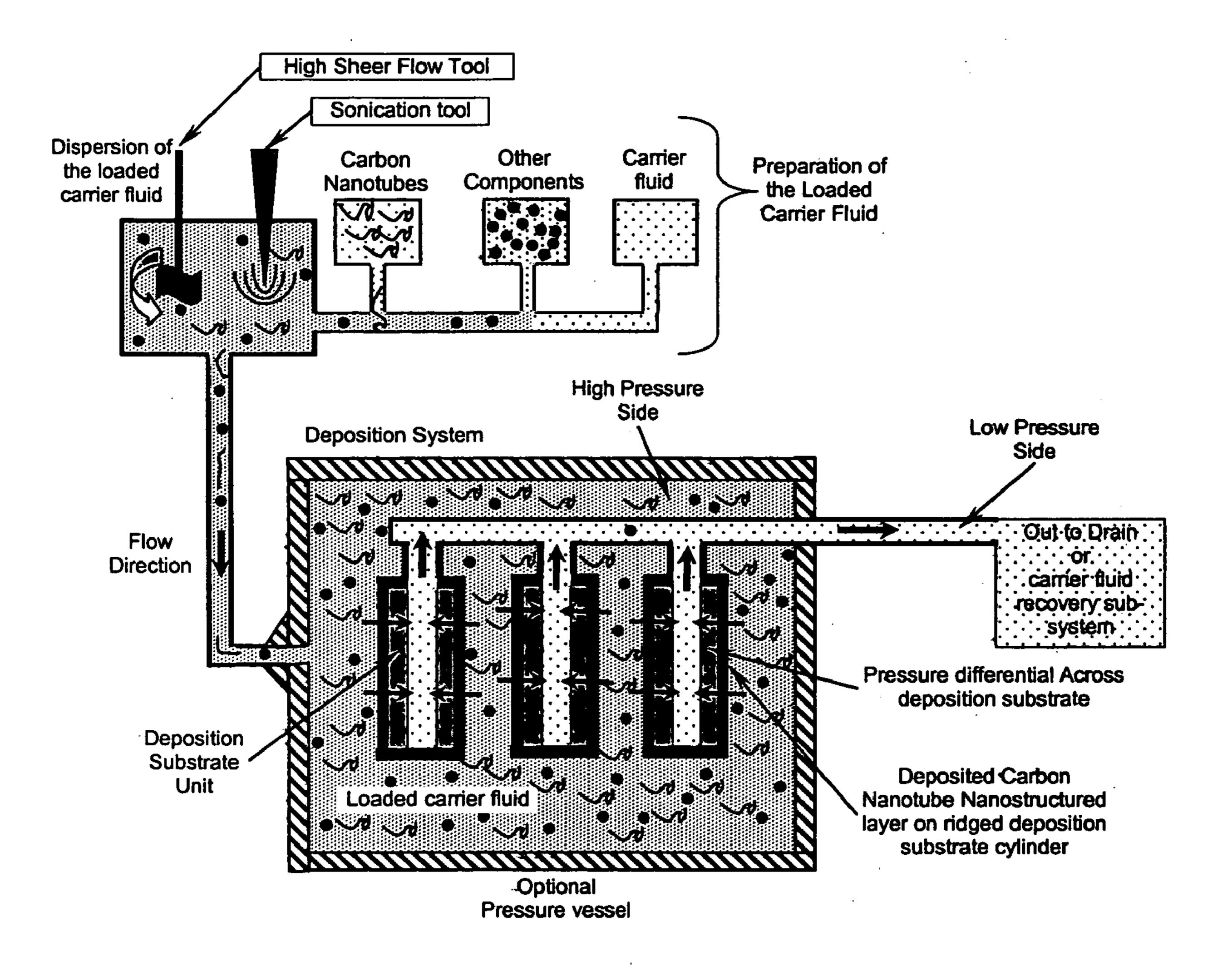
Figure 3. System for the direct deposition of carbon nanostructured material on a rigid substrate to form a seamless product
