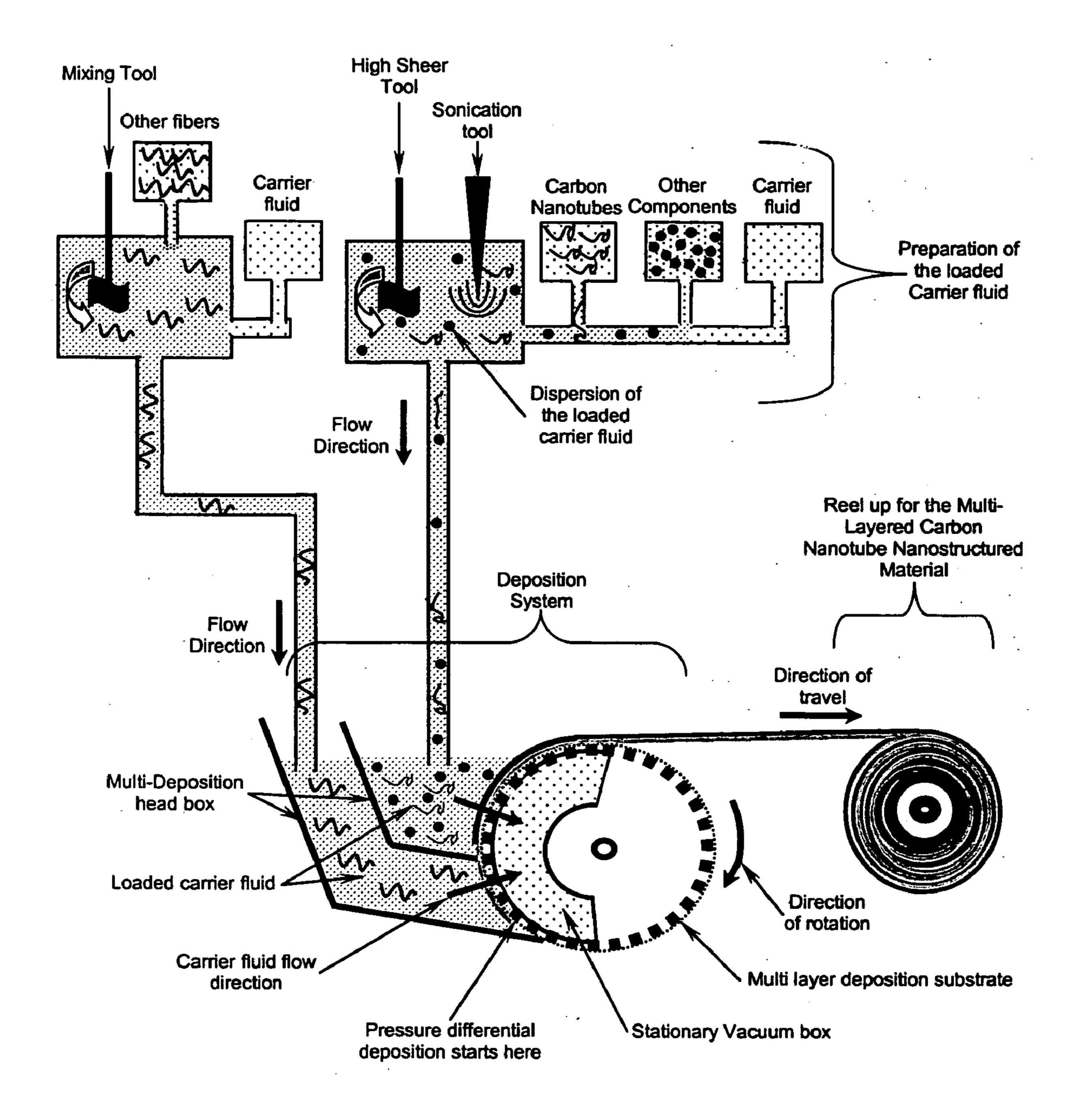
Figure 2. Cross-Section of Roto-former Nanostructured material Deposition System
