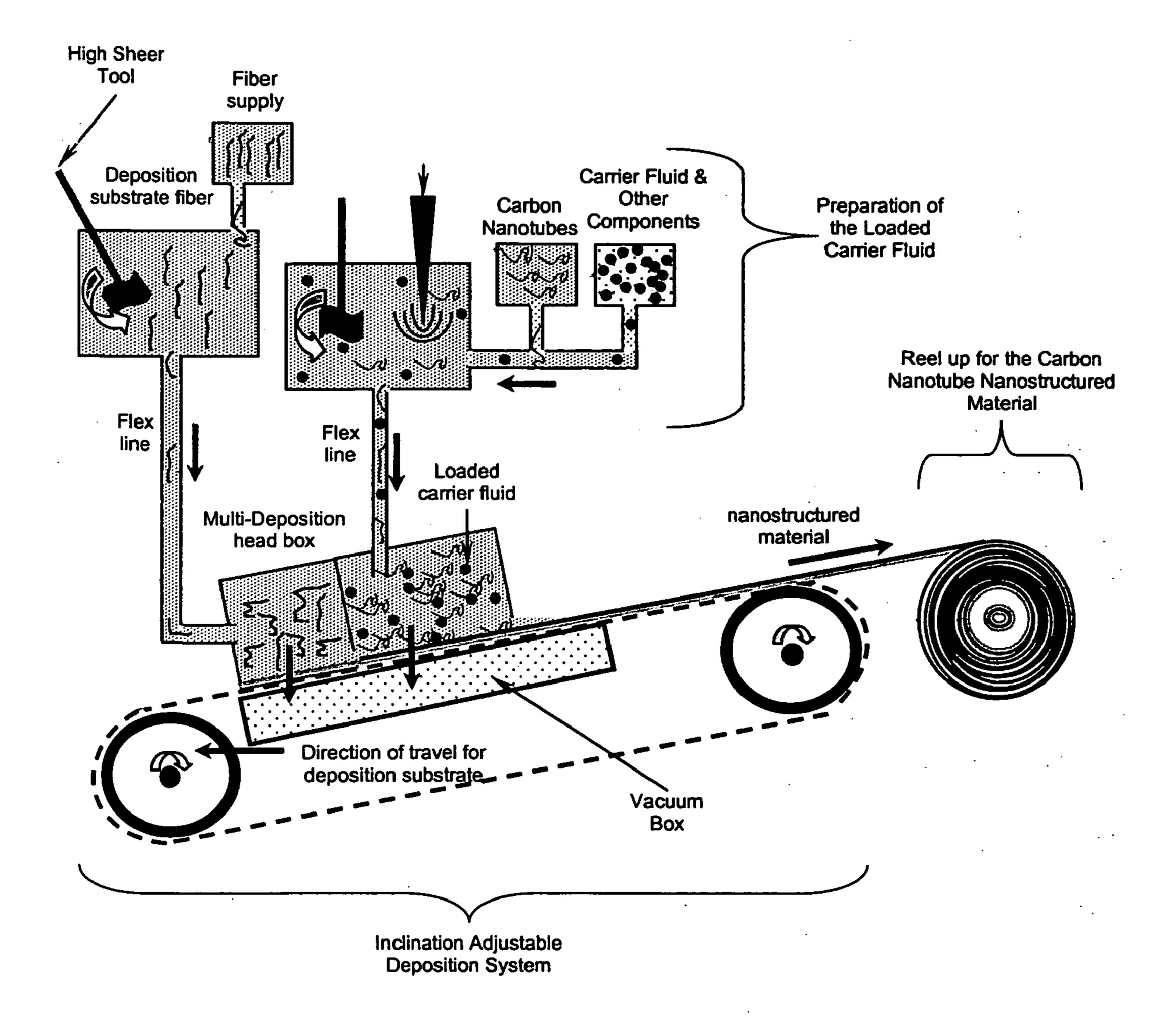
Figure 4. A continuous wire type system for making carbon nanotube nanostructured material.
