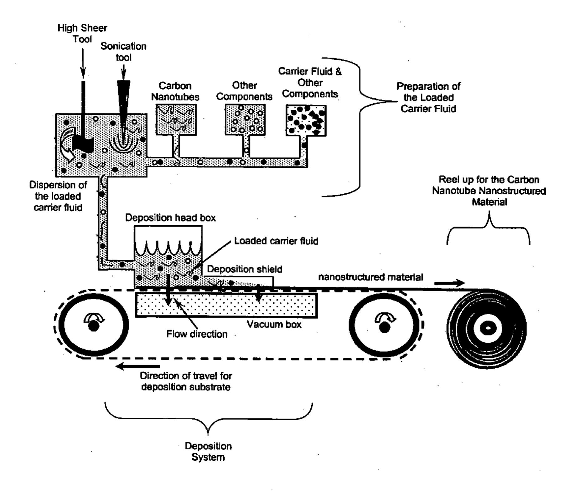
A Continuous Type Carbon Nanotube Nanostructured Material Fabrication System
