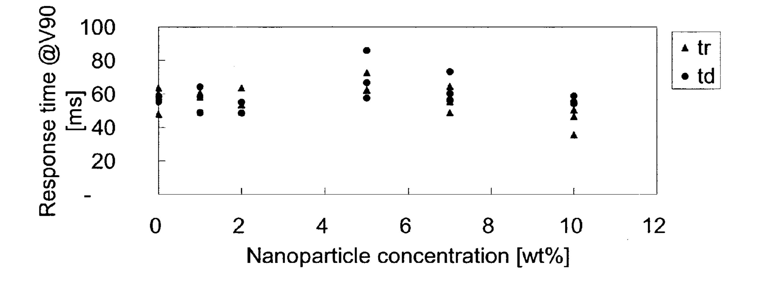
Fig. 5. Response time dependency with nanoparticle concentration. No clear trend was observed. tr is the time required to switch LC on when V90 is applied. td is the time required to switch LC off when V90 is turned off.
