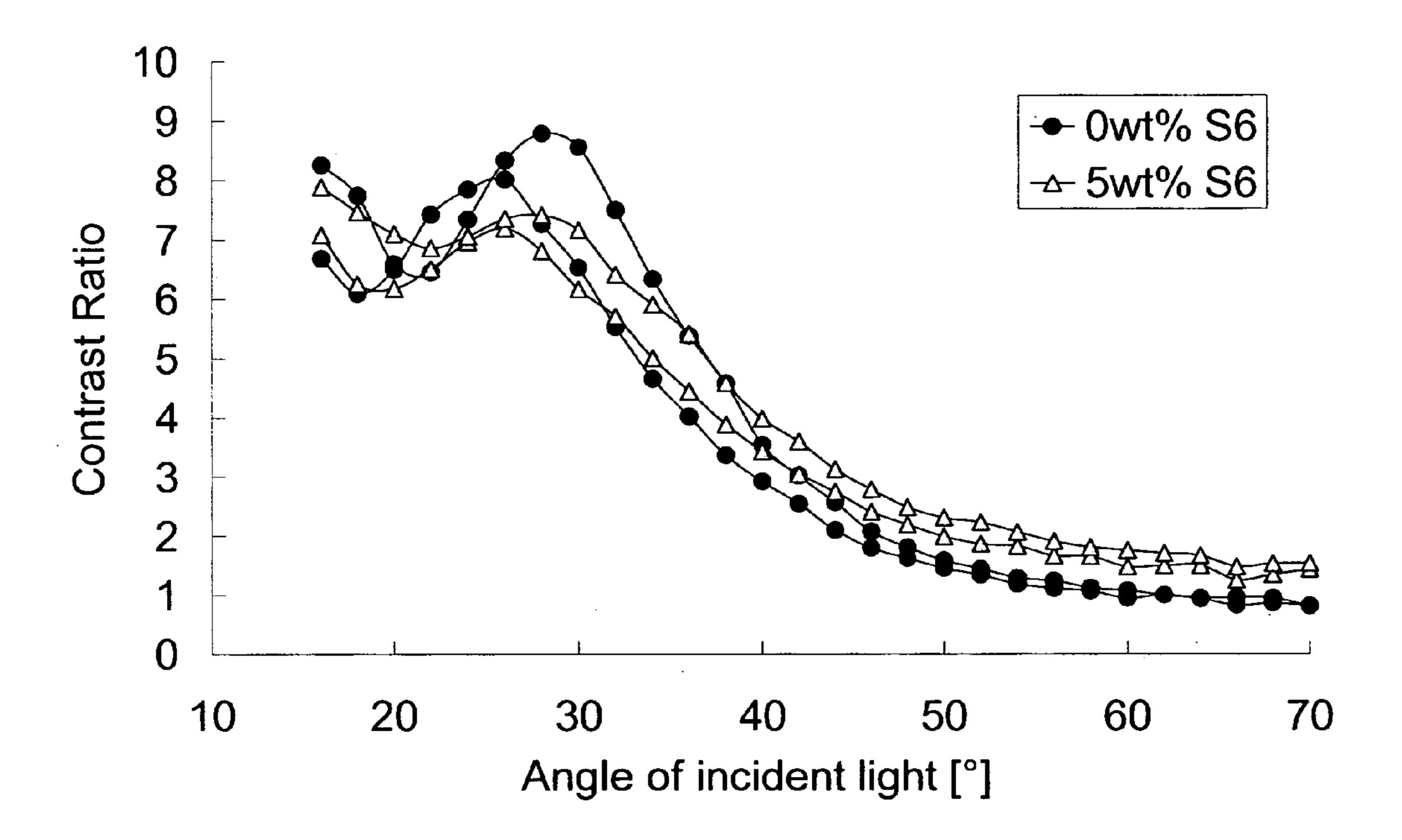
Fig. 7. Contrast ratio dependency with the angle of incident light. The contrast ratio decrease is less steep with 5 wt% S6 nanoparticle doped D-PDLC.
