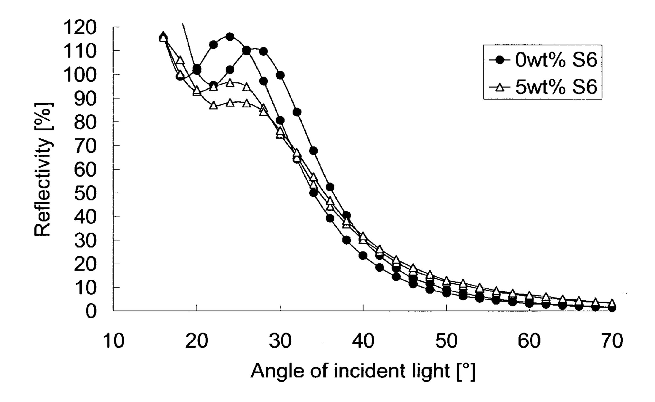
Fig. 6. Reflectivity dependency with the angle of incident light. The reflectivity decrease is less steep with 5 wt% S6 nanoparticle doped D-PDLC.
