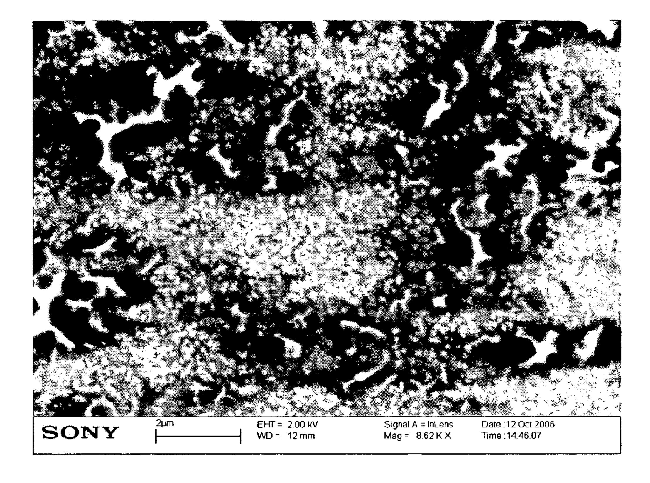
Fig. 2. SEM image of nanoparticle doped PDLC. S6 melamine-formaldehyde resin nanoparticles remain in the PDLC film even after the LC is washed with a solvent.
