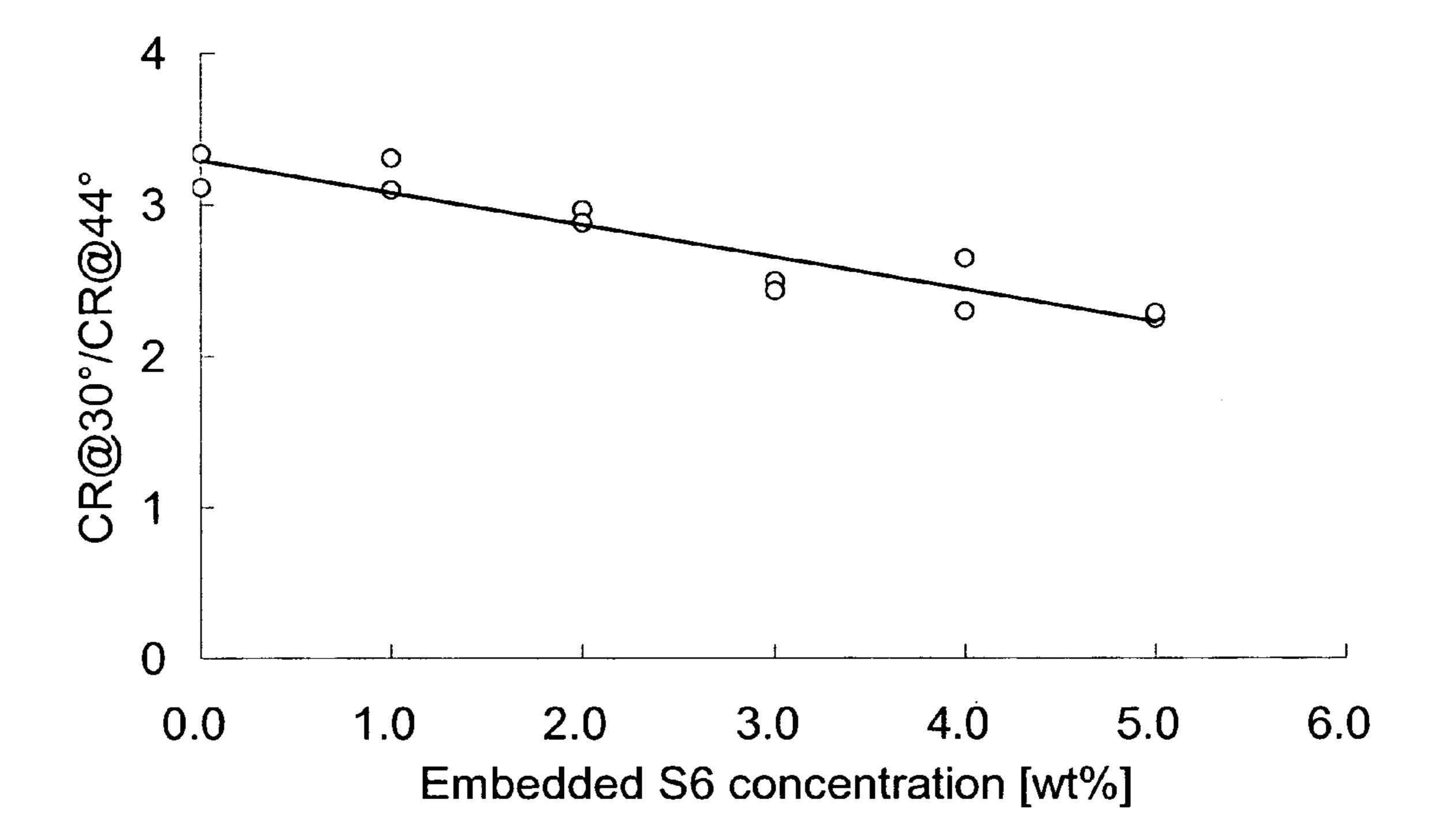
Fig. 8. Ratio of the contrast ratios at 30° and 44°. Decrease in the ratio shows that the viewing angle dependency decreases with S6 nanoparticle doping.
