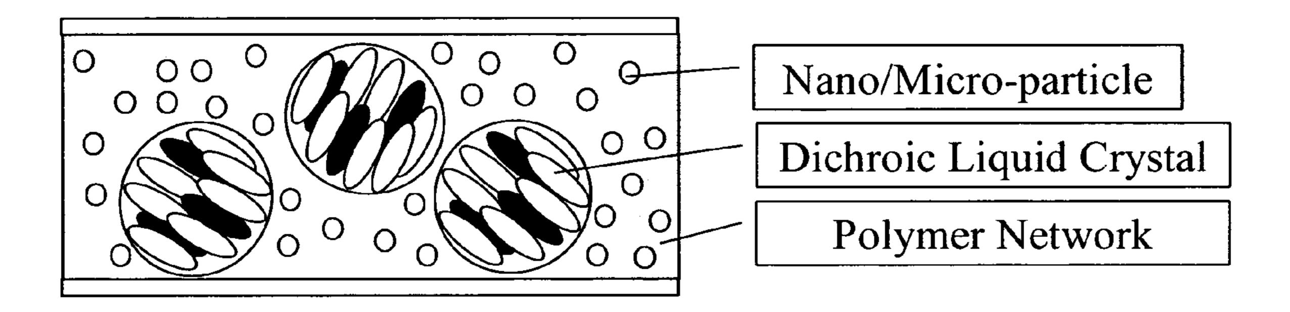
Fig. 1. Schematic drawing of nanoparticle embedded D-PDLC.
