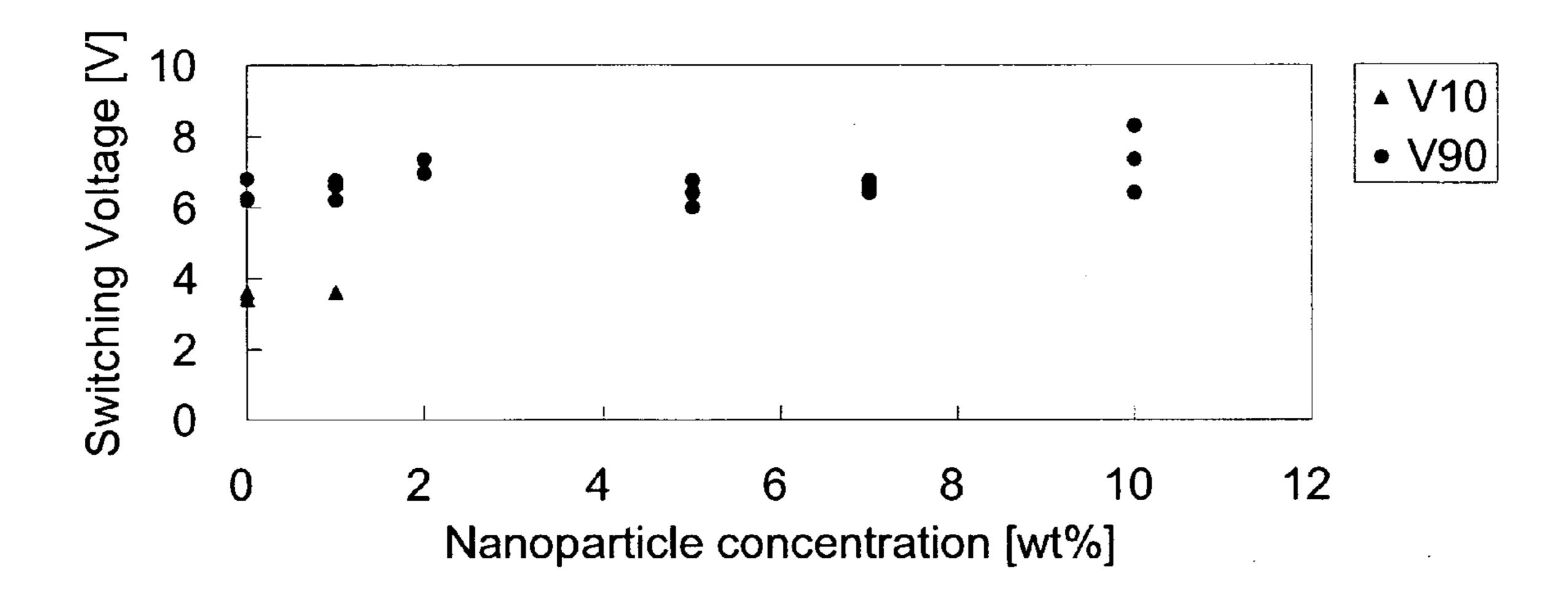
Fig. 4. Switching voltage dependency with nanoparticle concentration. No clear trend was observed. V10 is a voltage required to switch LC to 10% transmittance. V90 is a voltage required to switch LC to 90% transmittance.
