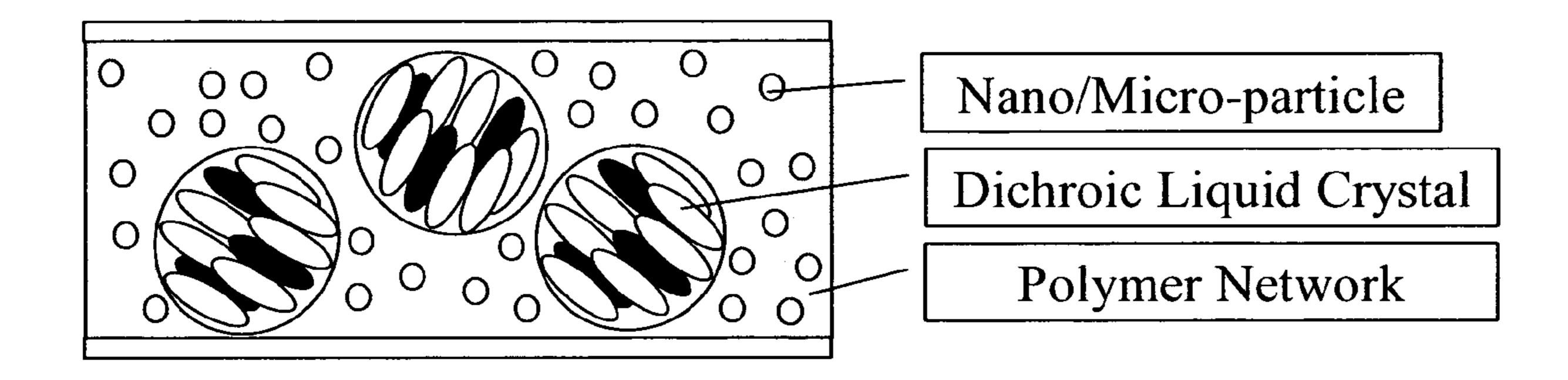
Schematic drawing of nanoparticle embedded D-PDLC.
