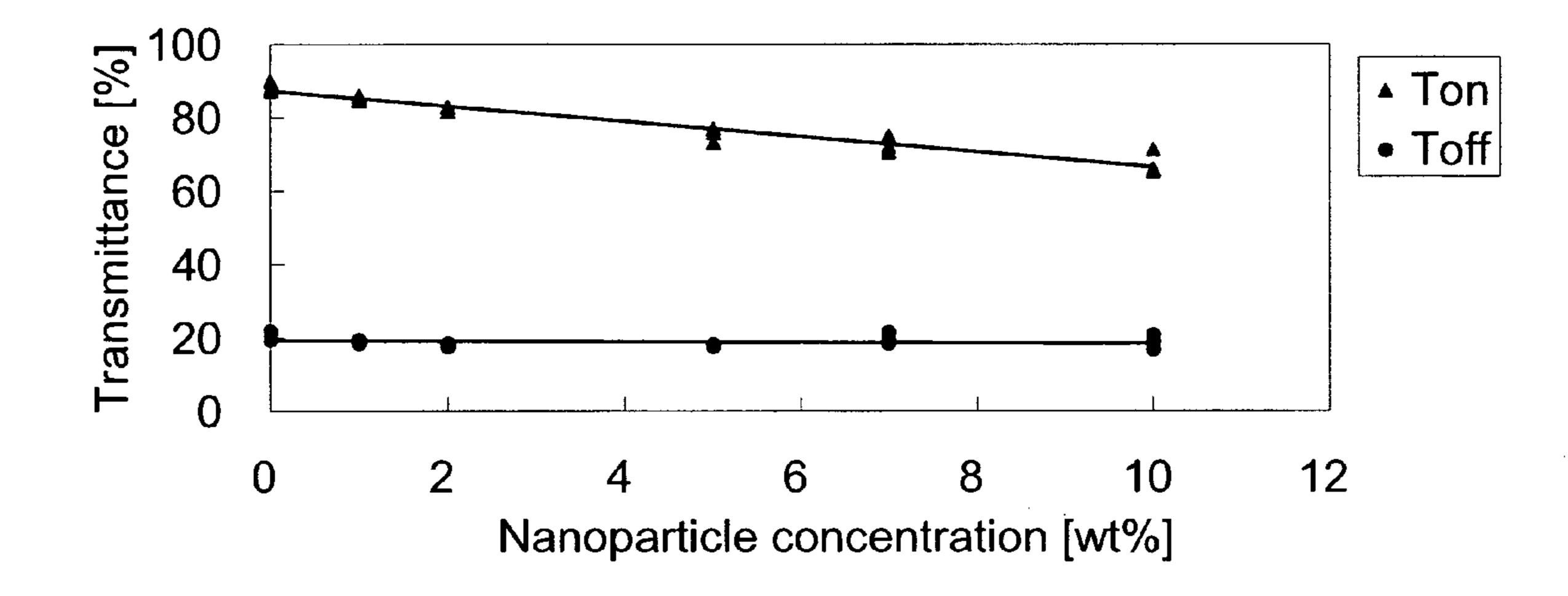
Fig. 3. On-state (Ton) & off-state (Toff) transmittance dependency with nanoparticle concentration. Ton decreases because of the scattering introduced by nanoparticles in polymer matrix.
