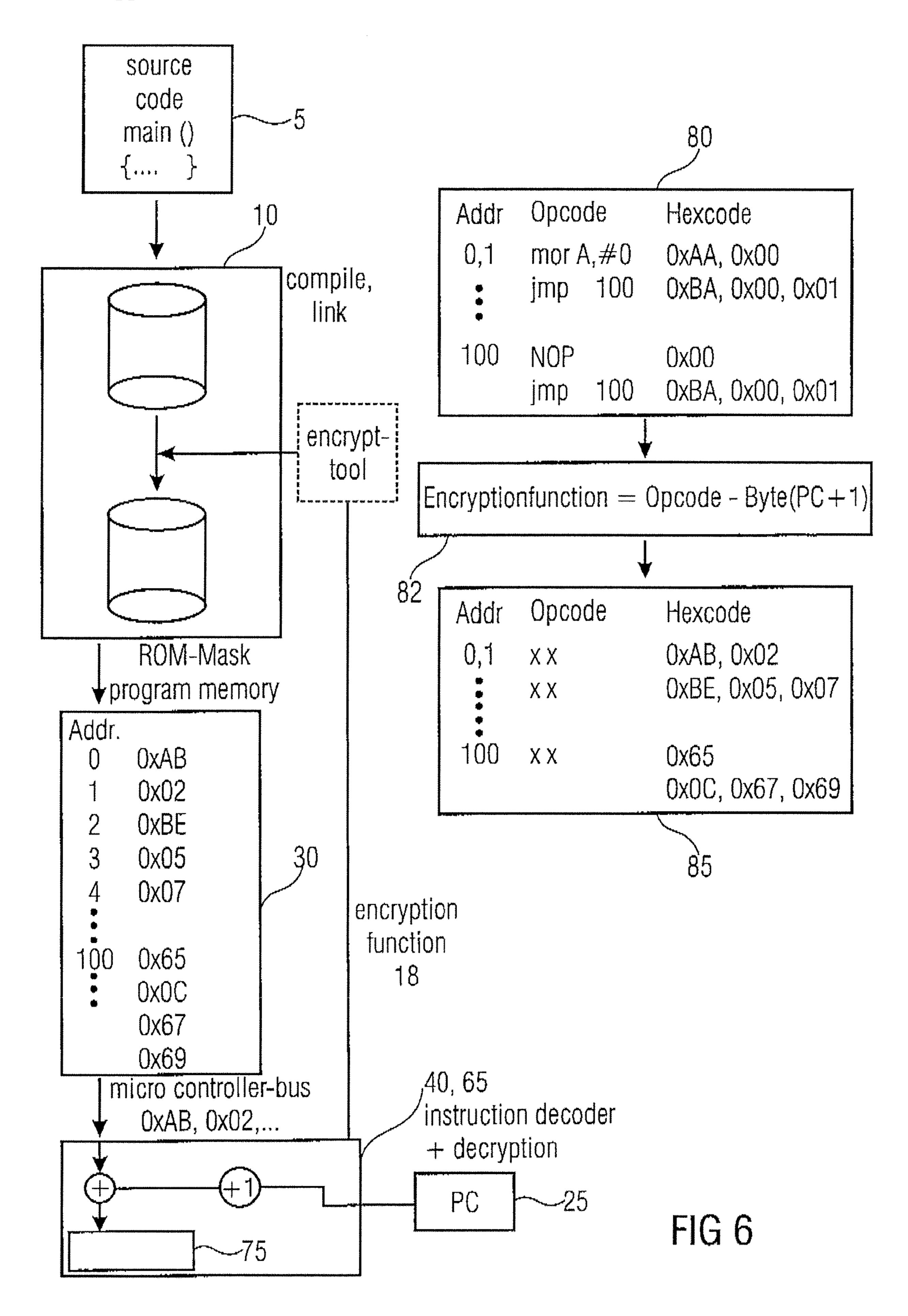
Compiling a source code into a machine language code for a processing unit
