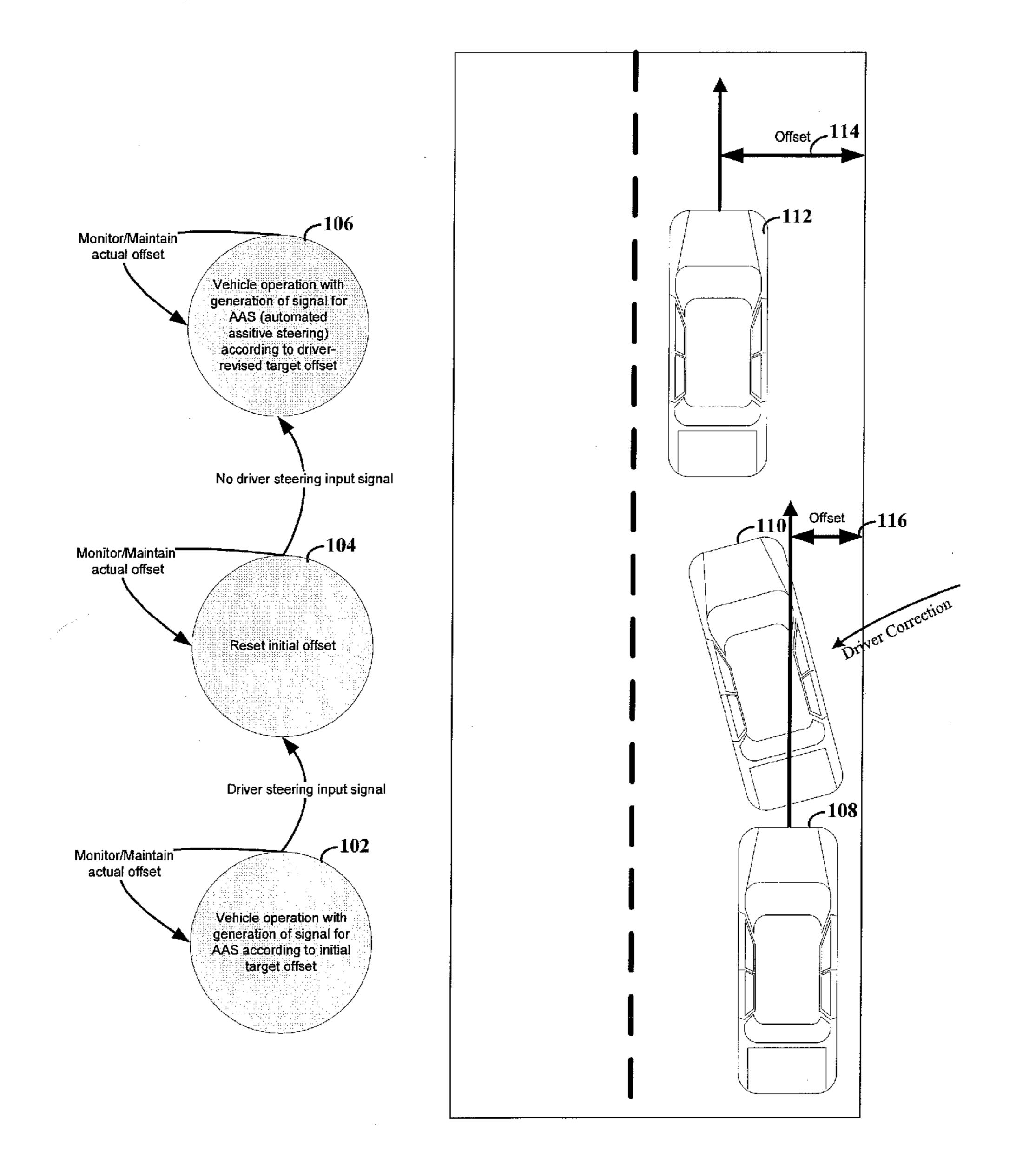
FIG. 1 Monitor/Maintain actual offset Vehicle operation with generation of signal for AAS (automated assitive steering) according to driverrevised target offset No driver steering input signal **-104** Monitor/Maintain\* actual offset Reset initial offset Driver steering input signal **-102** Monitor/Maintain actual offset Vehicle operation with generation of signal for AAS according to initial target offset
