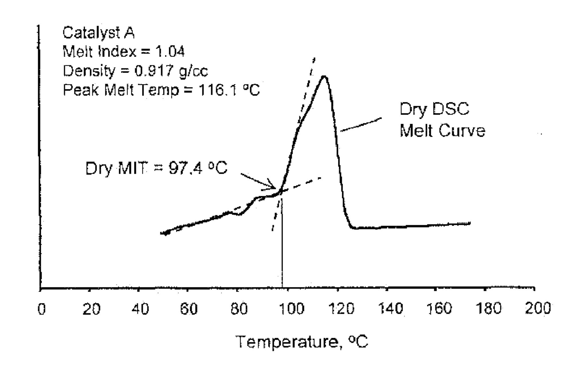
Figure 4 – Displaced MIT (MIT<sub>R</sub>)
