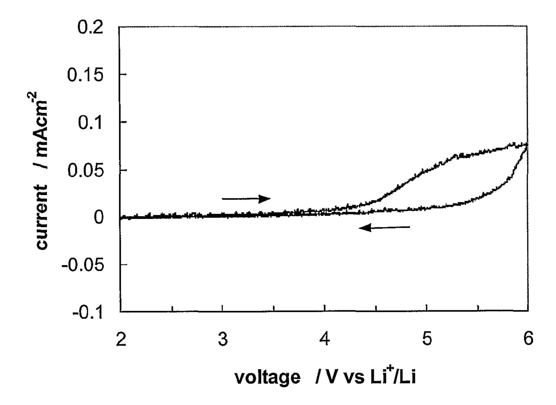
Figure 10C. Lithium deposition-stripping process and electrochemical oxidation of 80% EC-PC plasticized P(LiOEG<sub>3</sub>B) on aluminum electrode, at a scan rate of 1 mVs<sup>-1</sup> at room temperature. Al area =  $1.963 \times 10^{-3}$  cm<sup>2</sup>.
