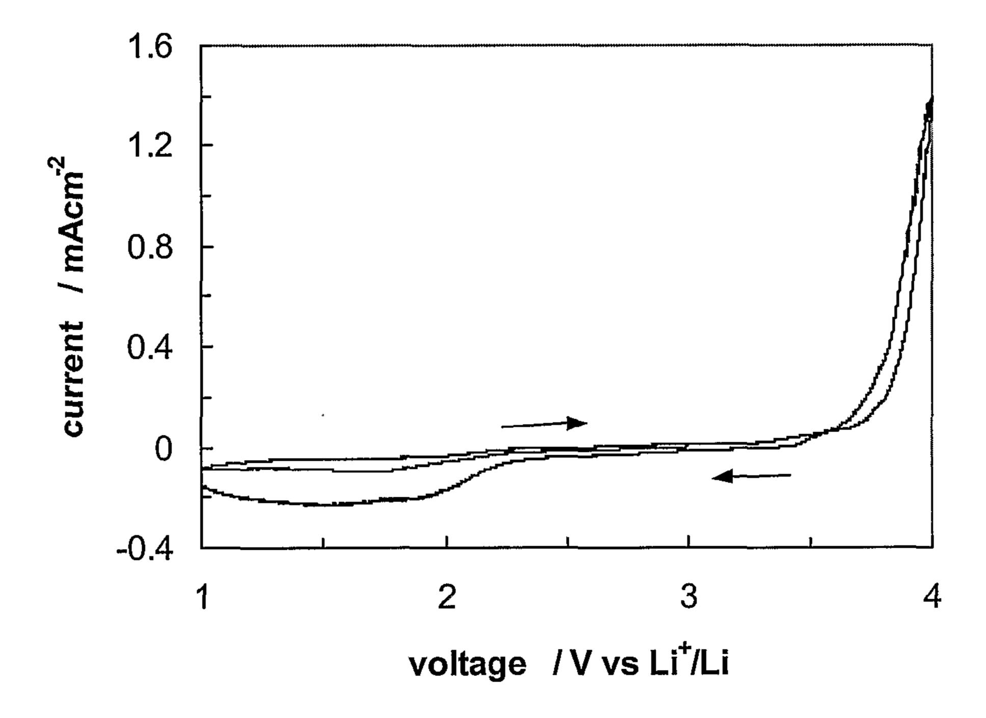
Figure 10D. Lithium deposition-stripping process and electrochemical oxidation of 80% EC-PC plasticized P(LiOEG<sub>3</sub>B) on copper electrode, at a scan rate of 1 mVs<sup>-1</sup> at room temperature. Cu area =  $1.963 \times 10^{-3}$  cm<sup>2</sup>.
