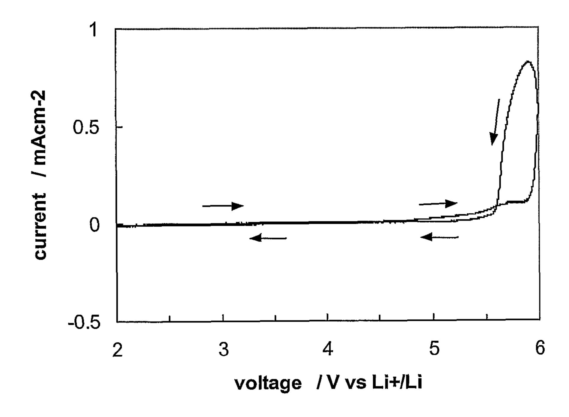
Figure 10A. Lithium deposition-stripping process and electrochemical oxidation of 80% EC-PC plasticized P(LiOEG<sub>3</sub>B) on stainless steel electrode, at a scan rate of 1 mVs<sup>-1</sup> at room temperature. SS area =  $1.963 \times 10^{-3}$  cm<sup>2</sup>.
