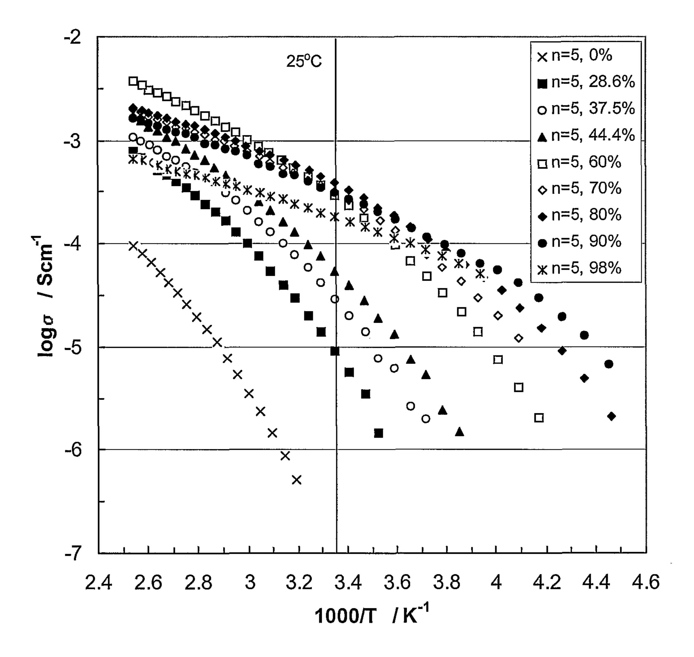
Figure 5B. Temperature dependence of ionic conductivity of EC-PC (1:1) plasticized P(LiOEG<sub>5</sub>B) with different EC-PC content.
