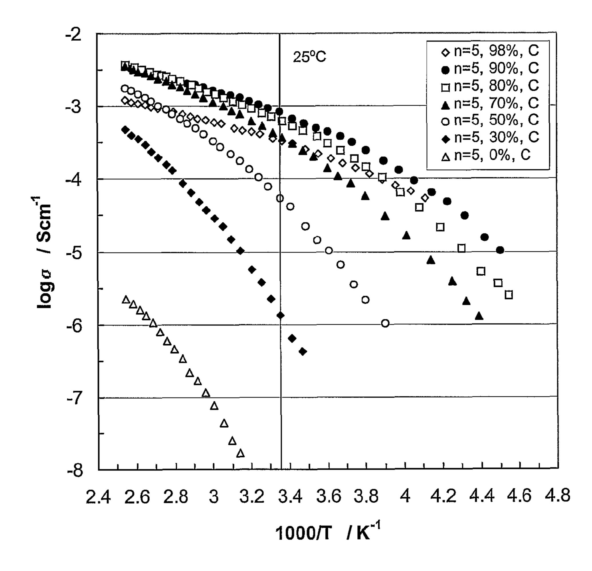
Figure 8A. Temperature dependence of ionic conductivity of EC-PC (1:1 by wt) plasticized LiBH<sub>4</sub>-crosslinked P(LiOEG<sub>5</sub>B) with different content of plasticizer.
