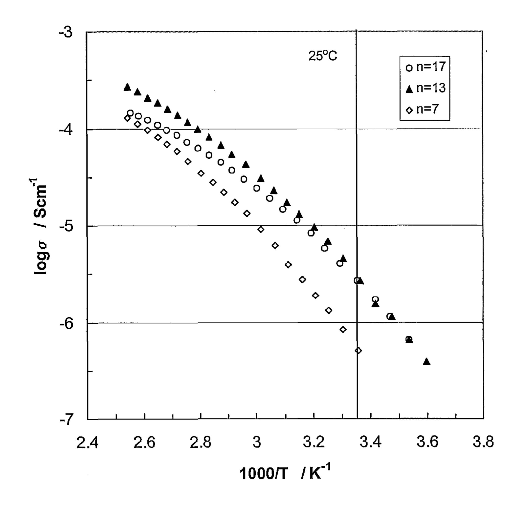
Figure 2. Temperature dependence of ionic conductivities of PPG-spaced polyMOBs, P(LiOPG<sub>n</sub>B), where the length of spacer PG<sub>n</sub> is 7 to 17.
