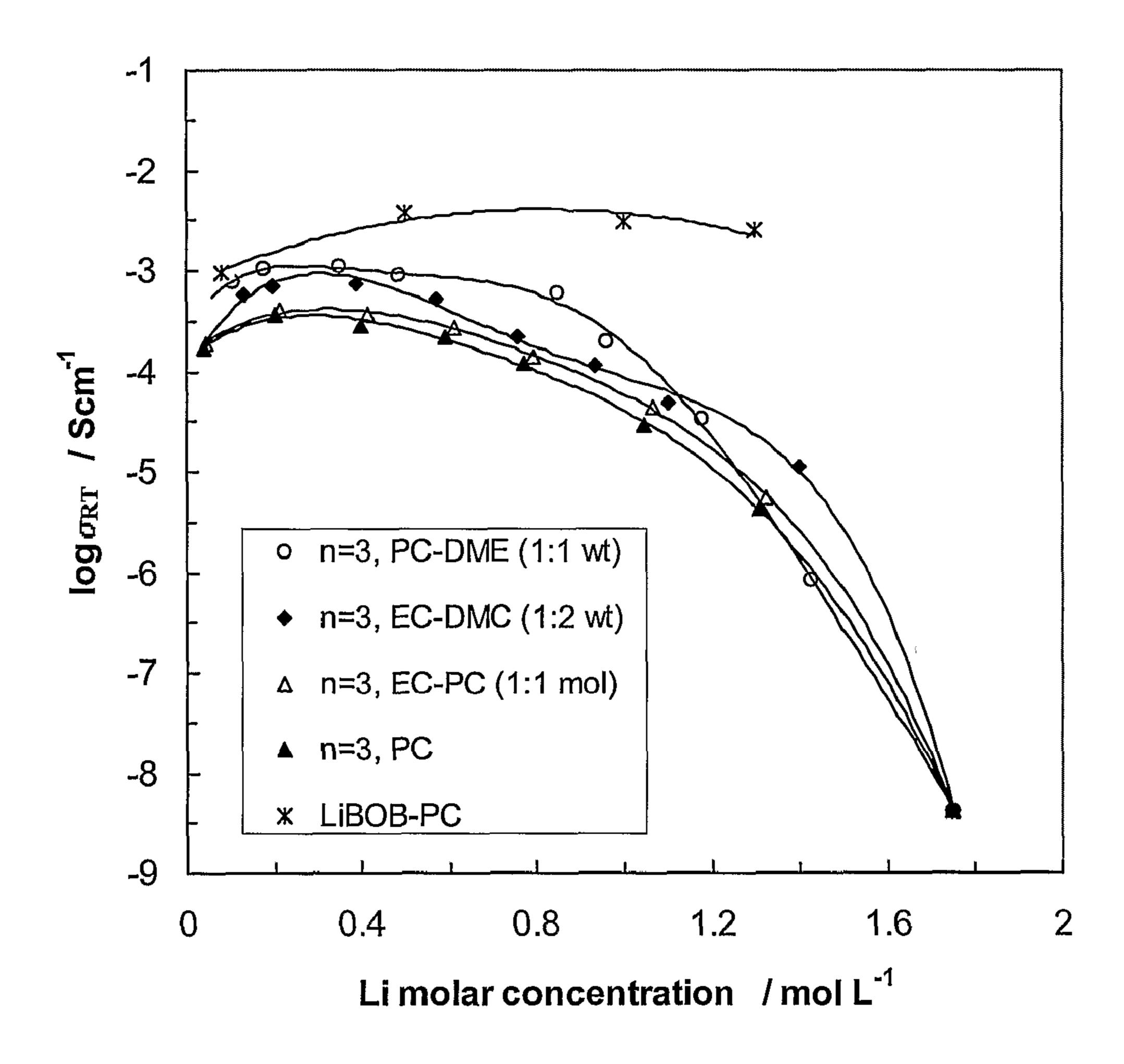
Figure 7. The room temperature conductivity of P(LiOEG<sub>3</sub>B) plasticized by different solvents and solvent mixtures with the variation of lithium concentrations. Comparison is also made with the conductivity of simple LiBOB solutions in PC. Remembering that our conductivity is entirely due to Li<sup>+</sup> cations, these results are seen as highly promising.
