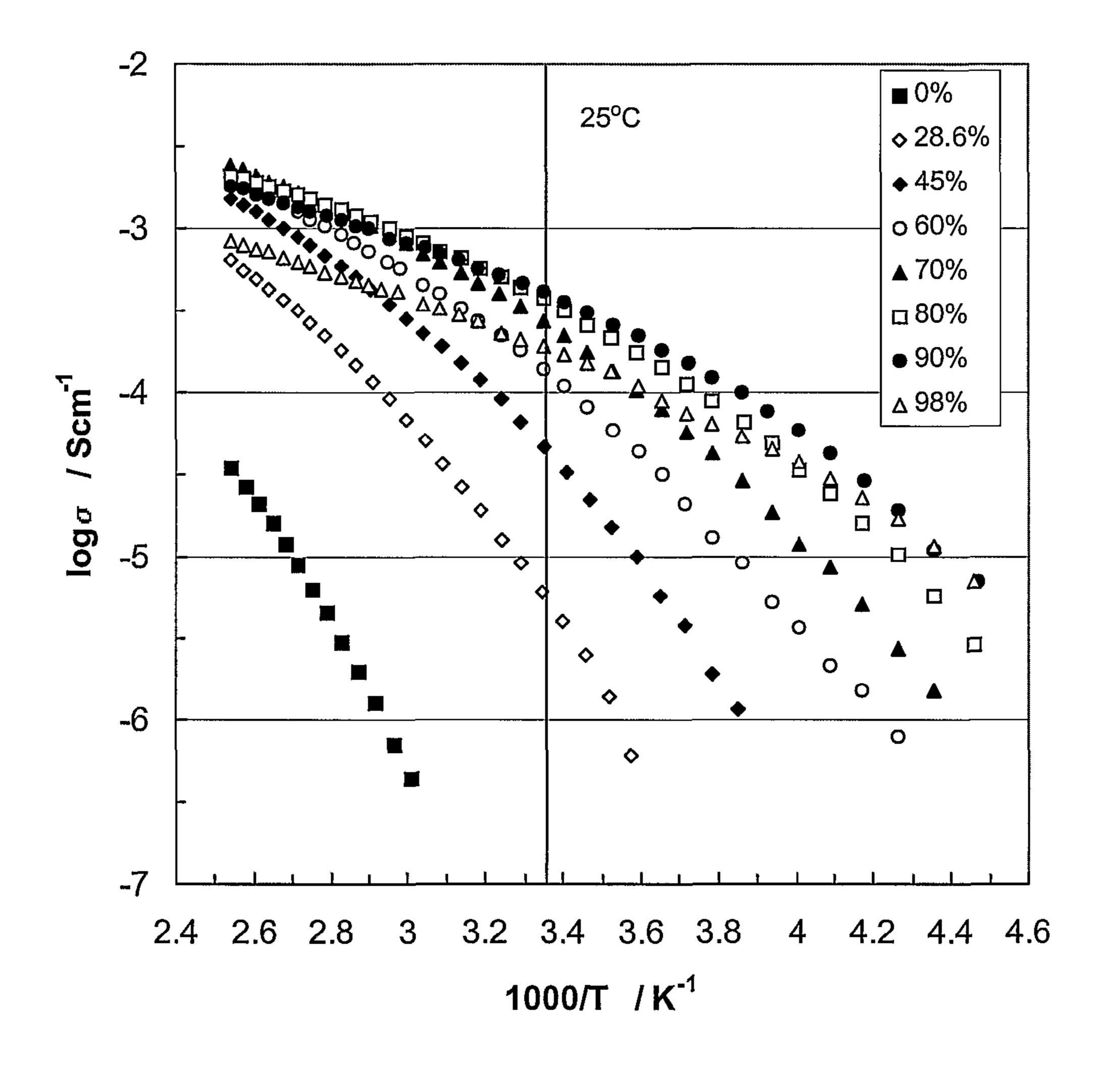
Figure 5A. Temperature dependence of ionic conductivity of EC-PC (1:1) plasticized P(LiOEG<sub>3</sub>B) with different EC-PC content.
