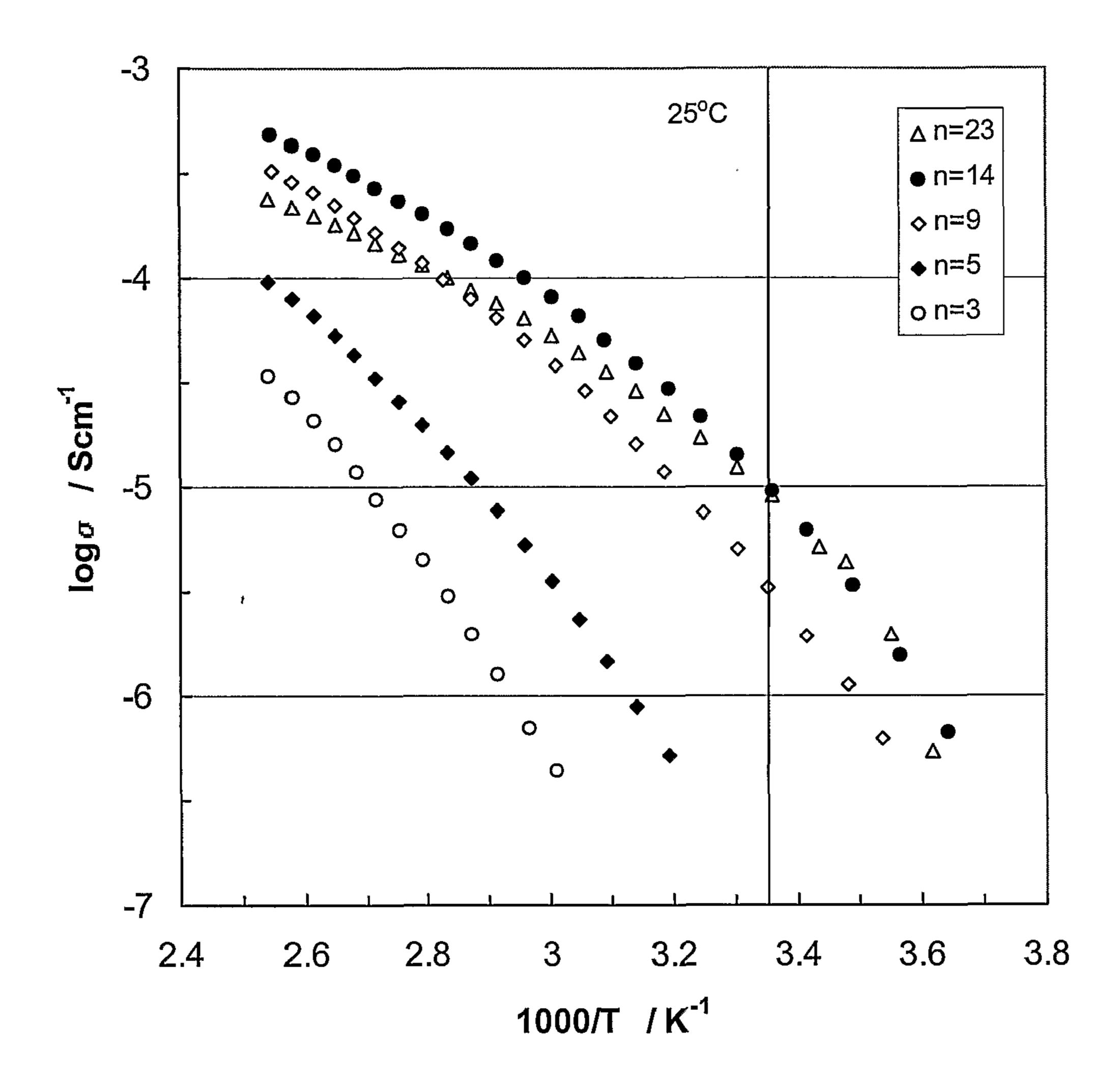
Figure 1. Temperature dependence of ionic conductivities of PEG-spaced polyMOBs, P(LiOEG<sub>n</sub>B), where the length of spacer EG<sub>n</sub> is 3 to 23.
