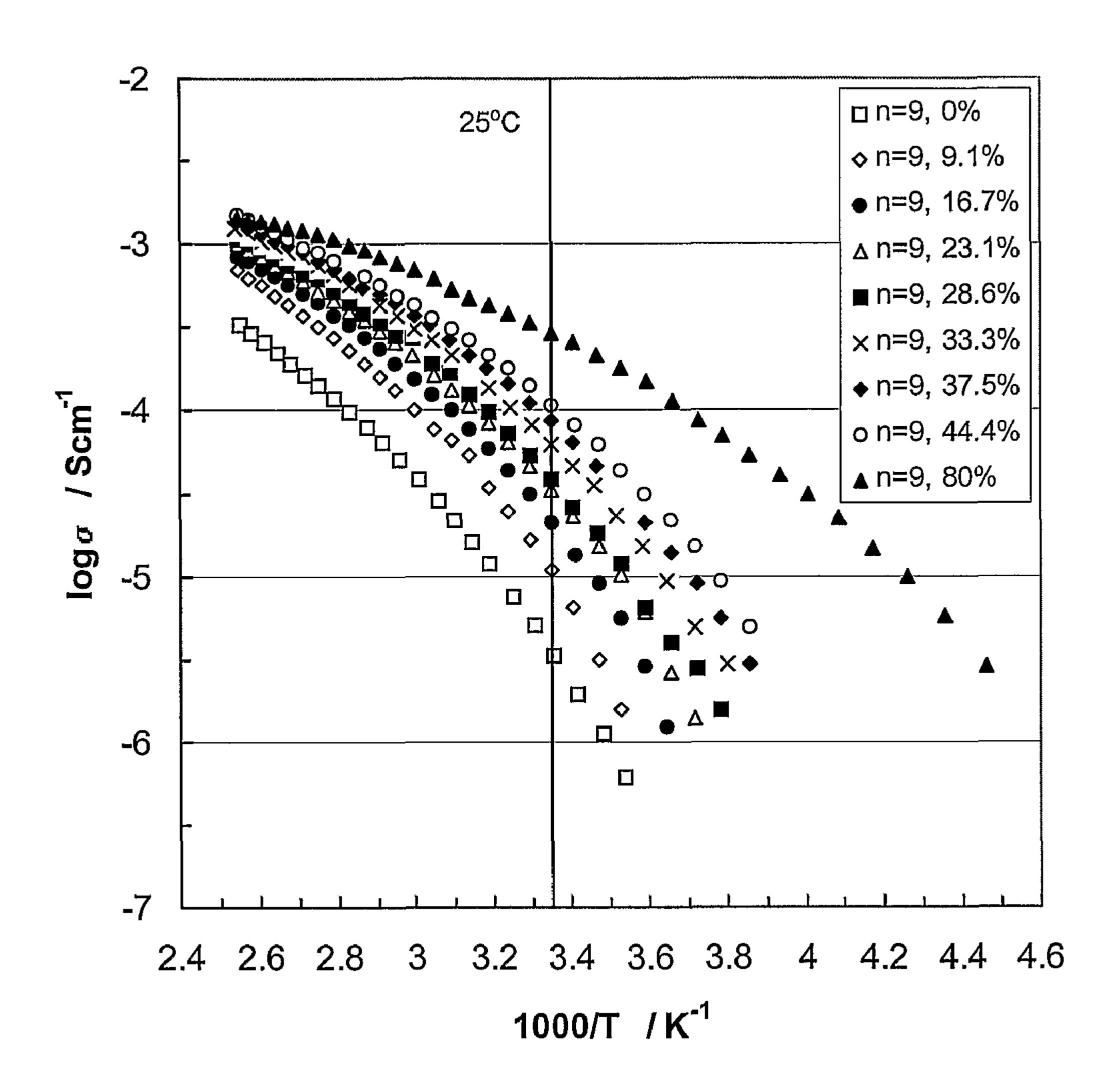
Figure 5C. Temperature dependence of ionic conductivity of EC-PC (1:1) plasticized P(LiOEG<sub>9</sub>B) with different EC-PC content.
