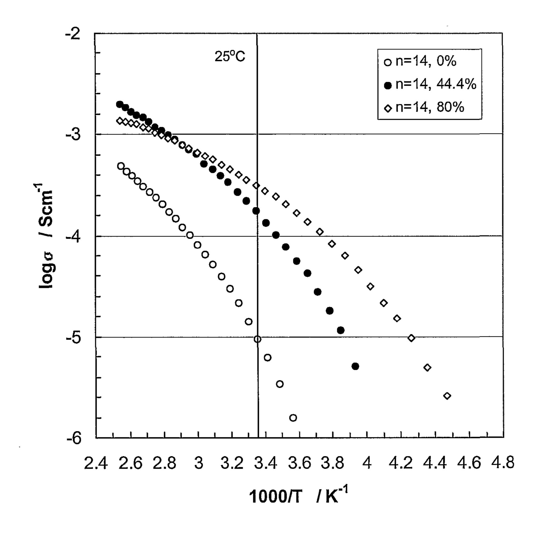
Figure 5D. Temperature dependence of ionic conductivity of EC-PC (1:1) plasticized P(LiOEG<sub>14</sub>B) with different EC-PC content.
