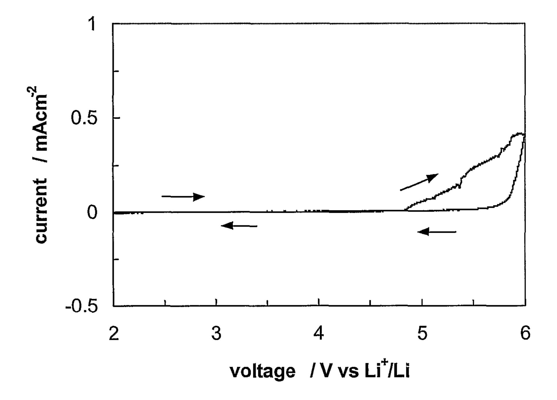
Figure 10B. Lithium deposition-stripping process and electrochemical oxidation of 80% EC-PC plasticized P(LiOEG<sub>3</sub>B) on nickel electrode, at a scan rate of 1 mVs<sup>-1</sup> at room temperature. Ni area =  $1.963 \times 10^{-3}$  cm<sup>2</sup>.
