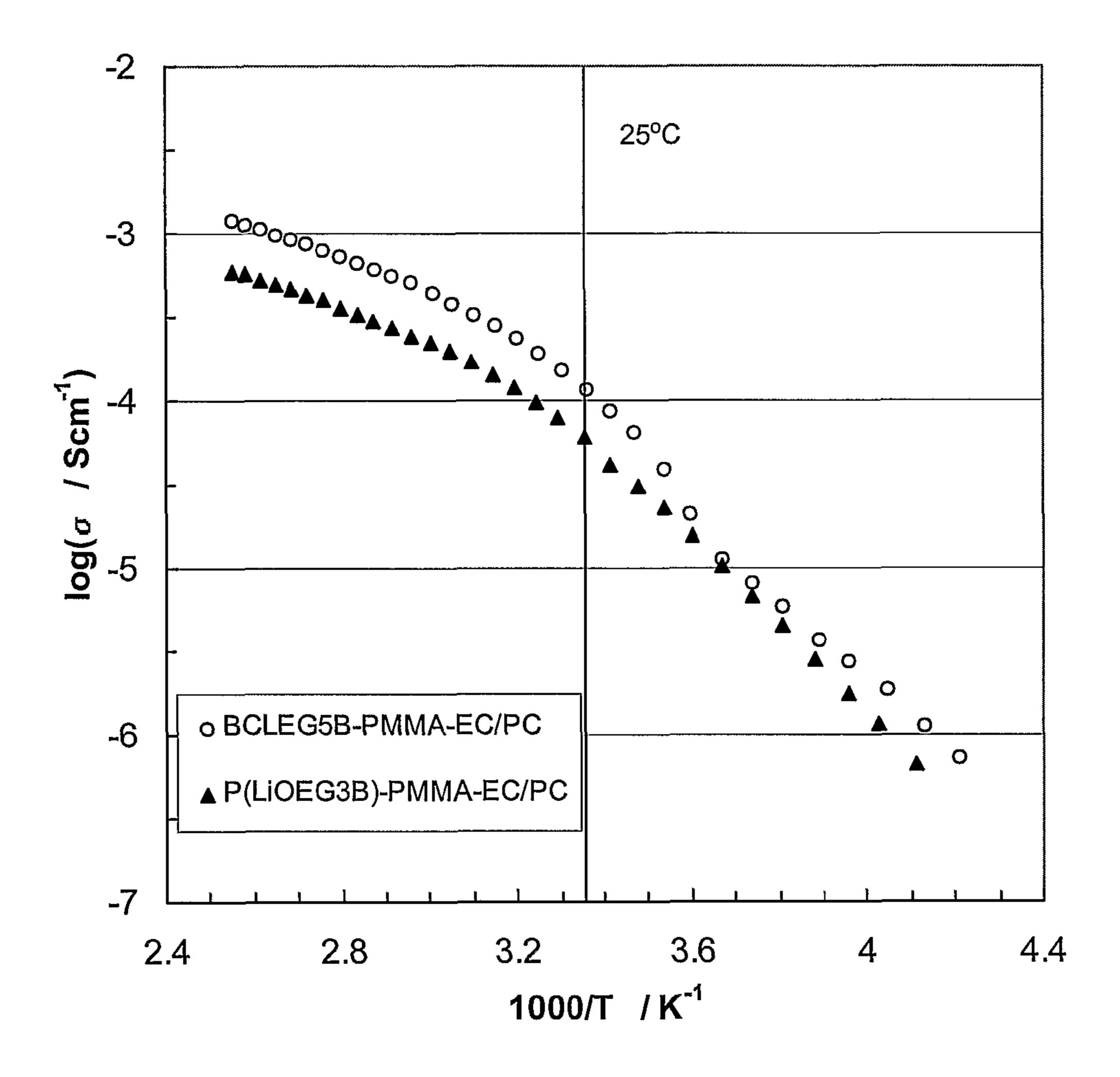
**Figure 9.** Temperature dependence of ionic conductivities of two gel electrolytes with composition of 20.92 PPMA-8.09 P(LiOEG3B)-35.45 EC-35.44 PC (Example 8), and 21.05 PMMA-7.91 BCLEG5B-35.53 EC-35.52 PC (Example 9), respectively.
