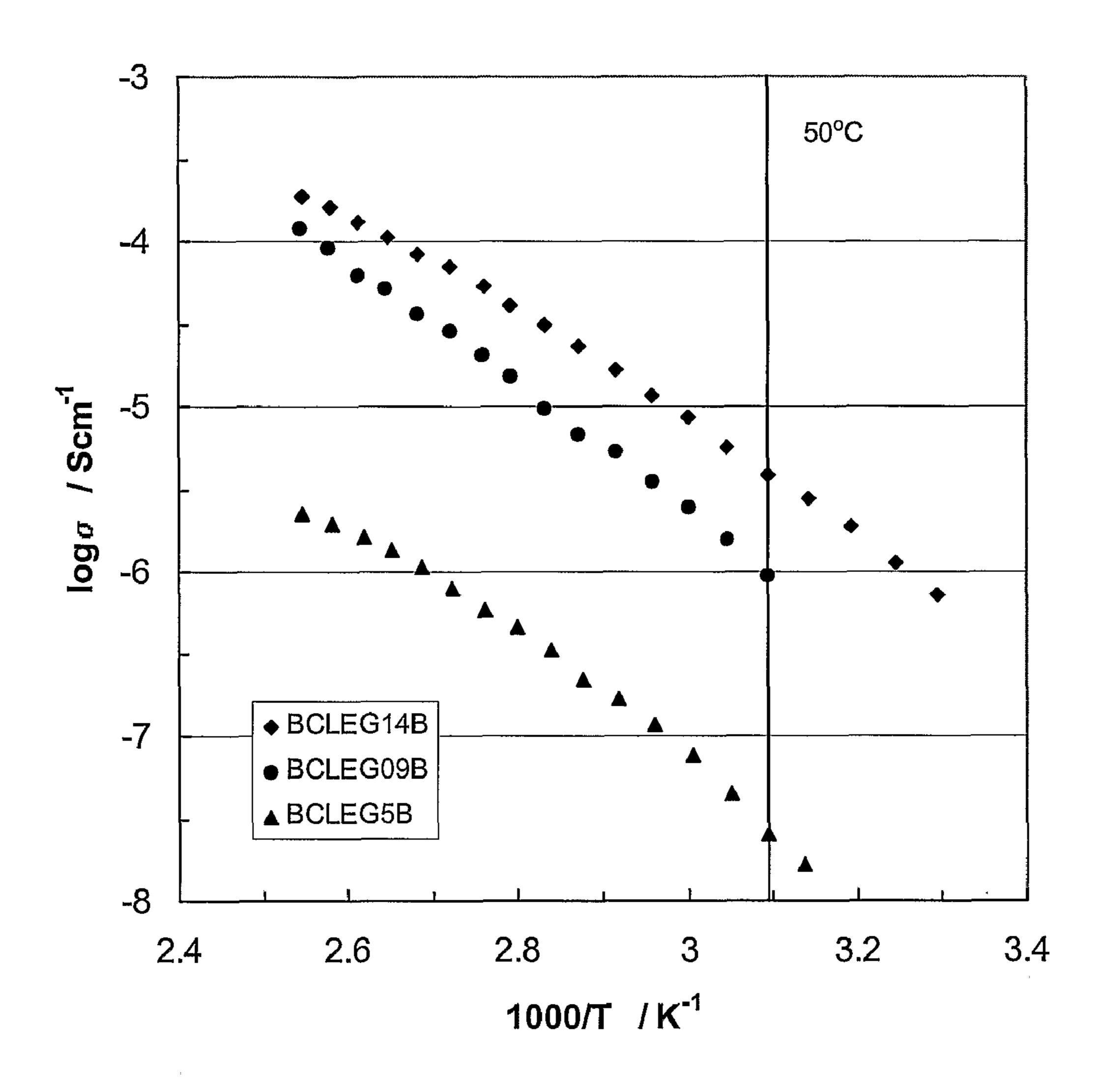
Figure 4. Temperature dependence of ionic conductivities of LiBH<sub>4</sub> crosslinked PEG-spaced polyMOBs, BCLEG<sub>n</sub>B, where the length of spacer EG<sub>n</sub> is 5 to 14.
