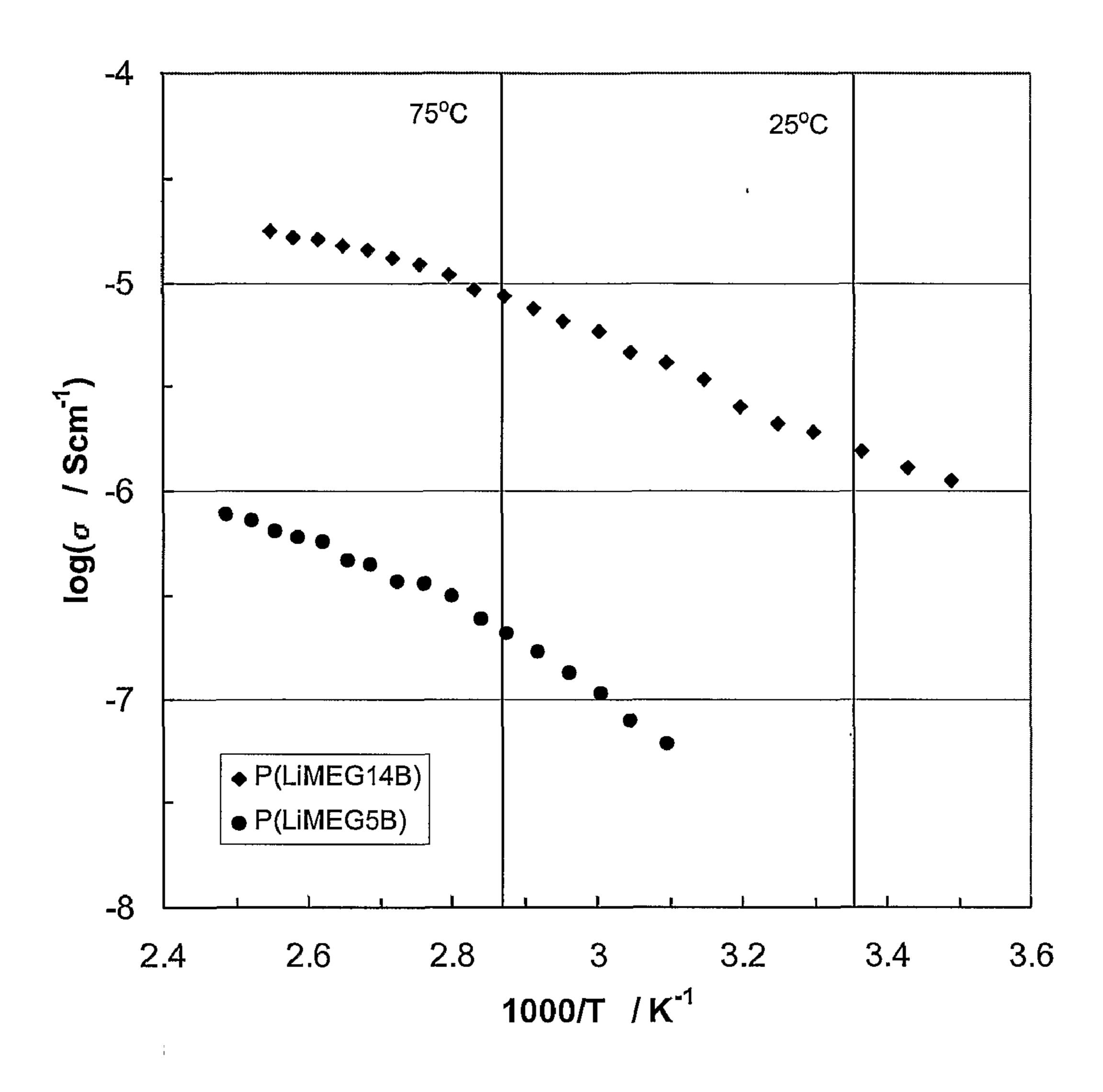
Figure 3. Temperature dependence of ionic conductivities of PEG-spaced polyMMBs, P(LiMEG<sub>n</sub>B), where the length of spacer EG<sub>n</sub> is 5 and 14.
