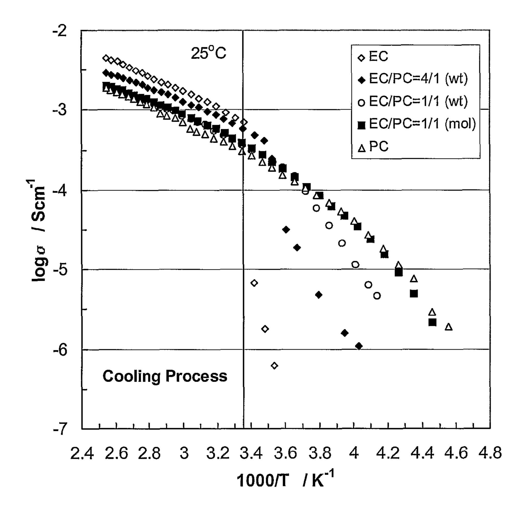
Figure 6. Temperature dependence of ionic conductivity of plasticized P(LiOEG<sub>5</sub>B) by different EC-PC compositions.
