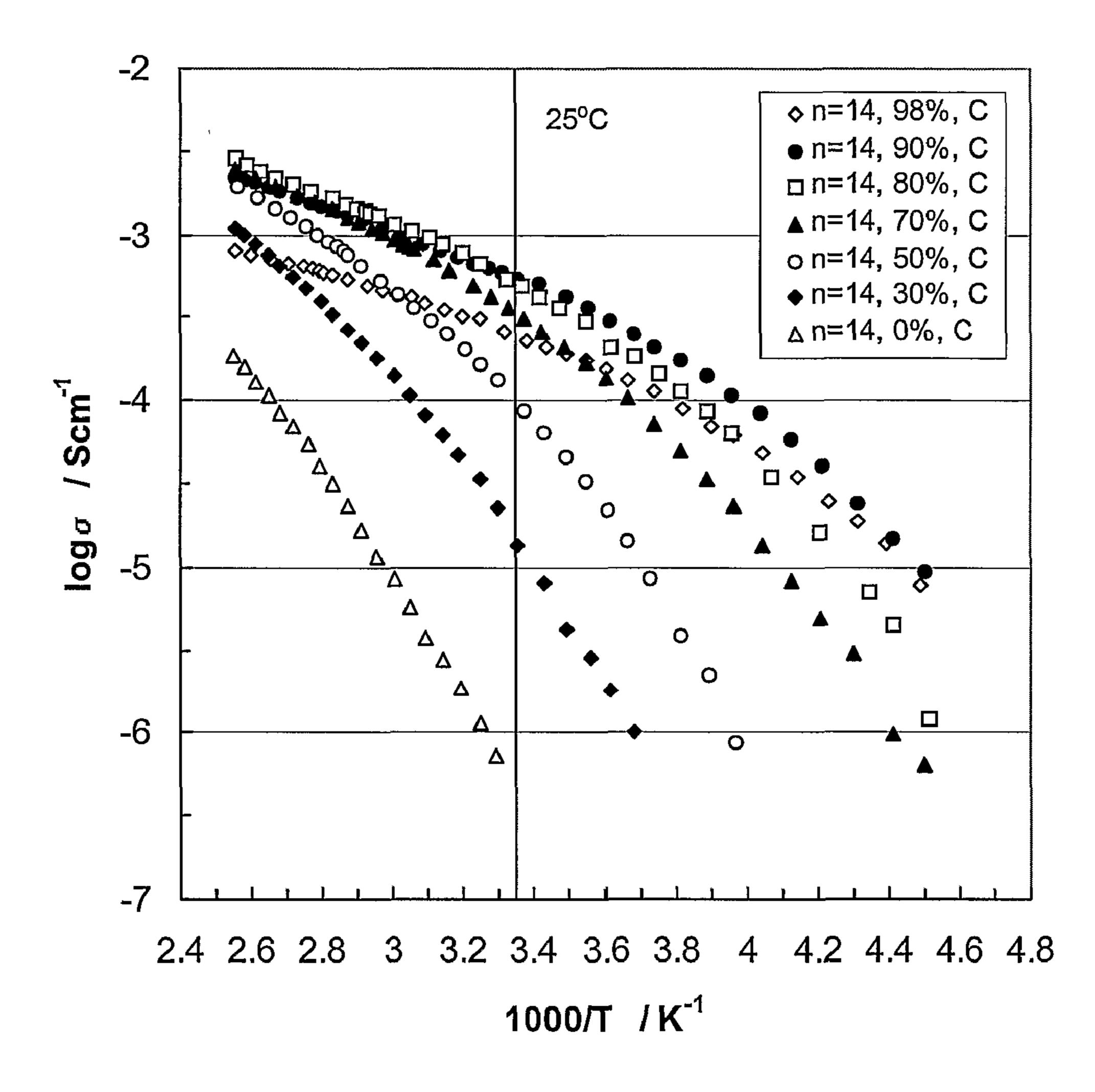
Figure 8C. Temperature dependence of ionic conductivity of EC-PC (1:1 by wt) plasticized LiBH<sub>4</sub>-crosslinked P(LiOEG<sub>14</sub>B) with different content of plasticizer.
