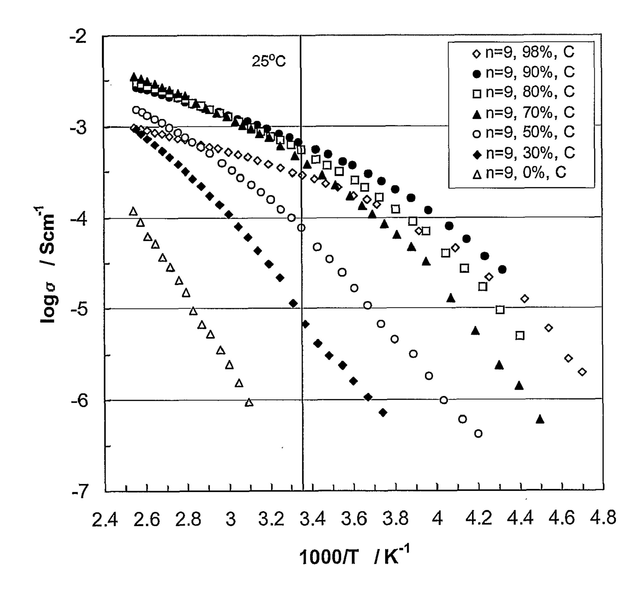
Figure 8B. Temperature dependence of ionic conductivity of EC-PC (1:1 by wt) plasticized LiBH<sub>4</sub>-crosslinked P(LiOEG<sub>9</sub>B) with different content of plasticizer.
