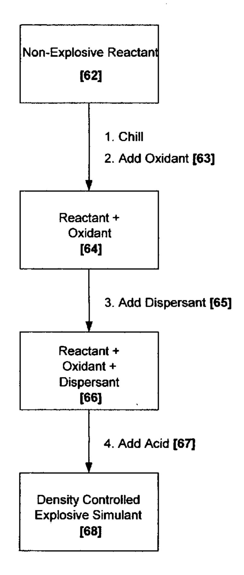
A schematic for the method for making a scent simulant that mimics the odors of live chemical explosives.
