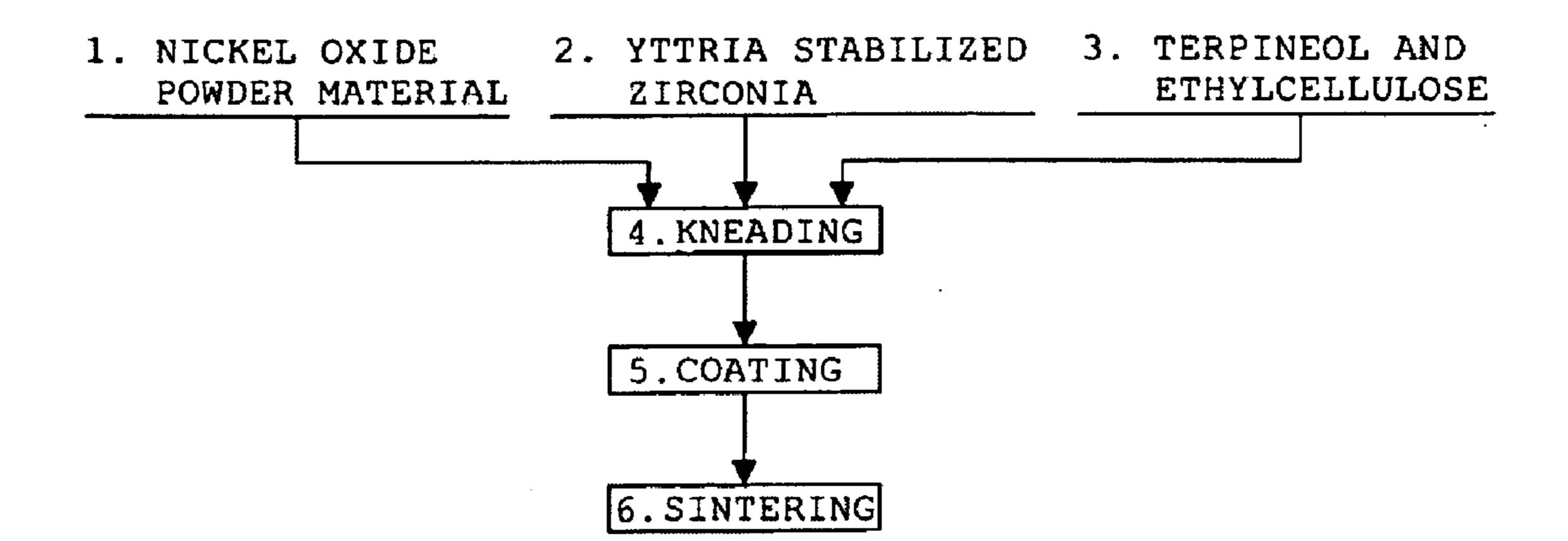
NICKEL OXIDE POWDER MATERIAL FOR SOLID OXIDE FUEL CELL, PRODUCTION PROCESS THEREOF, RAW MATERIAL COMPOSITION FOR USE IN THE SAME, AND ANODE MATERIAL USING THE NICKEL OXIDE POWDER MATERIAL
