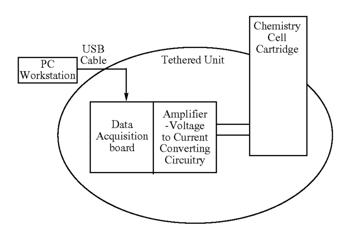
[0338] There a variety of functional requirements or tasks the workstation of this invention must satisfy. These include Control of the Amplifier circuitry
