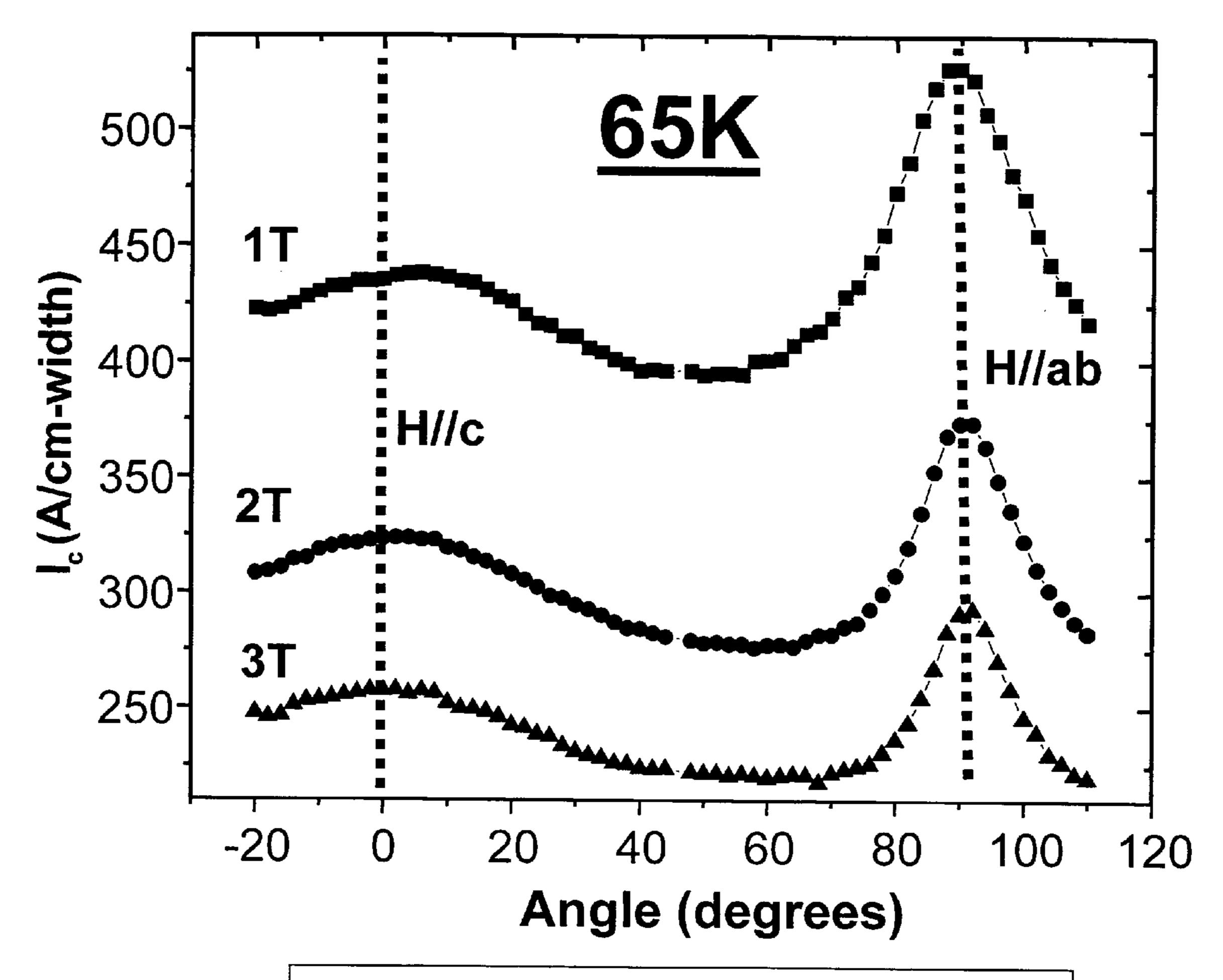
At 65K, 3T, for all field orientations  $J_e = 40,740 \text{ A/cm}^2$  (no stabilizer)  $J_e = 21, 154 \text{ A/cm}^2$  (50 µm stabilizer)
