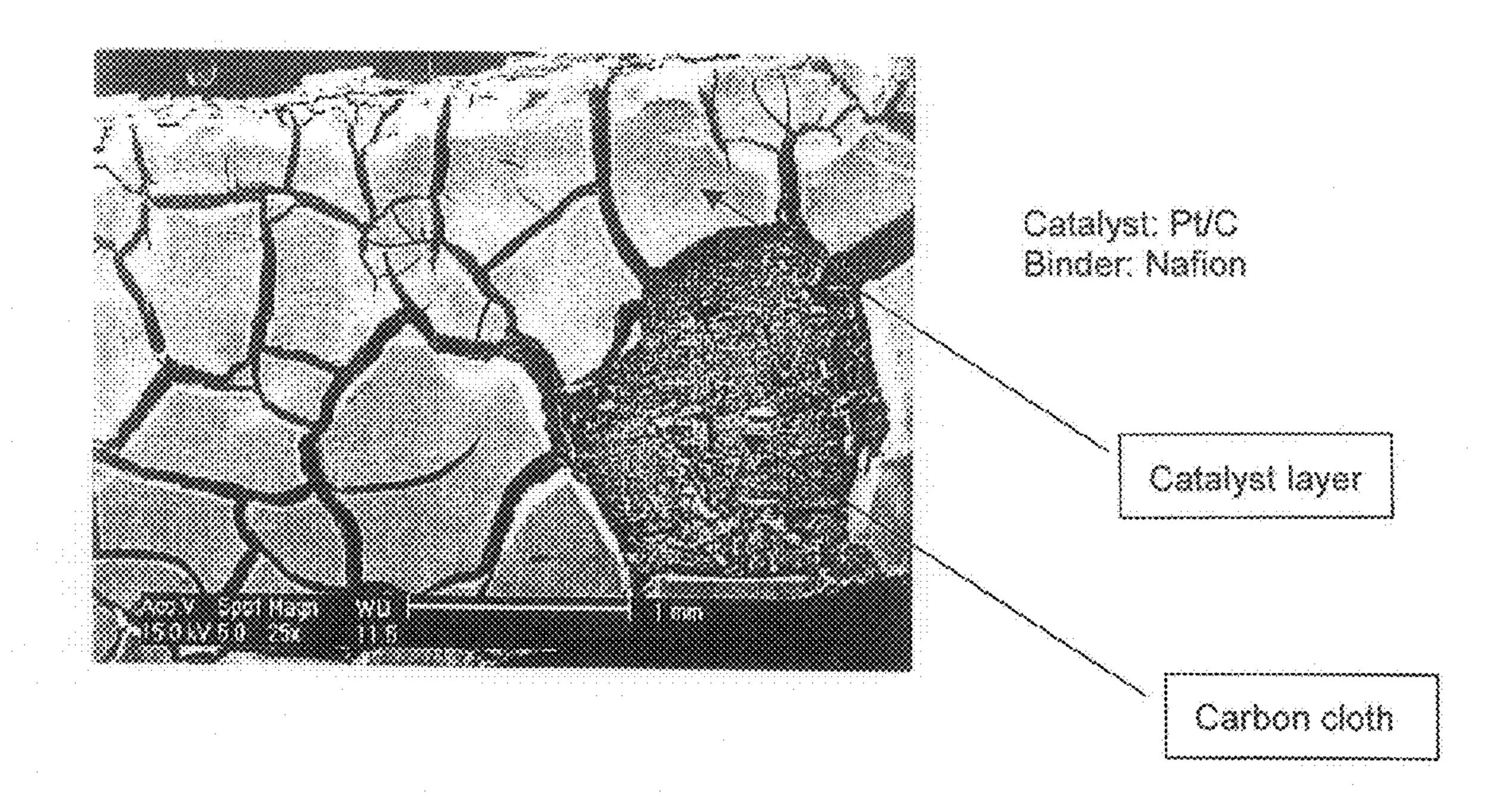
FUEL CELL ELECTRODE, METHOD FOR PRODUCING FUEL CELL ELECTRODE, MEMBRANE-ELECTRODE ASSEMBLY, METHOD FOR PRODUCING MEMBRANE-ELECTRODE ASSEMBLY, AND SOLID POLYMER FUEL CELL
