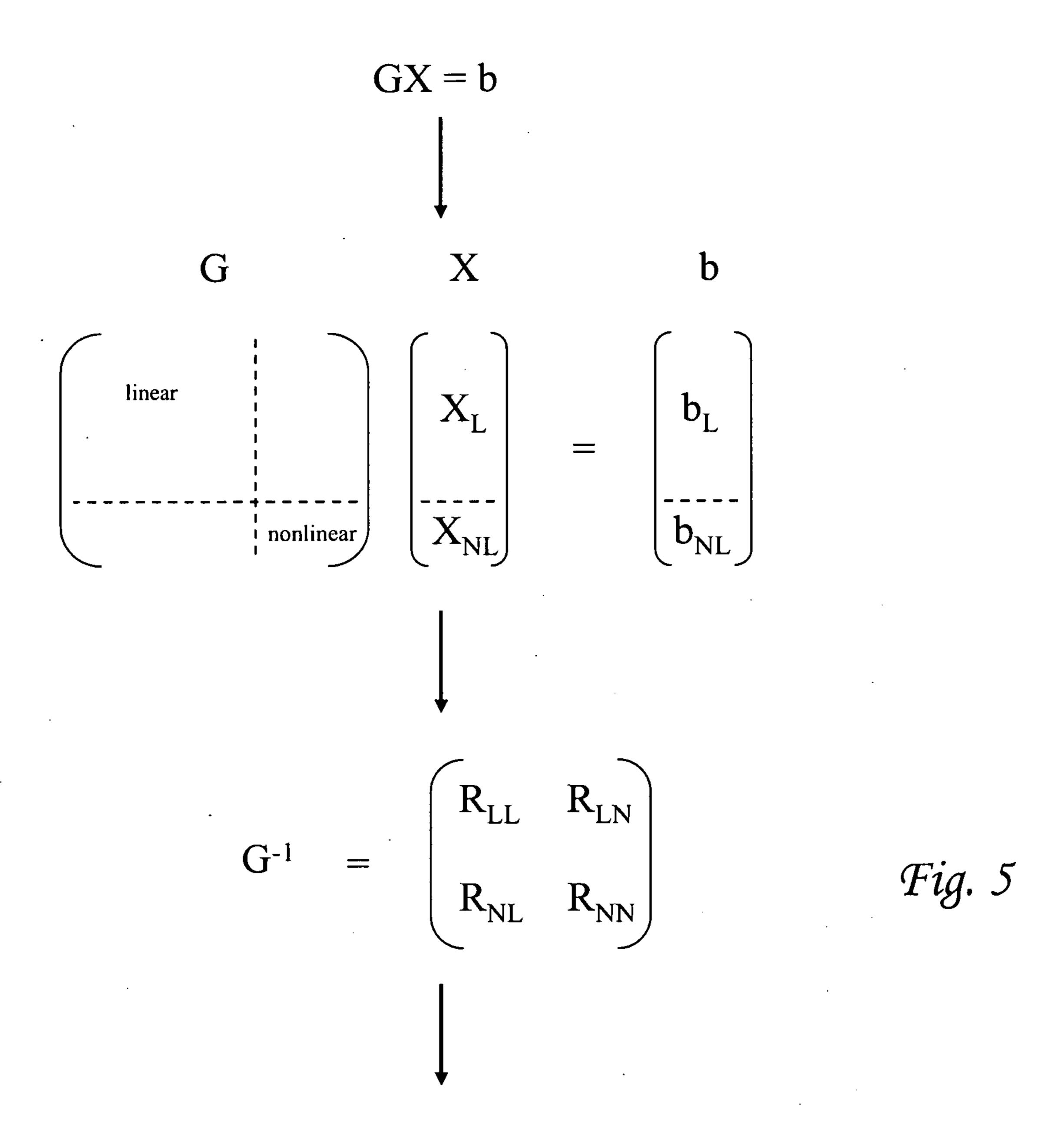
$$\begin{split} X_L^{k+1} &= [R_{LL}R_{LN}]I_L + R_{LN}(I_{NL}(X_{NL}^k) + J_{NL}^k(X_{NL}^{k+1} - X_{NL}^k)) \\ X_{NL}^{k+1} &= [R_{NL}R_{NN}]I_L + R_{NN}(I_{NL}(X_{NL}^k) + J_{NL}^k(X_{NL}^{k+1} - X_{NL}^k)) \end{split}$$
