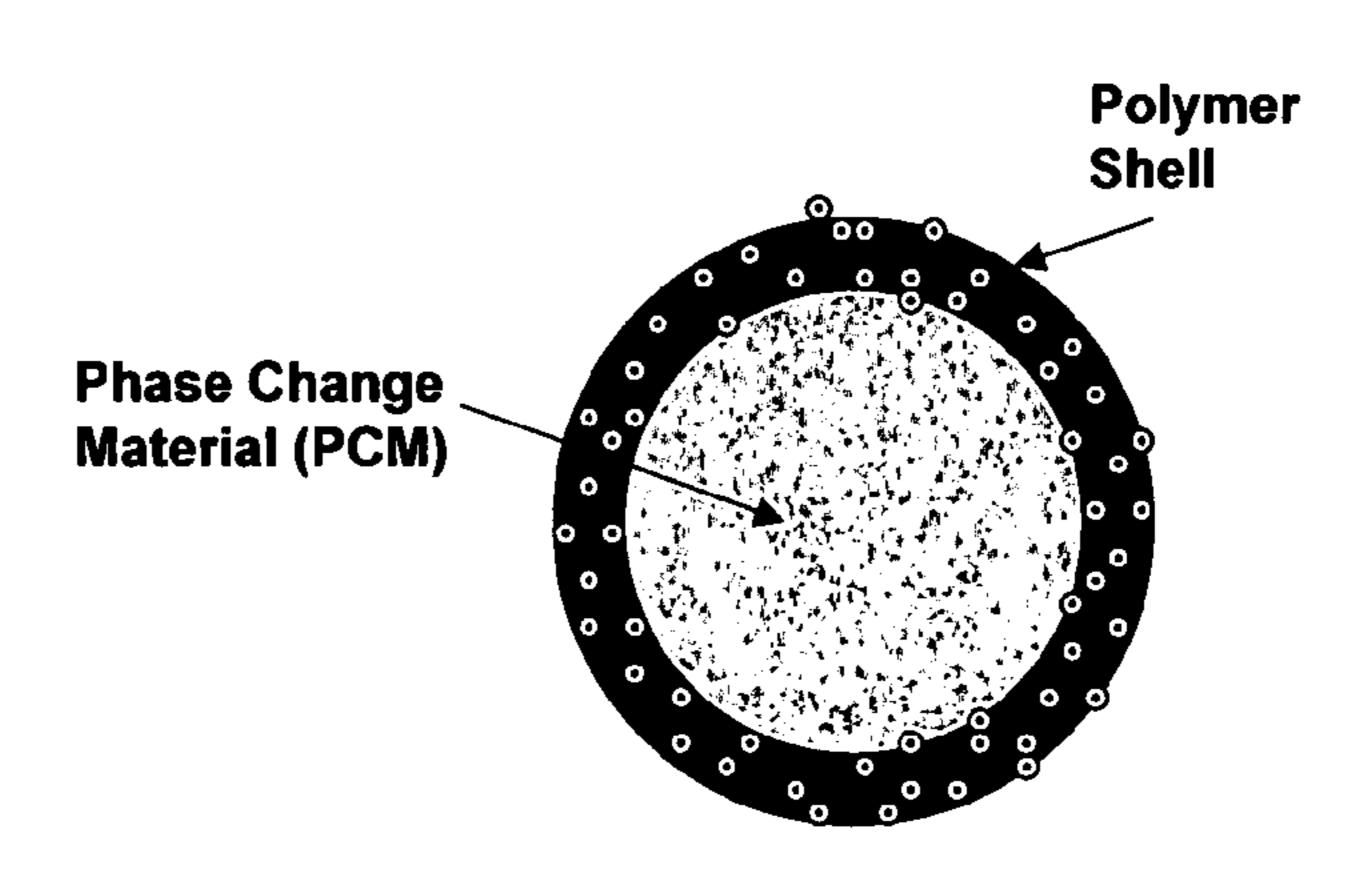
Figure 3. Structure of a PCM and polymer shell (embedded with nanoparticles) hybrid nanoparticle. The gray circles in the polymer shell layer are nanoparticles.
