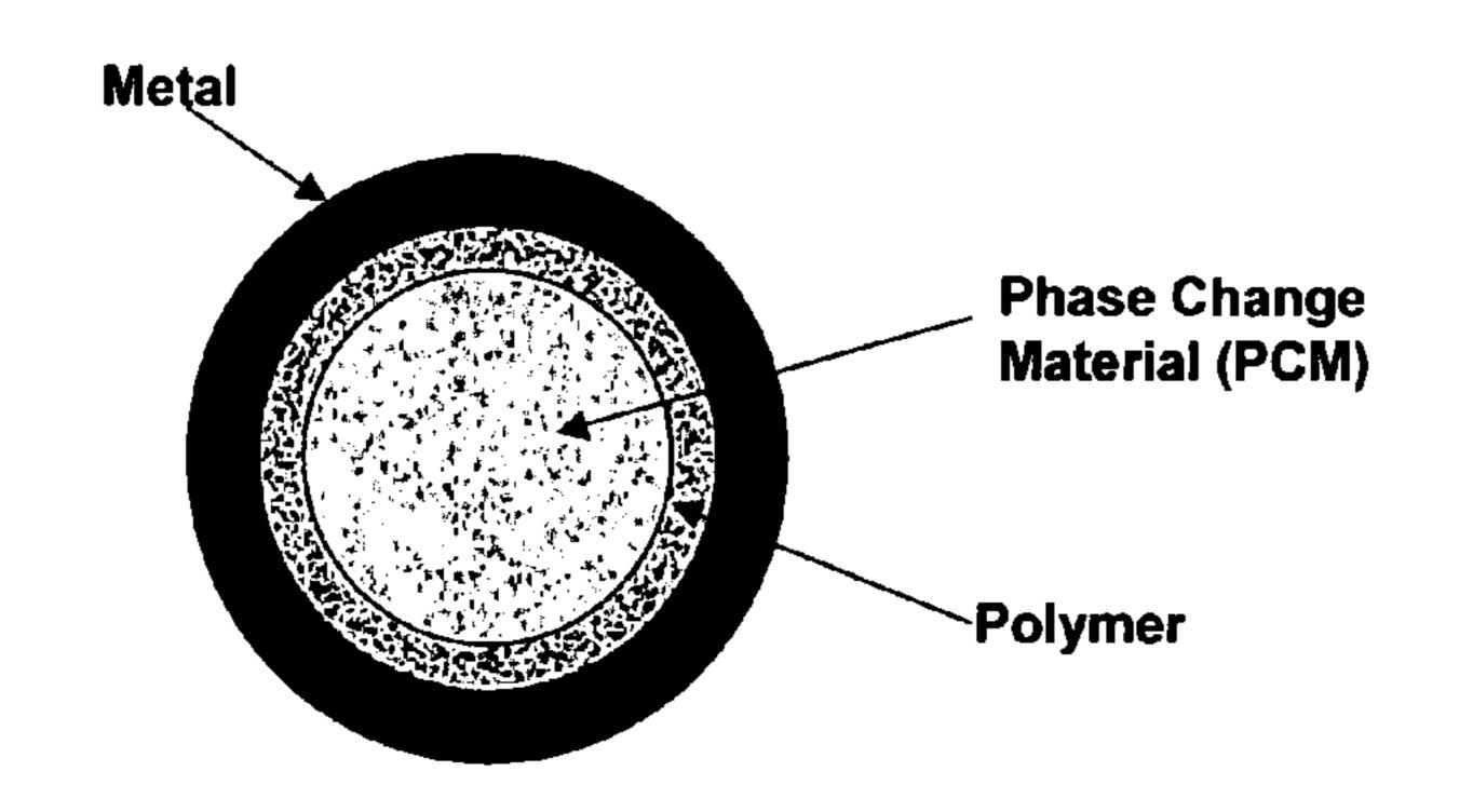
Figure 2. Structure of a PCM, polymer layer, and metal shell hybrid nanoparticle
