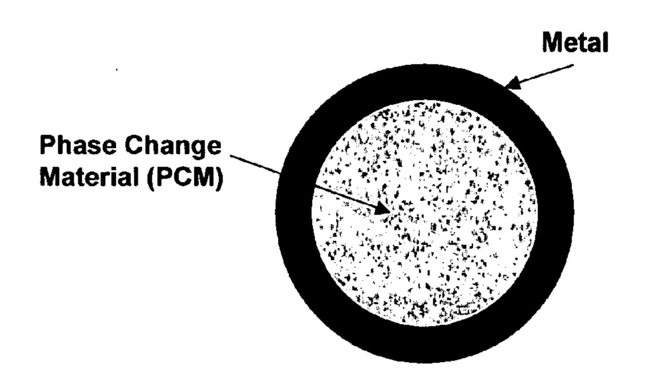
Figure 1. Structure of a PCM and metal shell hybrid nanoparticle
