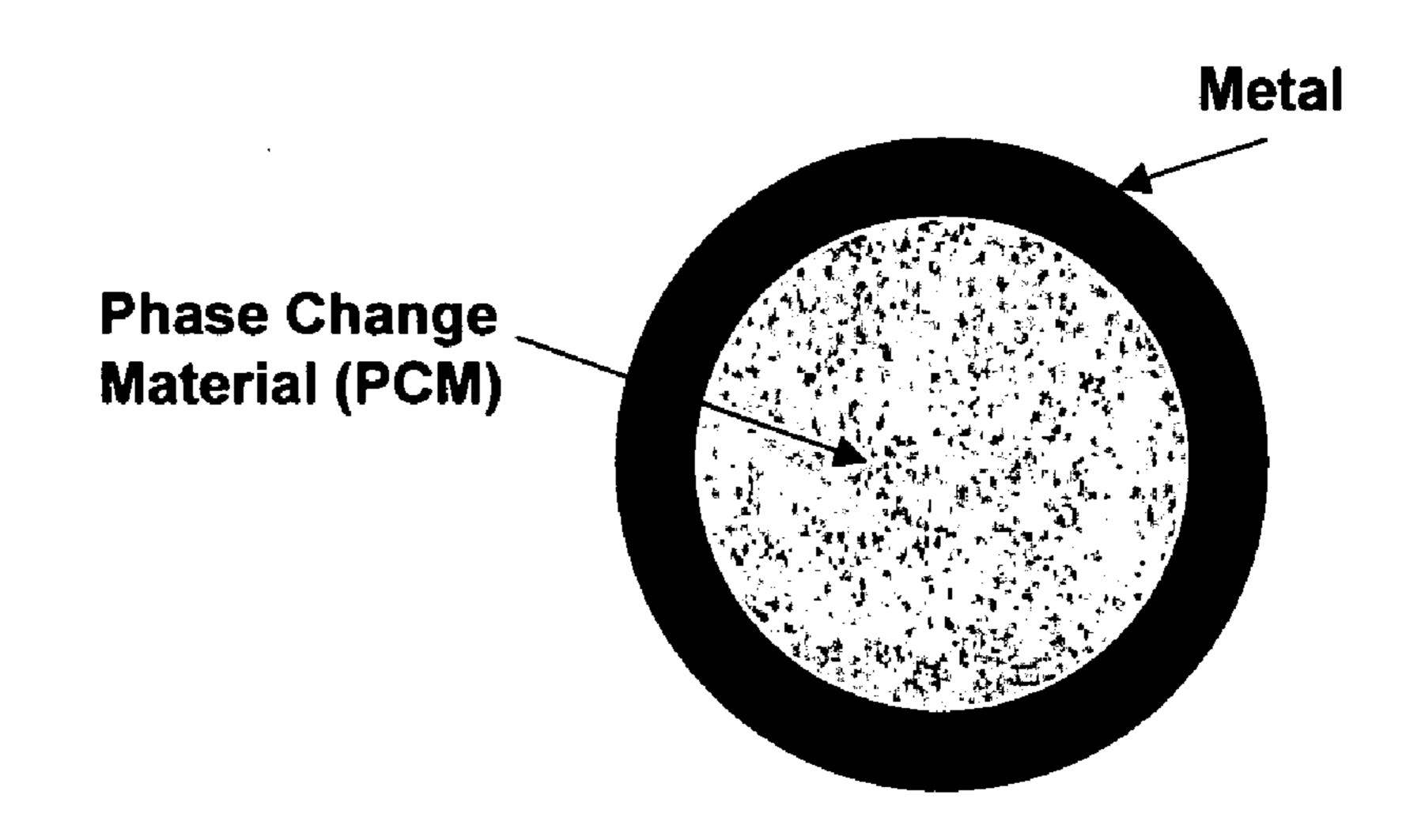
Structure of a PCM and metal shell hybrid nanoparticle
