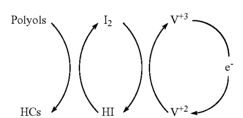
[0019] In the present invention, there is no waste byproduct produced, such as phosphoric acid. The HI/V<sup>2+</sup>V<sup>3+</sup> system
