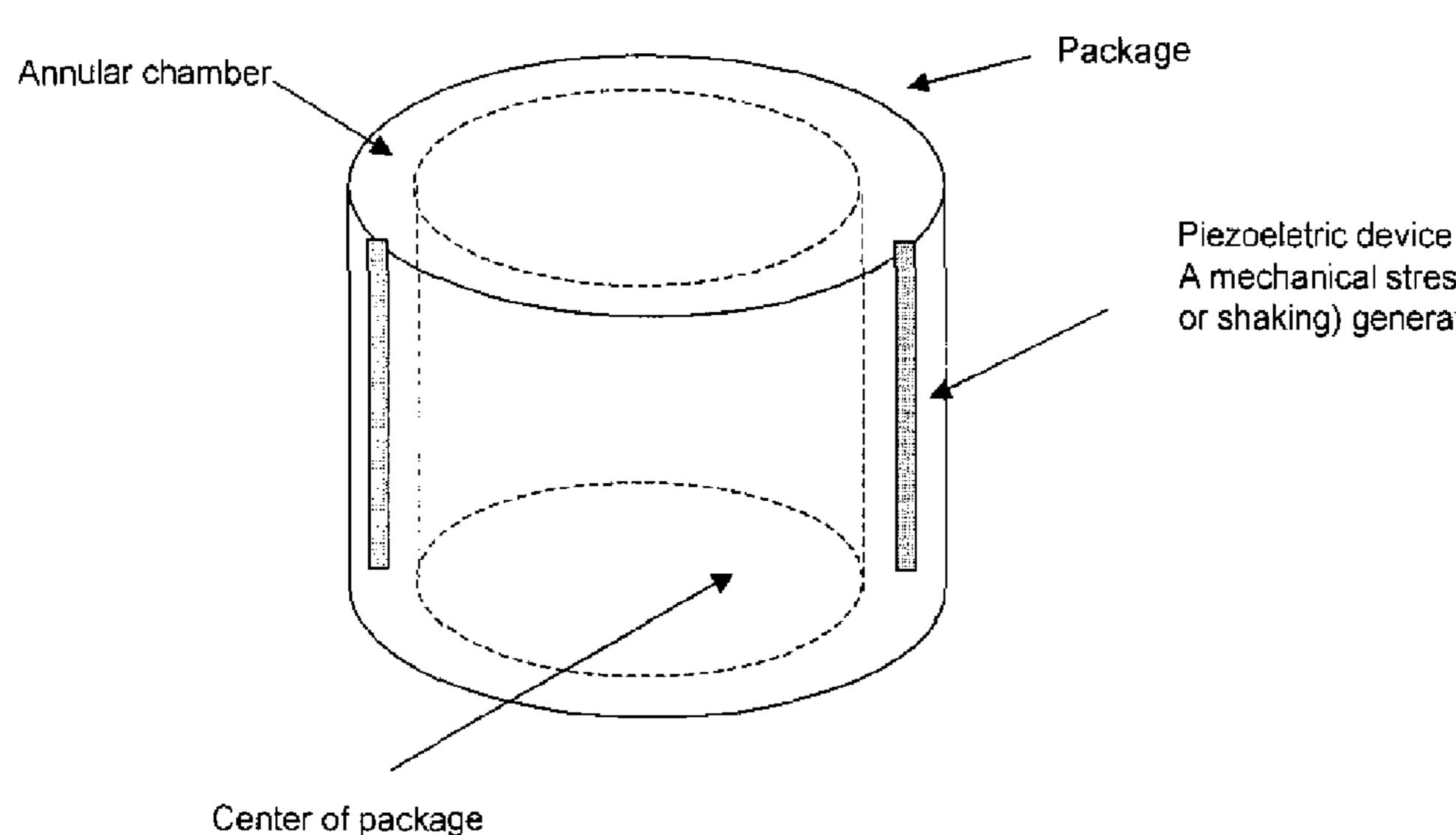
Piezoeletric device in annular chamber. A mechanical stress (e.g. via squeezing or shaking) generates a voltage.
