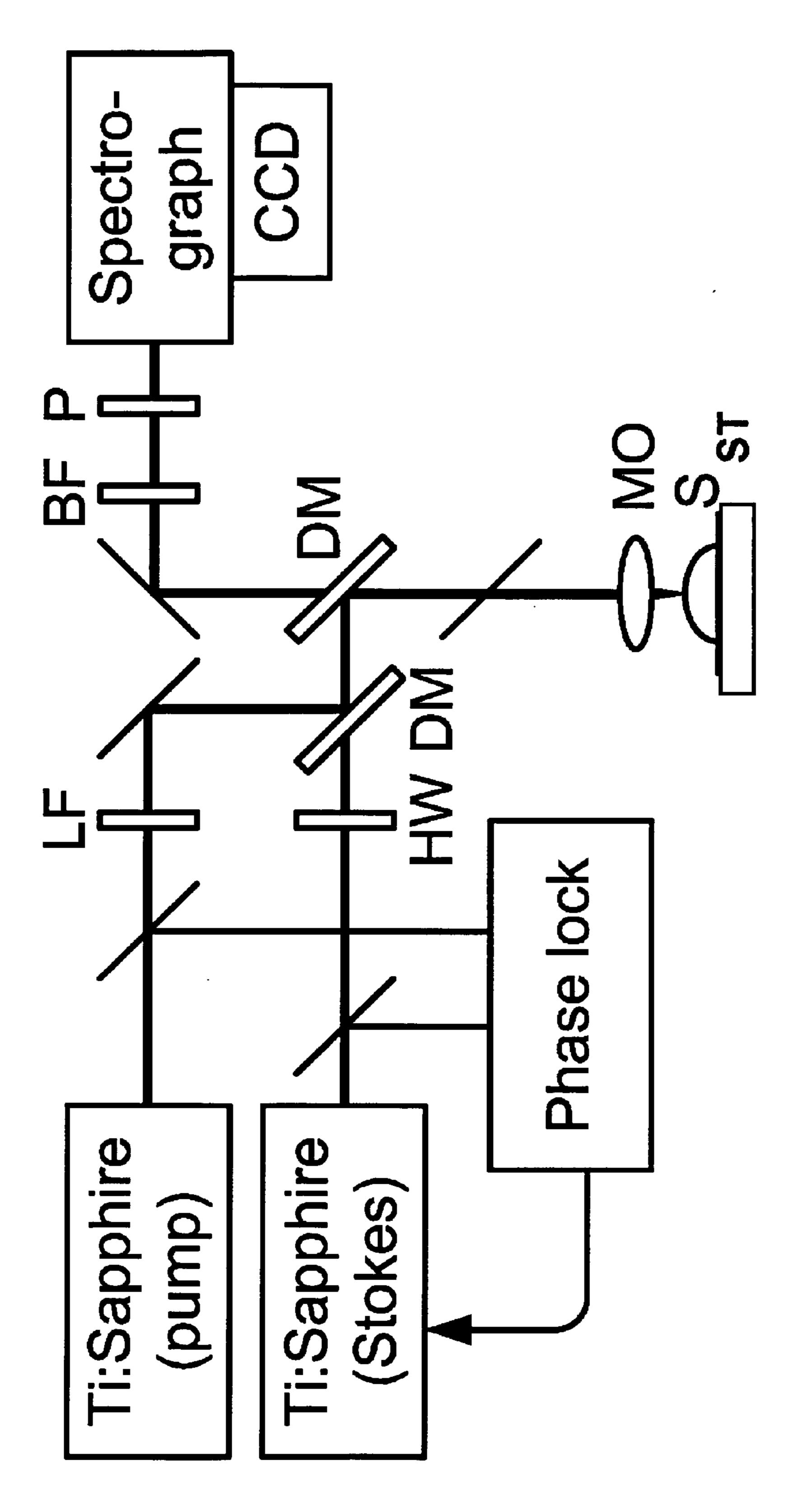
LF, laser line filter; HW, half-waveplate; DM, dichroic mirror; BF, ST, sample stage; CCD, charge coupled device camera
