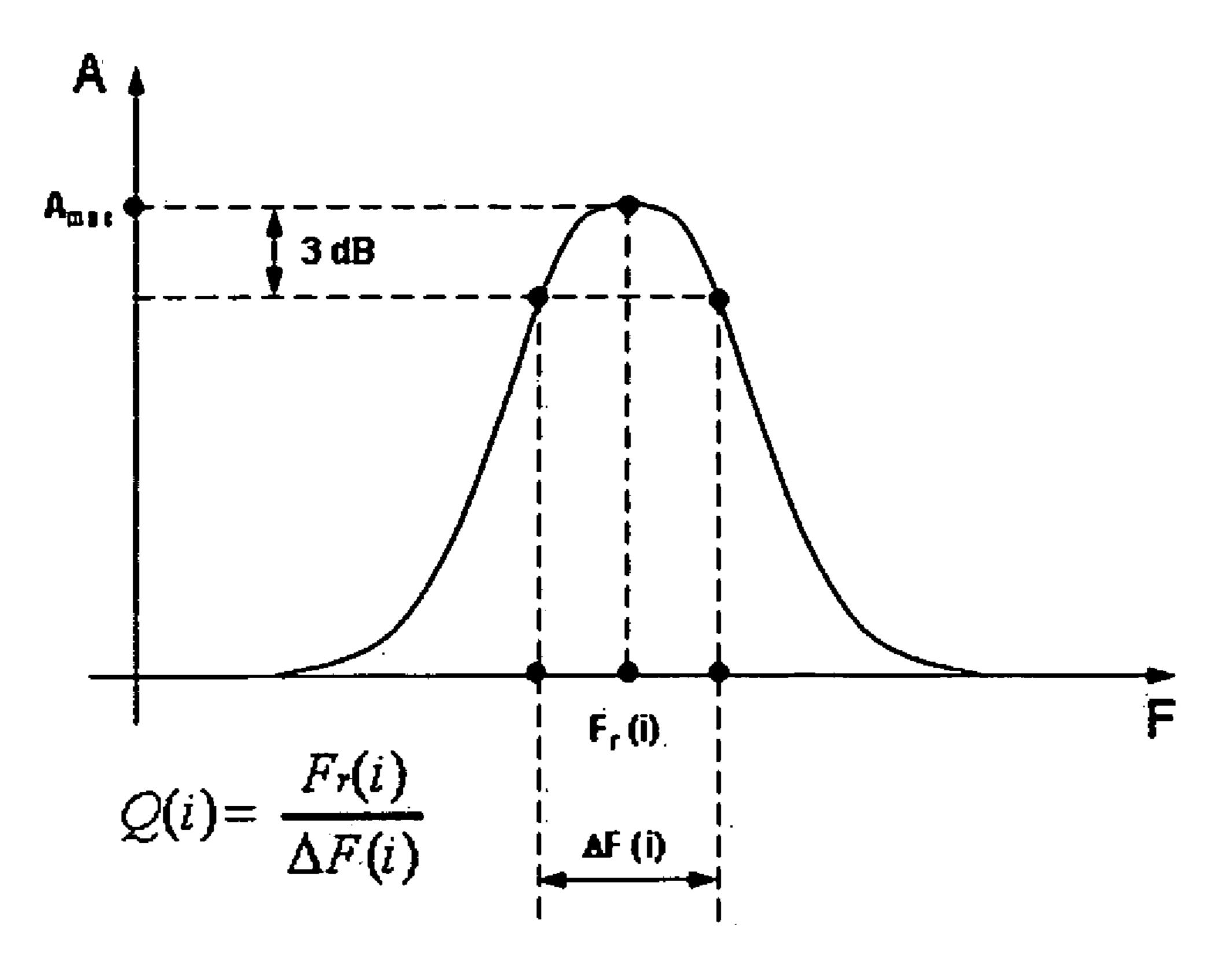
A<sub>max</sub> – maximum signal from LCR resonant circuit
