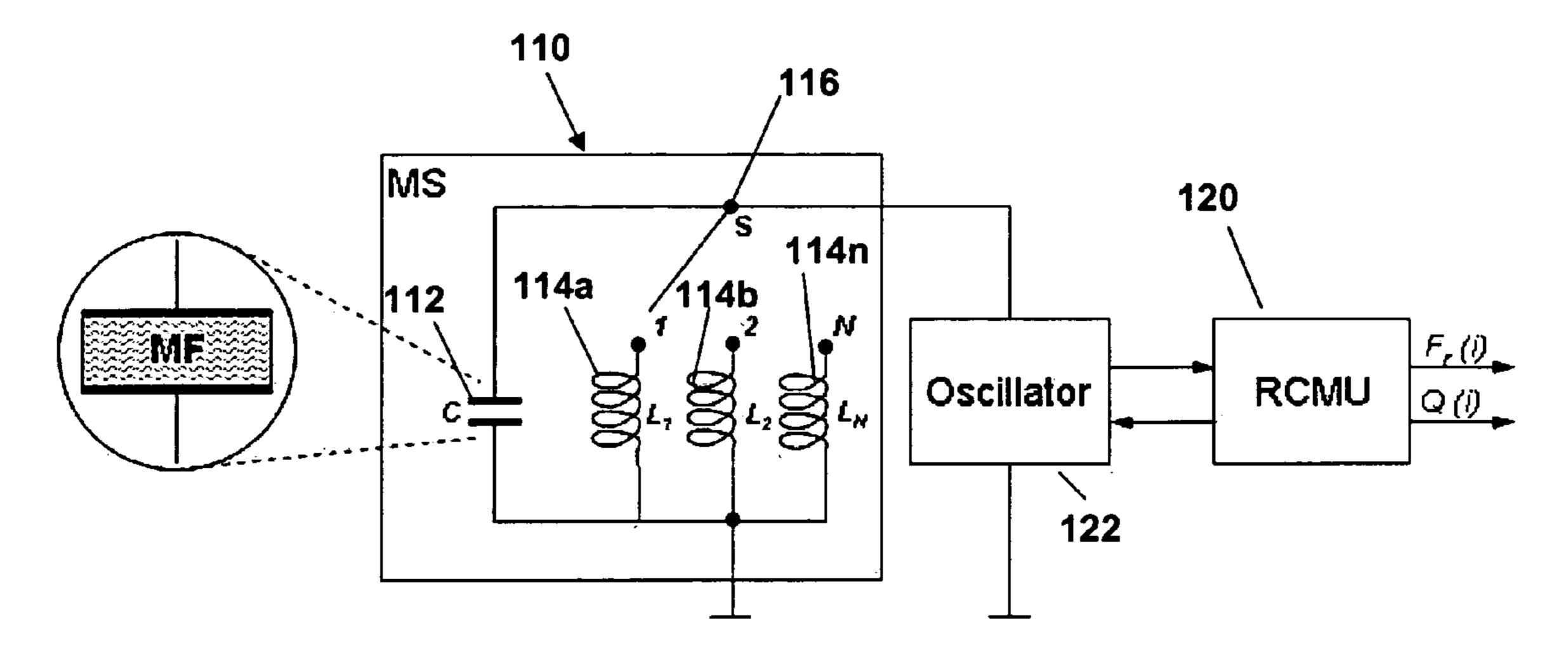
MS - measuring sensor (LCR Measuring Circuit)
