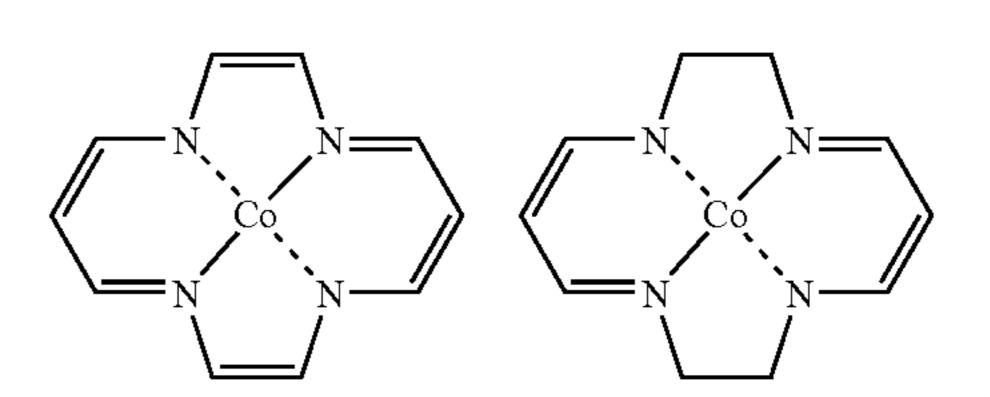
[0235] On the other hand, the center metal atom of a metal complex shifts to a high oxidized state at the time of oxygen reduction. In order to restore the catalyst ability at the next reaction cycle, the center metal atom must be reduced to the low oxidized state. This reduction reaction proceeds more easily the stronger the electron attraction of the complex ligand.
