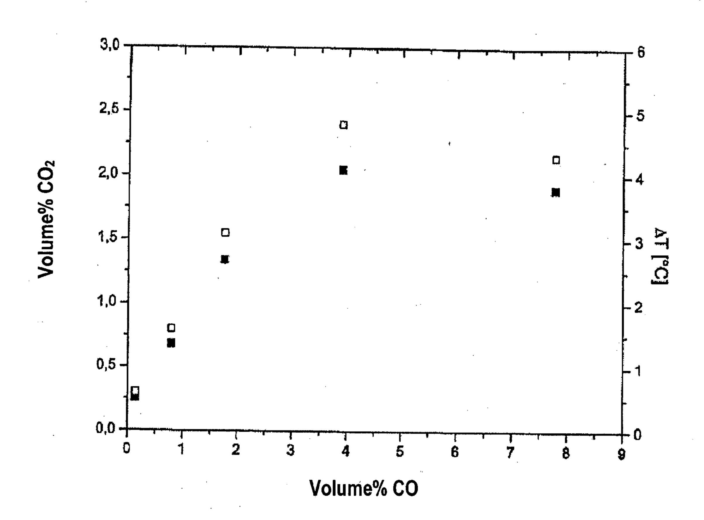
CO<sub>2</sub> yields (filled squares) and temperature differences (empty squares) at different CO concentrations at -20 °C
