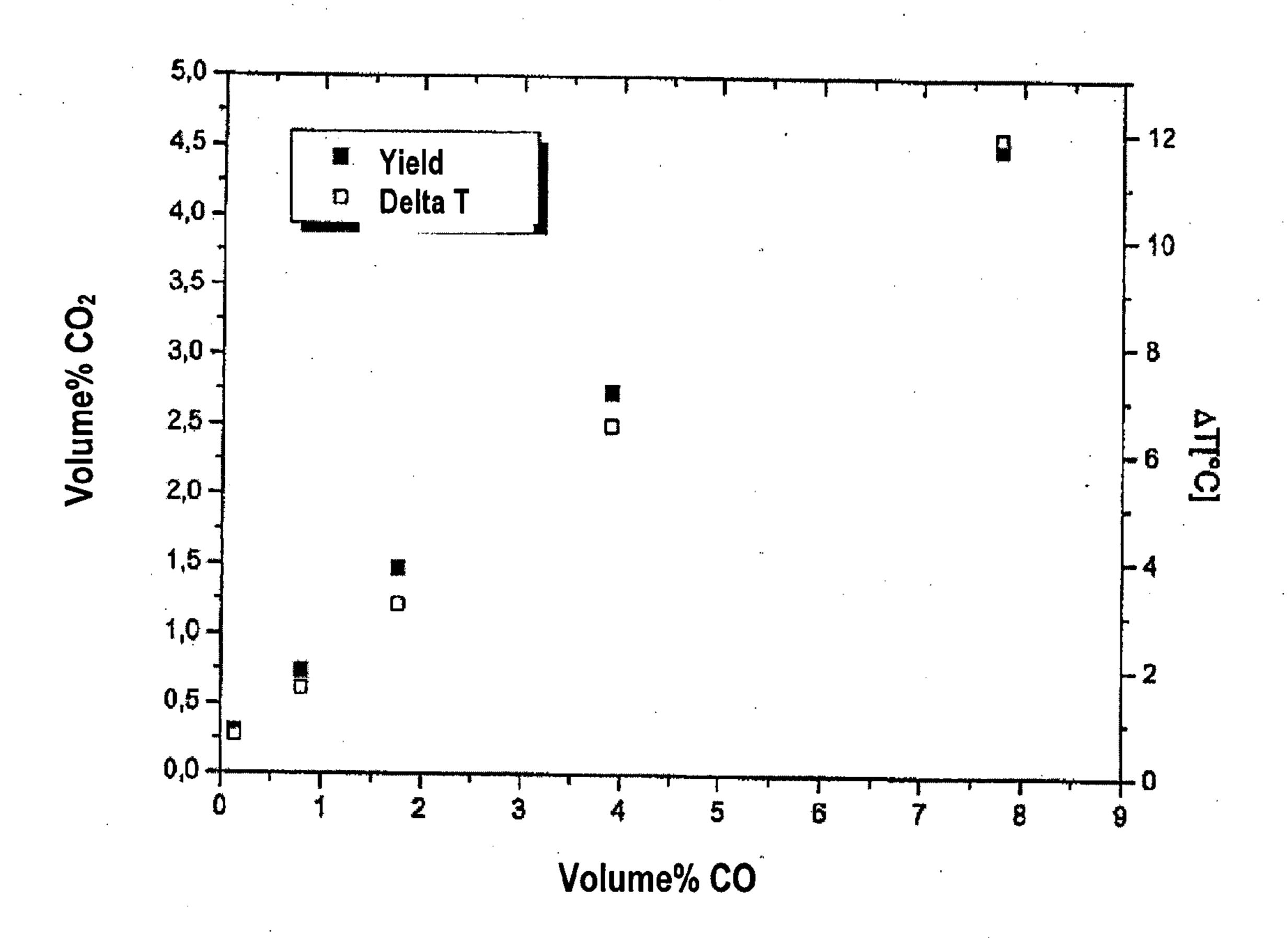
CO<sub>2</sub> yields and temperature differences at different CO concentrations at 0 °C
