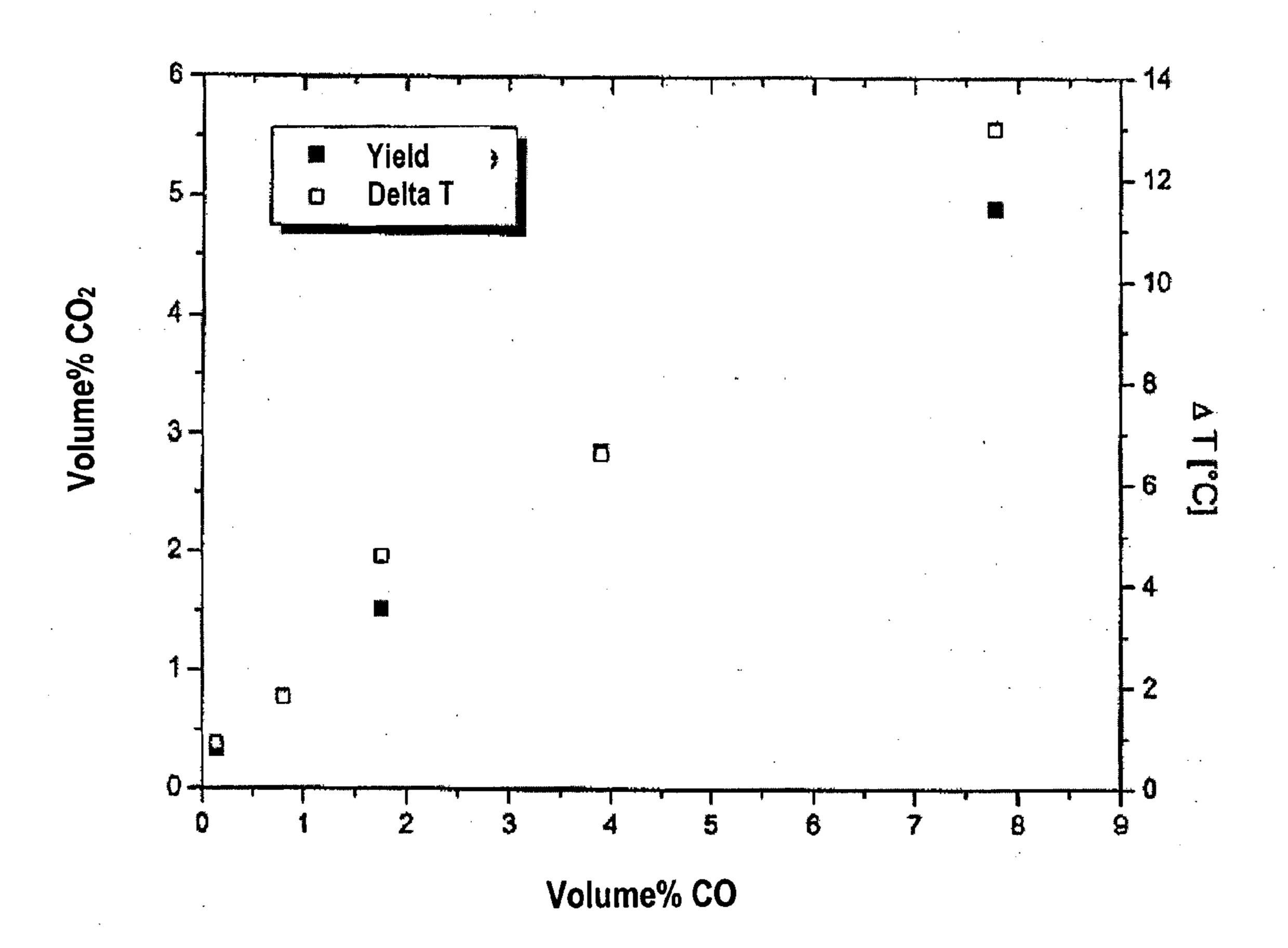
CO<sub>2</sub> yields and temperature differences at different CO concentrations at + 50 °C and a flow rate of 12.8 mL/min
