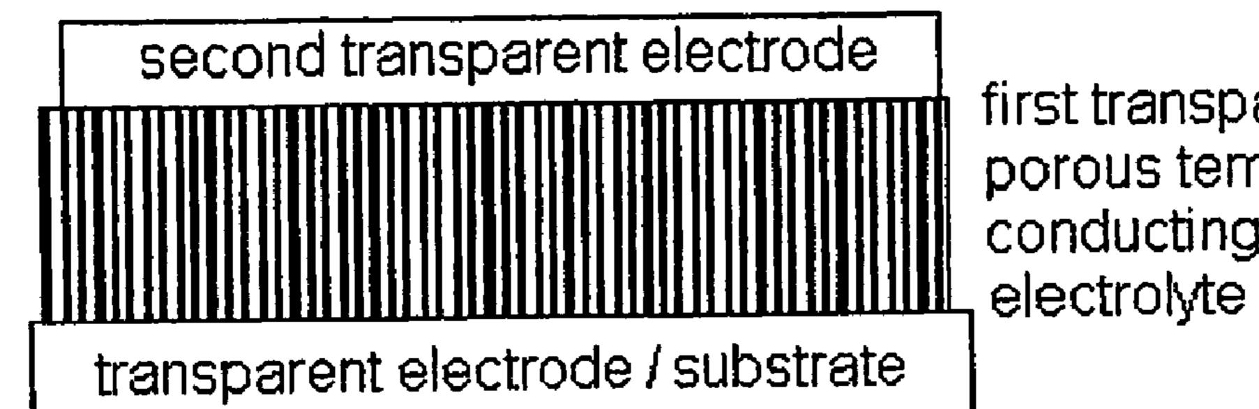
first transparent electrode/ porous template/ conducting polymer/ electrolyte
