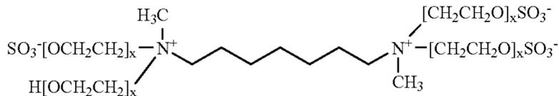
wherein x is from about 20 to about 30 and approximately 40% of the (poly)alkoxyene chain terminal alkoxy moieties are sulfonated.
