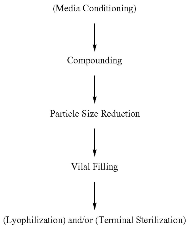
[0172] As indicated by the optional steps in parentheses, some of the processing is dependent upon the method of particle size reduction and/or method of sterilization. For example, media conditioning is not required for a milling method that does not use media. If terminal sterilization is not feasible due to chemical and/or physical instability, aseptic processing can be used.
