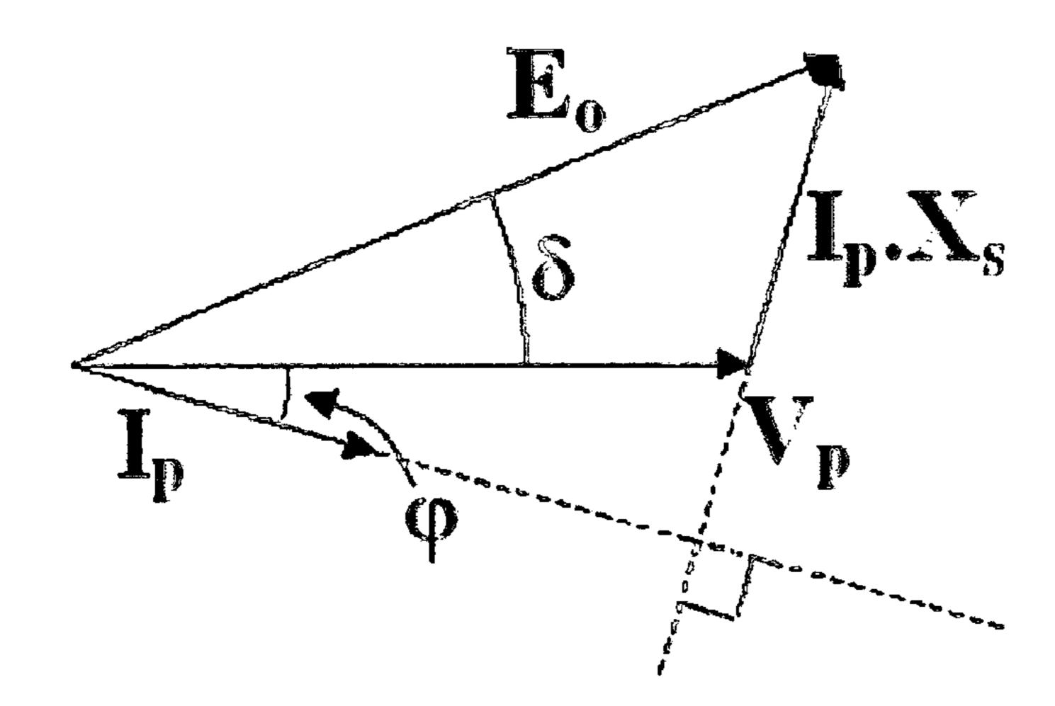
(b)  $E_o$  leads  $V_p$   $|E_o| > |V_p|$  means that  $I_p$  lags  $V_p$
