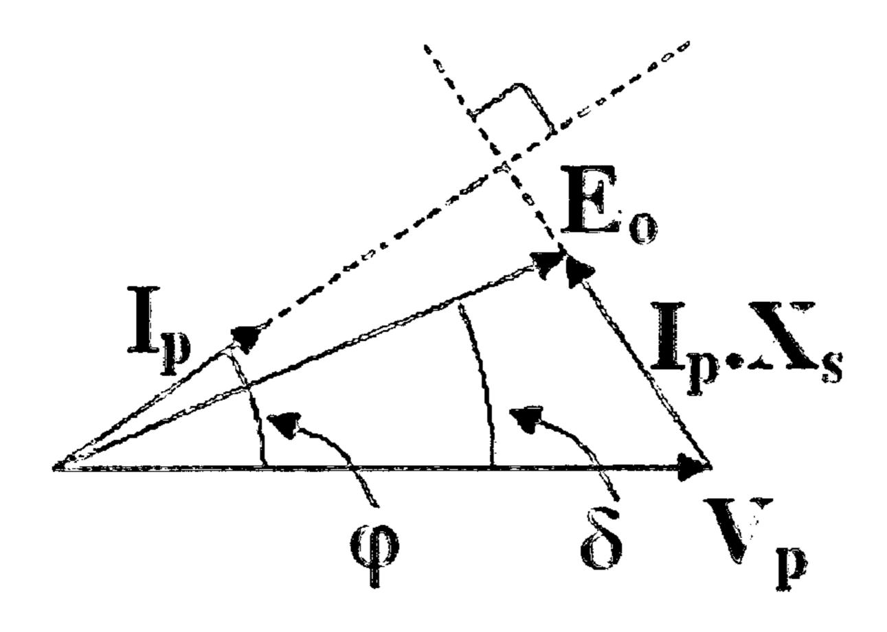
(a)  $E_o$  leads  $V_p$   $|E_o| < |V_p|$ means that  $I_p \text{ leads } V_p$
