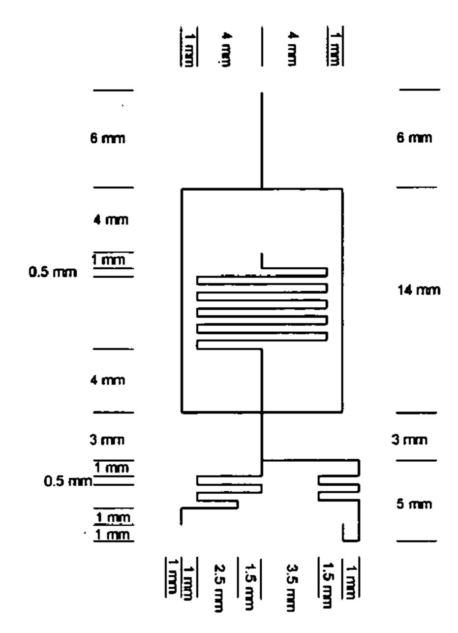
Drawing is on a 0.5 mm grid. All lines are 10 µm wide.
